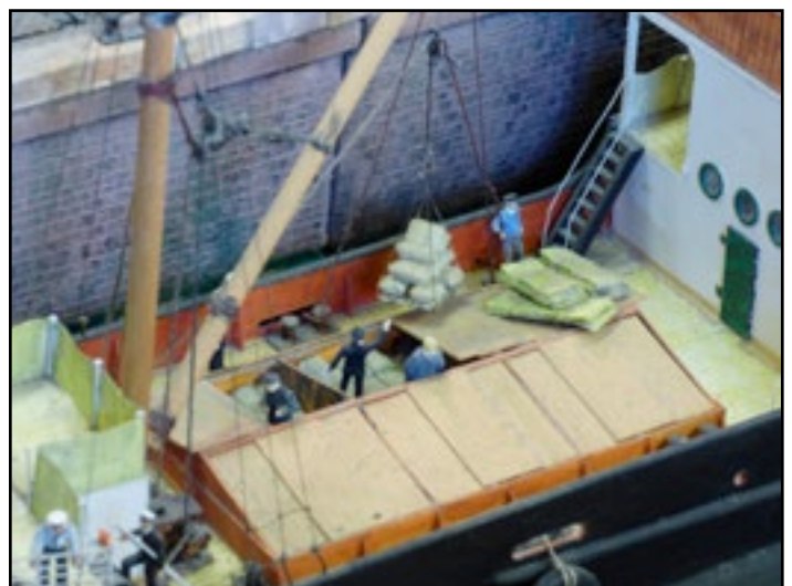
The cargo of potatoes is being unloaded from the fore-hatch using the ship's own derricks. Note the folded paper tarpaulins and the other fittings
