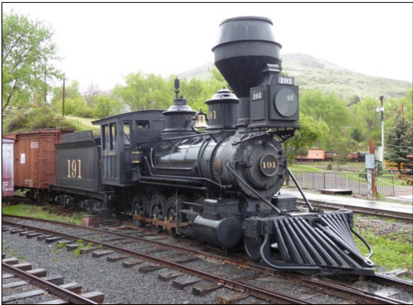
DL&G #191 a diamond stacked narrow gauge 2-8-0 at Colorado Railroad Museum, Golden CO (Mike Ford)
