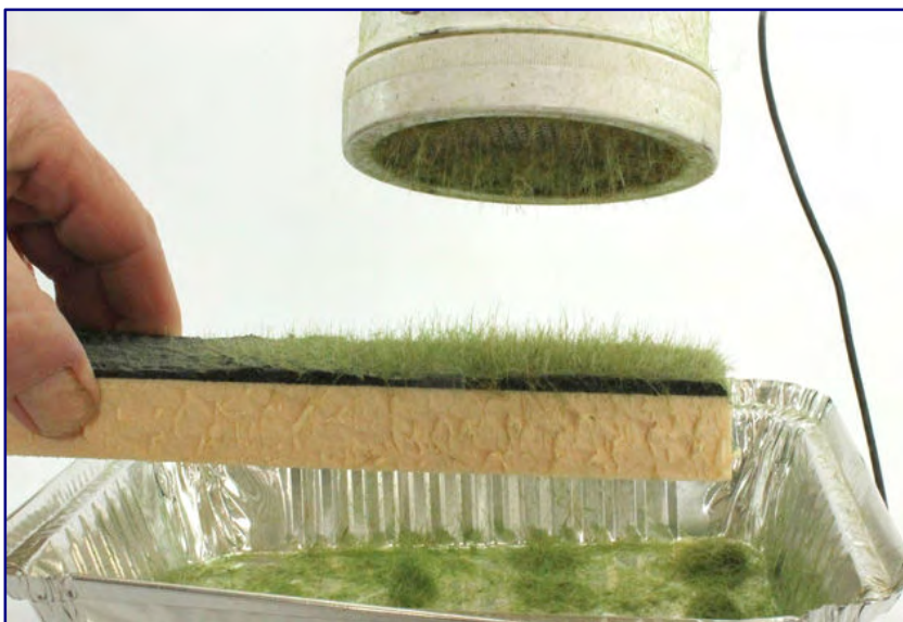
The difference to other electrostatic techniques is the ionising resin, which is seen here as a black layer on the test strip. It is now also possible to produce trees, which can be made in the same way. Photo: Microrama Model Decor
