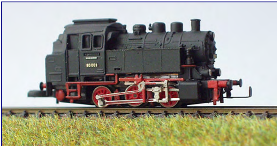
On Märklin's series 89, the fine detailing of Michael Bahls is based on detail control, brake remodelling, third dome and water boxes (art.-No. 5080). Photo: Bahls Modelleisenbahnen
