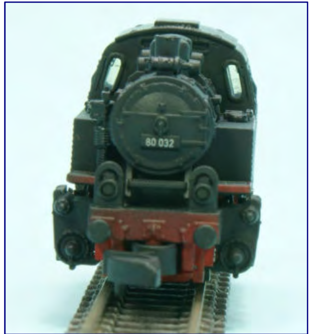
In the view from the front it is noticeable that the steam cylinder did not determine the largest width of the locomotive. That was the role of the cab, which appears to have been decreased in size.
