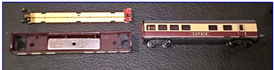
The individual modules are ready after dismantling both carriages (Fig. 2 above). The different coupling solutions of the two generations of TEE trainsets (Fig. 3 left) require a great deal of internal conversion work, as the old car body and the new electrical connection (Fig. 4 right) have to be brought together here. Photos: Torsten Scheithauer
