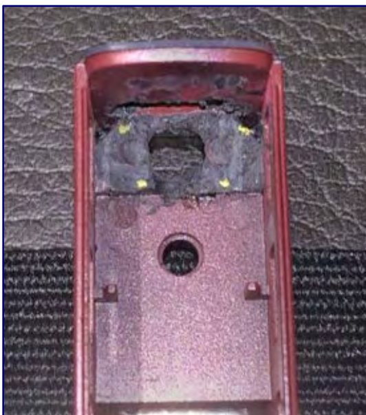
Left picture: Yellow colour marks the points for the four holes so that the coupler receptacles are secured in the floor. Photo: Torsten Scheithauer
