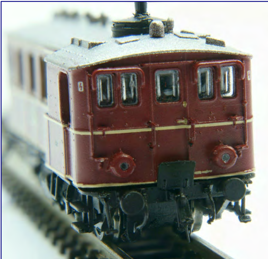
A view of the front reveals the most filigree parts of the steam railcar: steps on the right and left of the buffers, screw coupling and brake hoses. The railings next to the front door have also been recreated free-standing.
