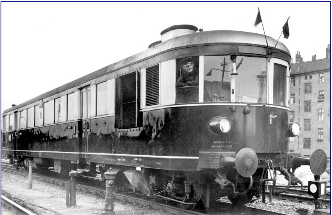
Influenced by the success of fully automatic steam generation systems, eight steam railcars (DT 51 to 58) were built by Borsig, Henschel and Wegmann for the Reichsbahn between 1934 and 1938. Hermann Maey had the new DT 53 driven into position in Berlin Stettiner Bahnhof on 4 May 1936. Photo: DLA Darmstadt (Hermann Maey), Sammlung Eisenbahnstiftung
