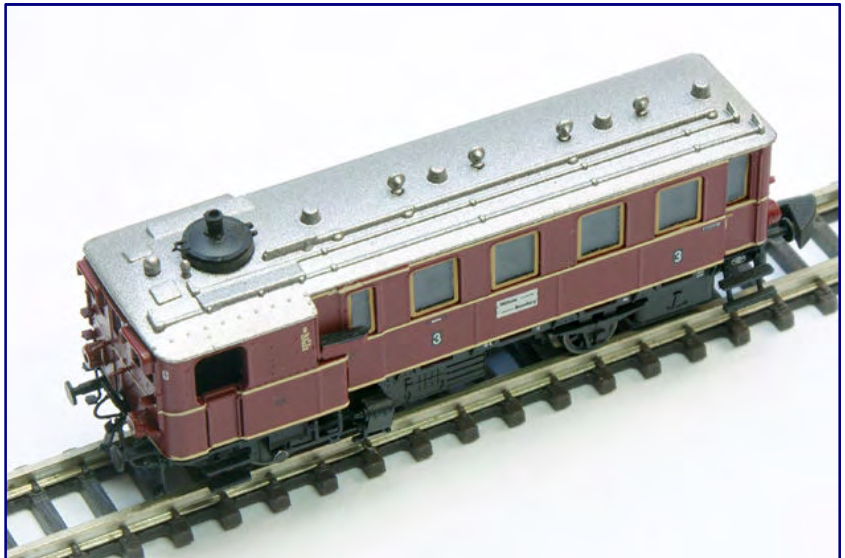
Also the detailing of the roof makes a good impression: We already knew the four torpedo fans above the passenger compartment from FR Freudenreich Feinwerktechnik, but not in this detail. To remove it, simply pull the housing upwards.
