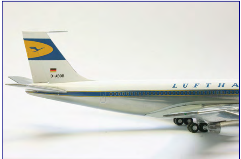
In the condition of 1960 the Boeing 707-400 still has a short rudder. Another striking feature is the Kranich company logo in the yellow parable, which Lufthansa had finally decided on.
