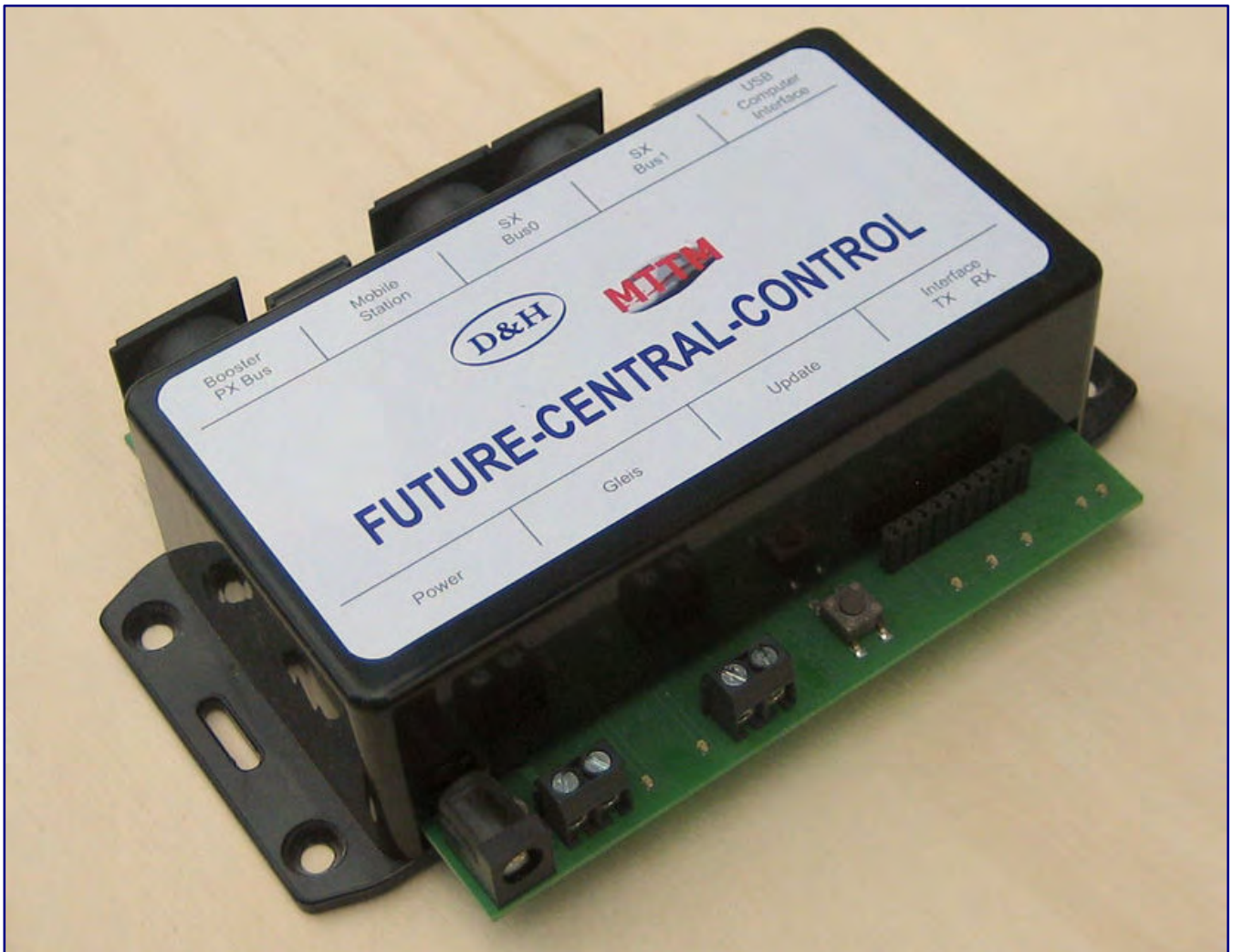
The FCC (Future-Central-Control) from Doehler & Haass is one of the digital control centres to which a handheld controller with display or a computer must be connected separately. Photo: Andreas Hagendorf
