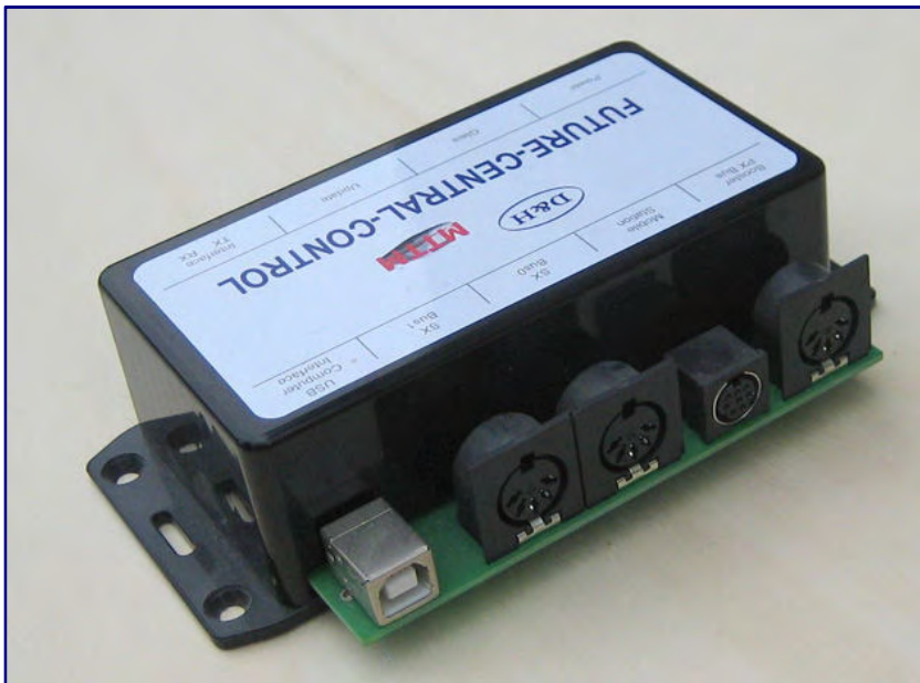
The number of different interfaces, shown here is the FCC of D&H, is an important decision criterion when choosing the digital system. Photo: Andreas Hagendorf
