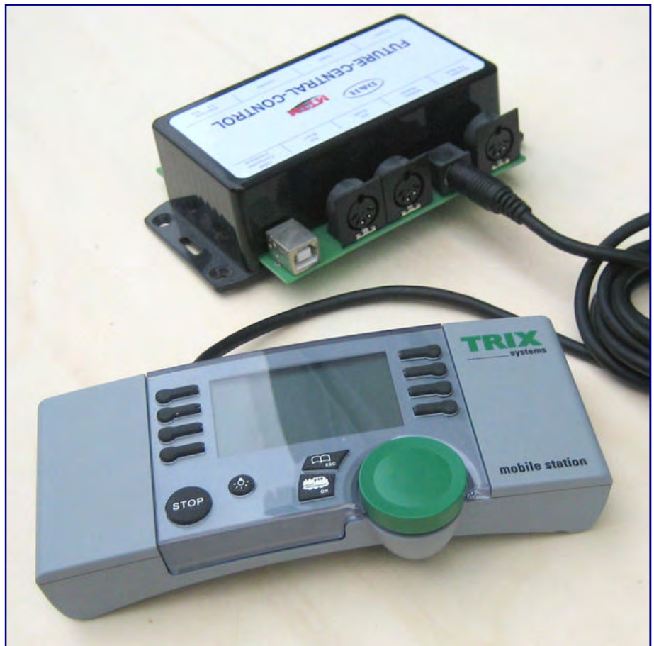
Here a Mobile Station 1 from Trix has been connected to the FCC as a hand controller. On its own, it also works as a small control centre, but only for the power train.
