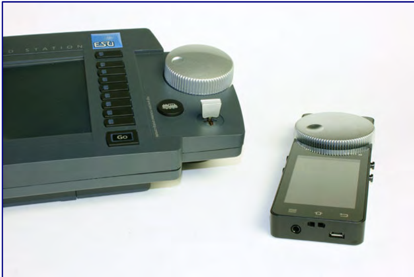
Many of the central units available on the market already have an integrated amplifier (booster).
