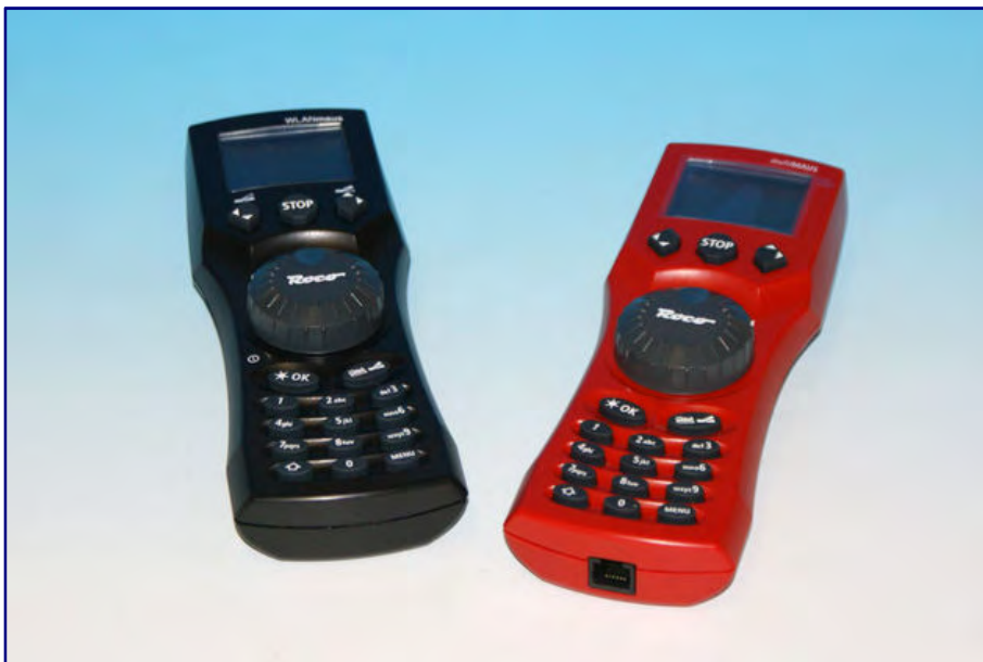
The multi-handset control from Roco (right), which is also used in Z gauge, is both a handset control and a small central unit. It can also switch points or mechanical signals. Its modern successor is the WLAN mouse (left) from the same manufacturer.
