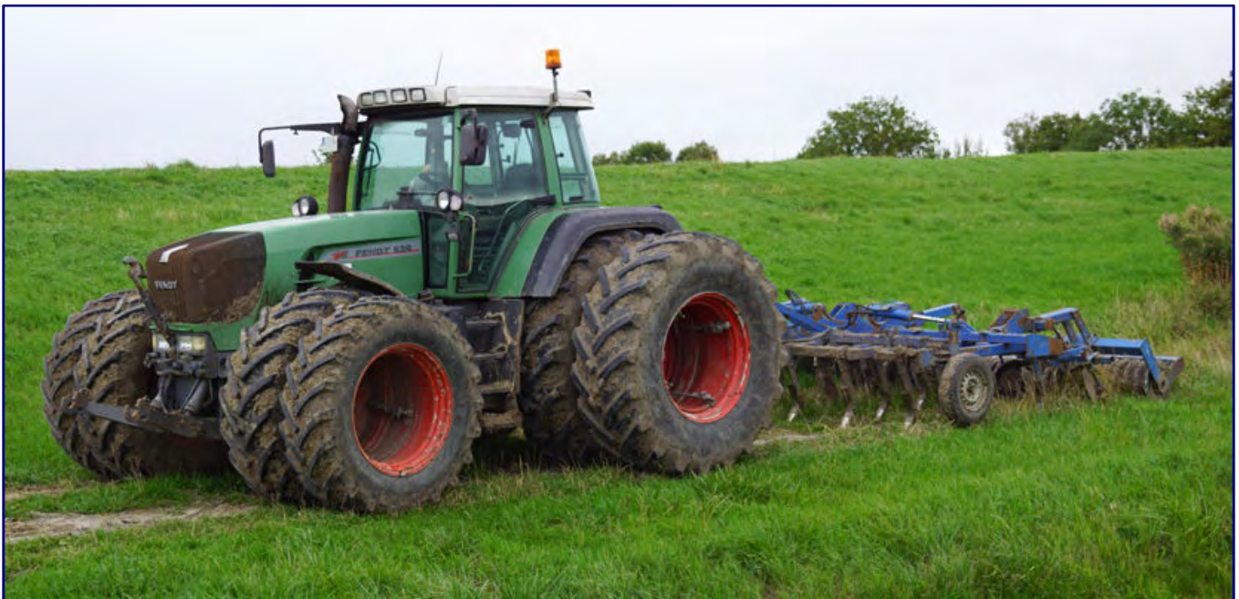
Over the last seventy years, tractors have become larger and more powerful to meet the ever-increasing demands of the equipment that they pull. This Fendt 926 Vario TMS, which has dual tyres on both axles for weight distribution on unstable ground, can be classified close to the current peak performance. Fendt has been part of the American AGCO Group since 1997.
