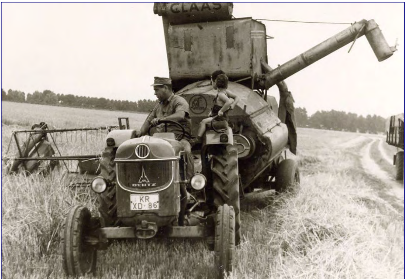
The development of a combine harvester in Germany was first started by the manufacturer Claas. In 1946, the machine was ready for series production. The result in the form of the trailed combine harvester Claas Super can be seen here in a later version with grain tank at the harvest behind a Deutz D40 tractor in 1969. Photo: Mgweb (public domain)
