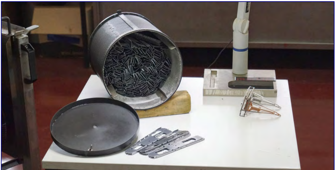
The cast housings are prepared for the further manufacturing and assembly steps using various deburring processes, including beam deburring (top photo). In electroplating, metallic surfaces are refined and hardened, and also chemically blackened. The opened, filled container (photo below) shows how the parts to be processed migrate into the bath.
