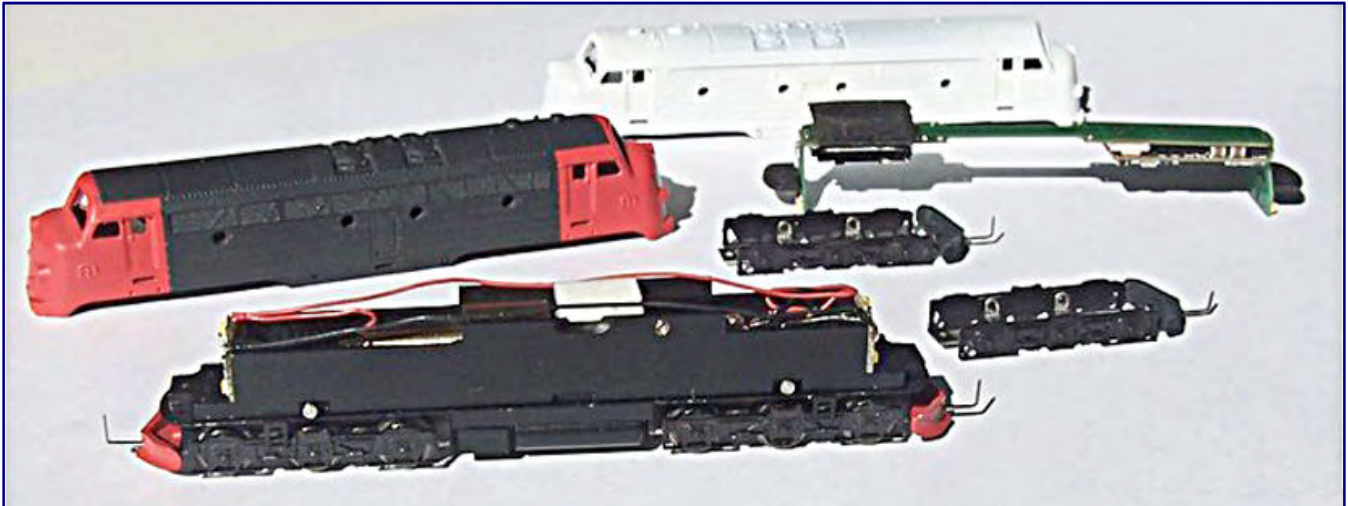
Delivery of a completely redesigned NOHAB diesel locomotive is scheduled to start in early 2019. It avoids the obvious mistakes of the Märklin model and can also be equipped with Velmo digital sound on request. Photo: FR Freudenreich Feinwerktechnik
