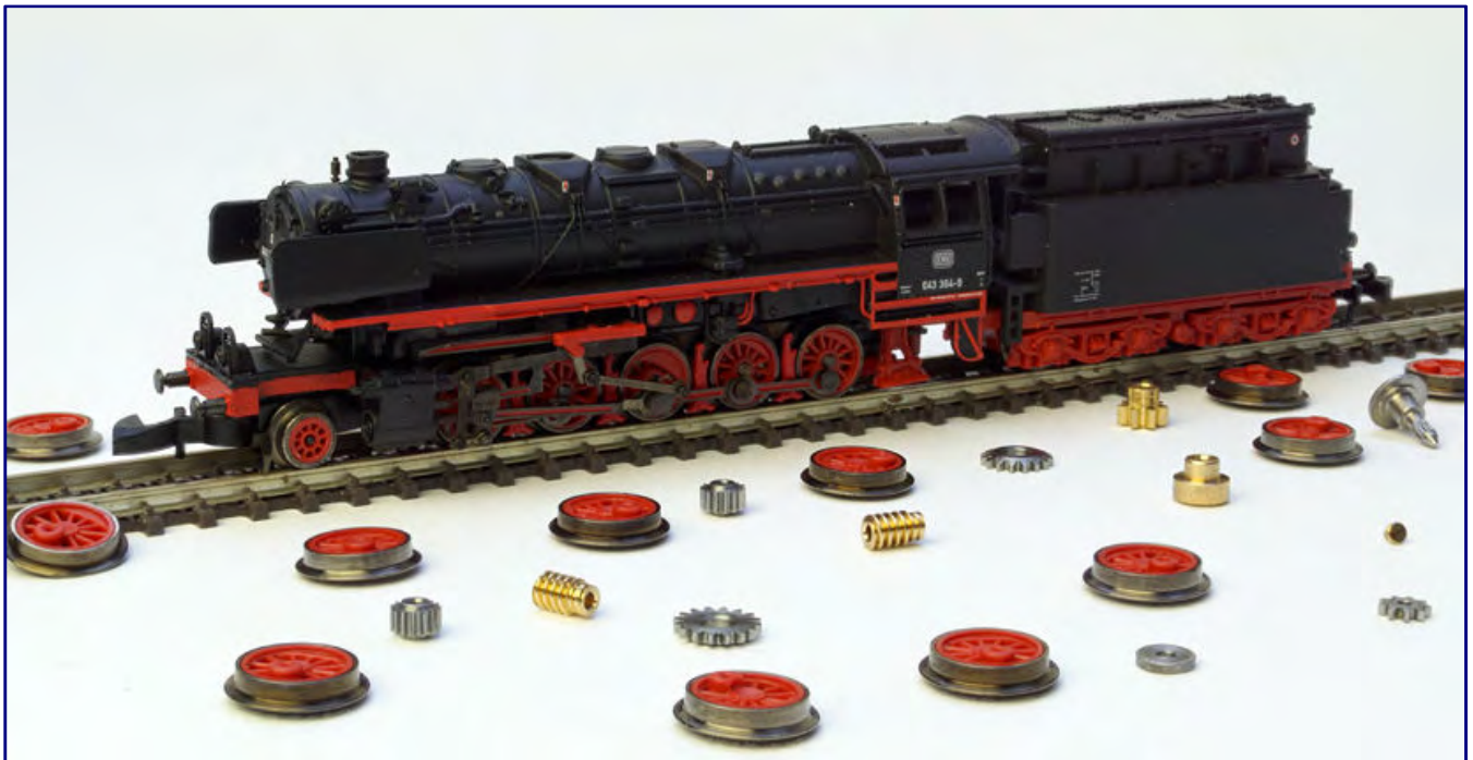
Examples of parts produced in or at least with the assistance of the automatic lathe shop: Steam locomotive wheels (with injection moulding insert), gear wheels, buffers, worms and, as the smallest parts, attachment bolts for the linkage of a Z gauge steam locomotive (shown far right in the picture).
