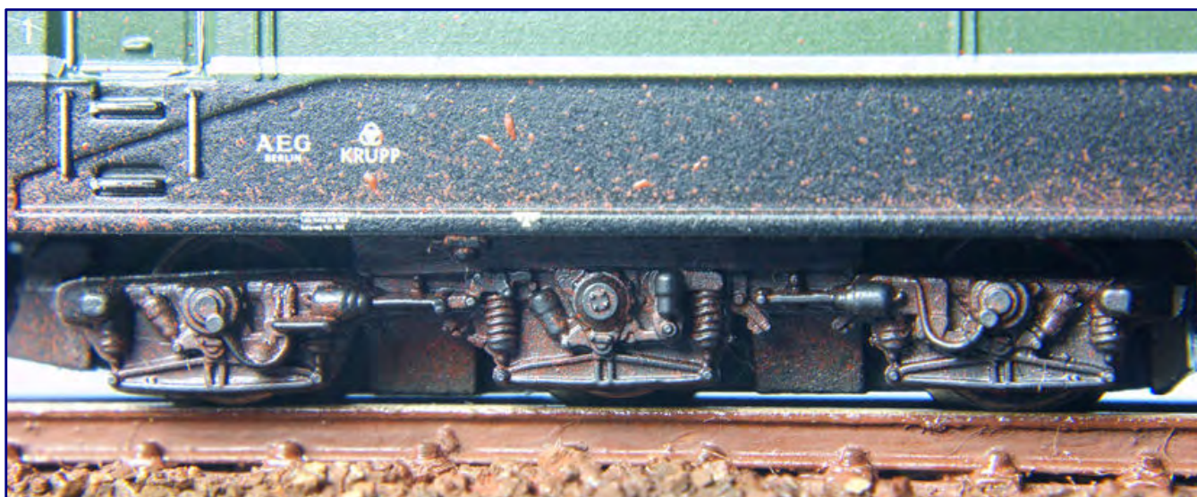
If a six-axle bogie with driven centre axle is not correctly assembled, all three wheels can usually be seen at the same height (middle picture). If the assembly is correct, however, the middle wheel is slightly higher (picture below), so that its tread has no track contact, as can be seen here in the macro picture.
