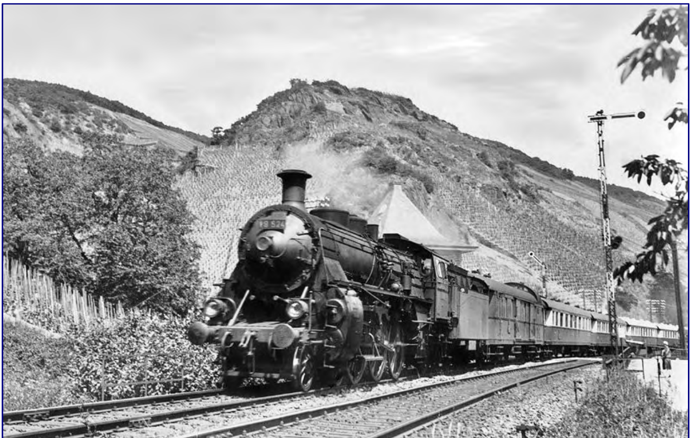
In 1930 when 18 524 the FFD 102 "Rheingold" passed the Peternach block station near Boppard southwards, it already had electric lighting, but no smoke deflectors. From our current point of view, the main signal with the negative sign on the arm also appears unusual. Photo: DLA Darmstadt (Maey) / Eisenbahnstiftung
