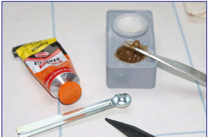
With Pattex Stabilit Express the zinc die casting and the brass casting are permanently joined. The adhesive is first filled deep into the boreholes before the adhesive seam between the two halves follows.
