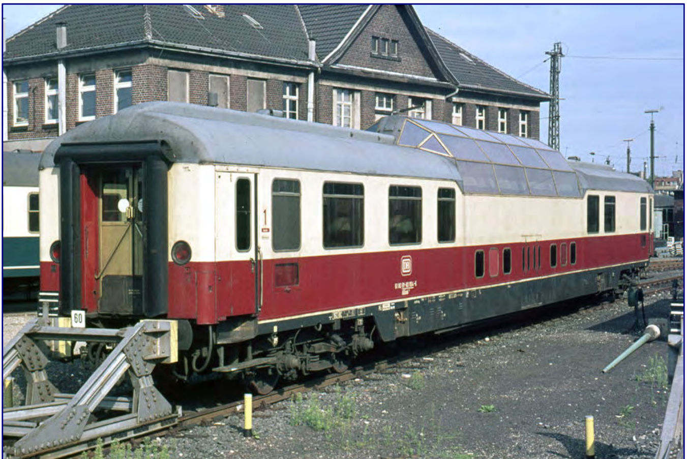
The special feature of the new “Rheingold”, apart from the Buckels dining cars, was above all the ADÜmh 101 observation car, which remained unique in Germany. With the upgrading to TEE, the trains soon changed their colours to purple/beige. The car 81 - 80 004 belongs to the replicas for the “Rheinpfel” from 1963, recognizable by only four side windows in the viewing area. Here the wagon is on 1 August 1976 for a revision to guest in the Bw Cologne Bbf. Photo: Peter Schiffer / Eisenbahnstiftung
