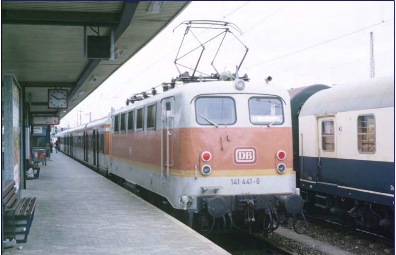
141 141-6 with time-division multiplex reversing train control was one of the seven machines destined for the new S-Bahn in Nuremberg. Here the locomotive with such a train from x-wagons waits as S 1 to Lauf (on the left the Pegnitz) on 1 October 1988 in Nürnberg Hbf for the departure. Photo: Archive Petkelis
