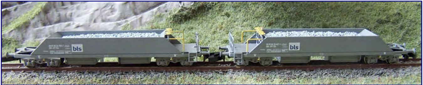
The Xas 73 new ballast wagons are currently being delivered as BLS rental vehicles. Photo: FR Freudenreich Feinwerktechnik
