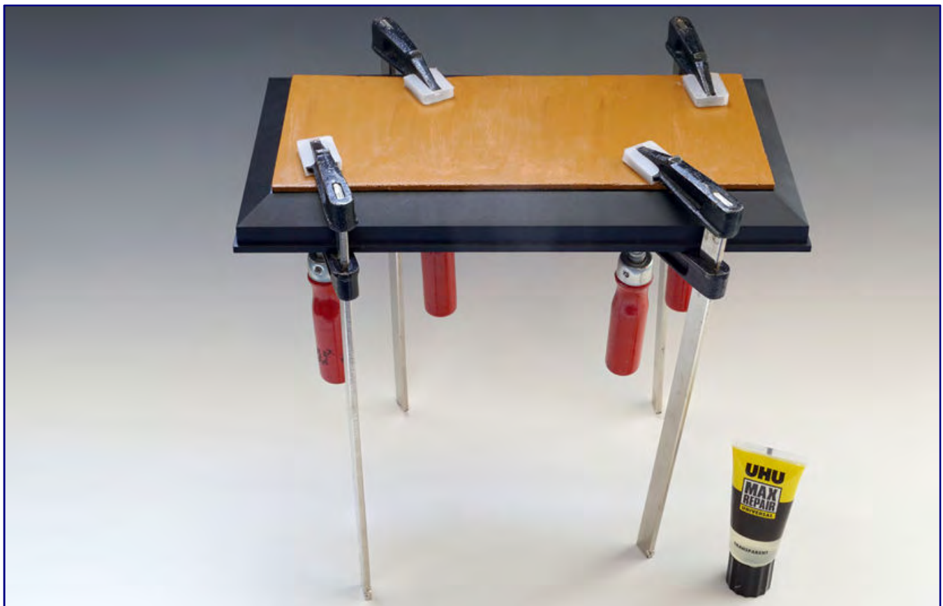
A lacquered plywood board forms the base for the construction of the diorama. It is glued to the plastic base with a special glue from Uhu and fixed there with screw clamps until it is completely dry.
