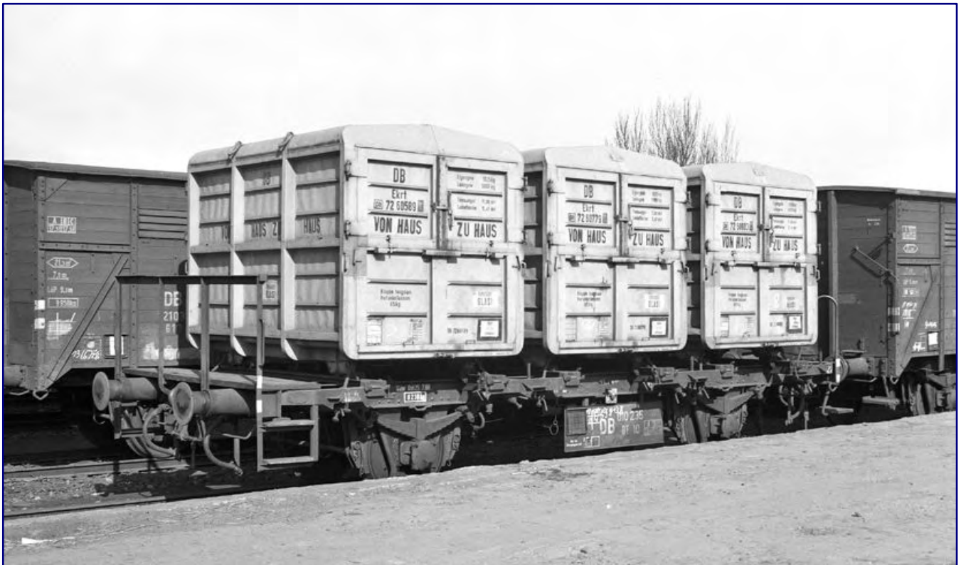
The container wagons BT 10 were created by conversion on old chassis of covered wagons of the types G 10 and G(r) 20. Two such donor wagons of the first type are located in Kassel in March 1961 next to and behind the wagon with the serial number 010 235. Photo: Reinhard Todt, Eisenbahnstiftung
