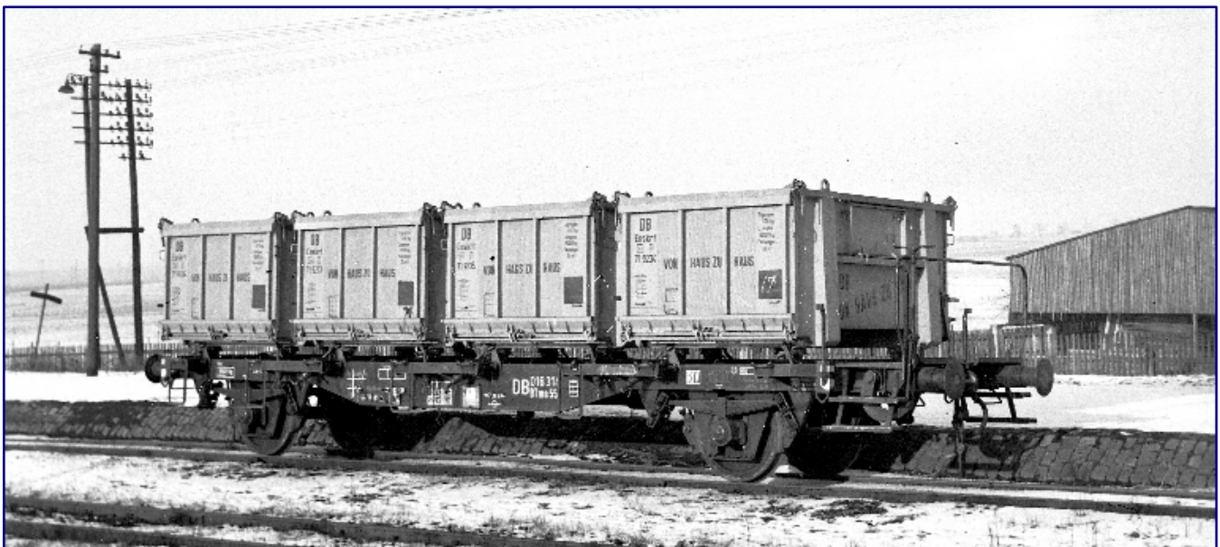
The tank wagon BTms 55, built in series from 1955, here the copy with the company number 016 314, marks the transition to the four-wheeled wagon. In January 1958 it was captured in the picture with Eoskrt 21 containers, which, raised with steel extension walls, would have been the correct model for Märklin's latest model. Photo: Reinhard Todt, Eisenbahnstiftung
