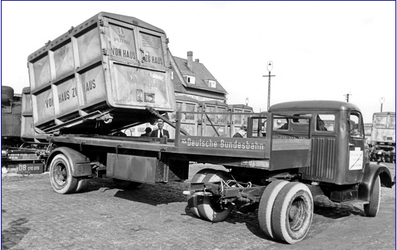
This semi-trailer, like the one on the photo on page 22, comes from the Bochum bus, bus trailer and vehicle manufacturer von Lienen. The photograph taken in Bochum in 1961 shows us how this solution required the vehicle to approach the train and the Pa containers to be transferred. Photo: Barnarius, Eisenbahnstiftung
