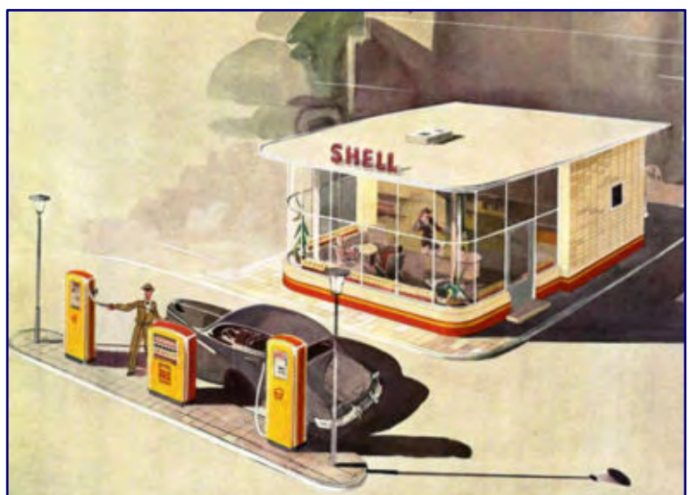
A company-specific architecture was also characteristic of the post-war history of petrol station chains. At first, Shell did without a canopy and let the glass front of the cashier's office take effect for itself. A typical stylistic element was the lanterns that bordered the tank island. Photo: Sammlung Ulrich Biene
