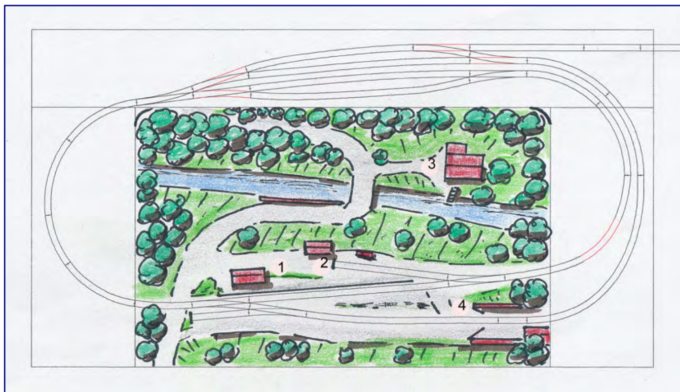
Simple track plan (top) with the different sections measured in centimetres. Bottom: scenery proposal with 1 depot, 2 loading siding, 3 farm house, 4 industrial access.
