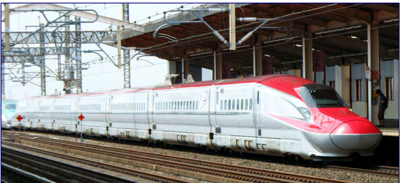
Not all Shinkansen lines stop in Oyama and so the trains can be observed here on the middle tracks even when passing through at top speed. However, this double unit consisting of an E5 (rear) and an E6 (front), which could be stopped in full length, made an intermediate stop on 14 May 2016.
