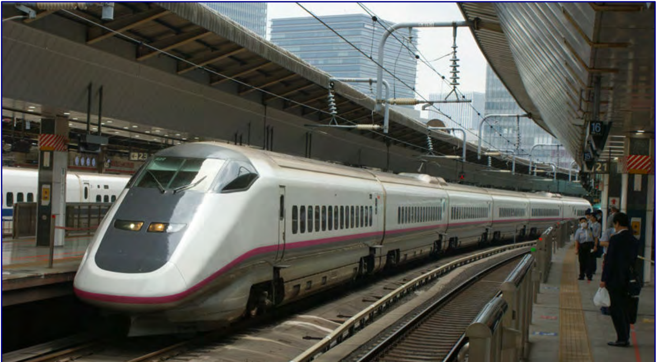
The Shinkansen E3, which was also in Tokyo on the same day, only ran at a maximum speed of 275 km/h. The six-piece set had the same space capacity as its successor, which was longer by a middle car.
