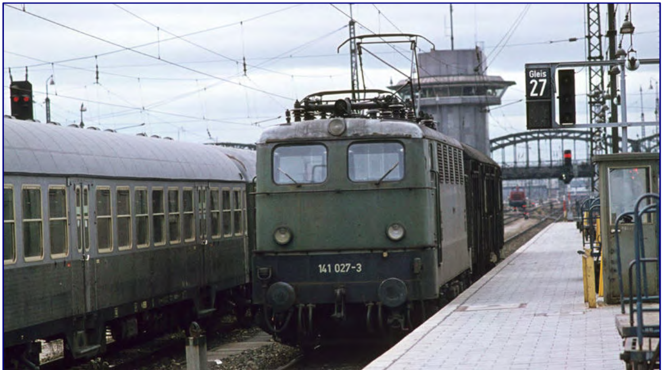
141 027-3 is still largely in its original condition on 10 November 1974 when manoeuvring in the Starnberg wing station (Munich main station), with a circumferential rain gutter, step grating and holding bar as well as the original lamps and silent fans. Only the signage was adapted to the computer age. The sounds of the rear derailer and the chrome-oxide green colour earned the series the nickname "firecracker." Photo: Eckerle, Archive Petkelis
