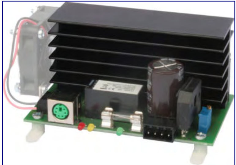
View of the open power section of the GFR1500 with attachable fan. Photo: Heißwolf Modellbahnzubehör
