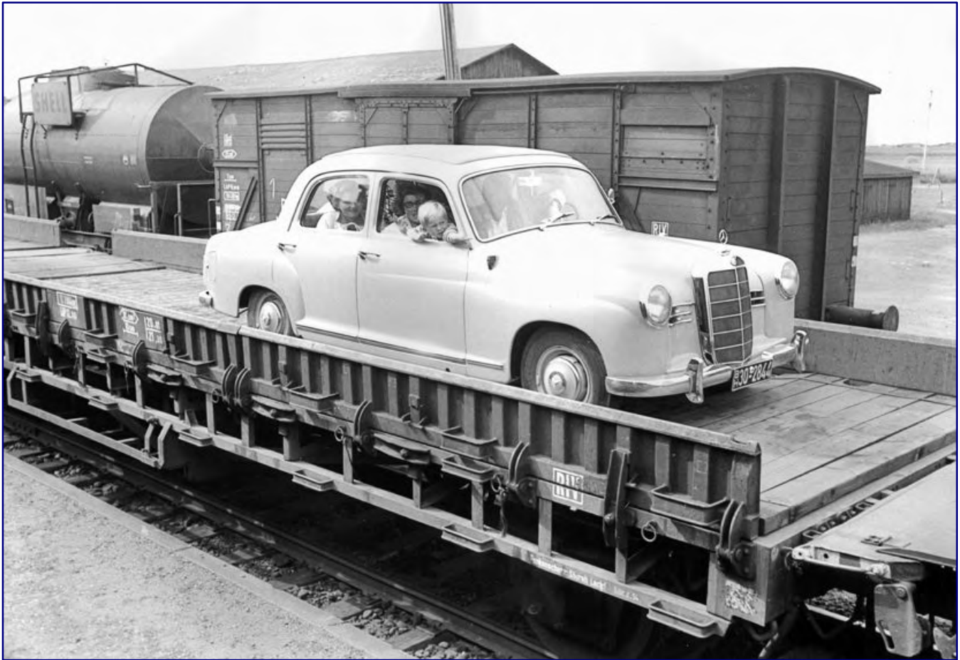
Motor vehicles of various types were also among the typical loads of low side and stanchion cars. Between 1950 and 1953, the DB equipped 25 wagons with heating cables for Sylt traffic in order to place them between the locomotive and the passenger coaches. In 1955 in Niebüll, a Mercedes-Benz 180 D with a pontoon body was driven onto a stake car of the type Rmmhs 31. Photo: Walter Hollnagel / Eisenbahnstiftung
