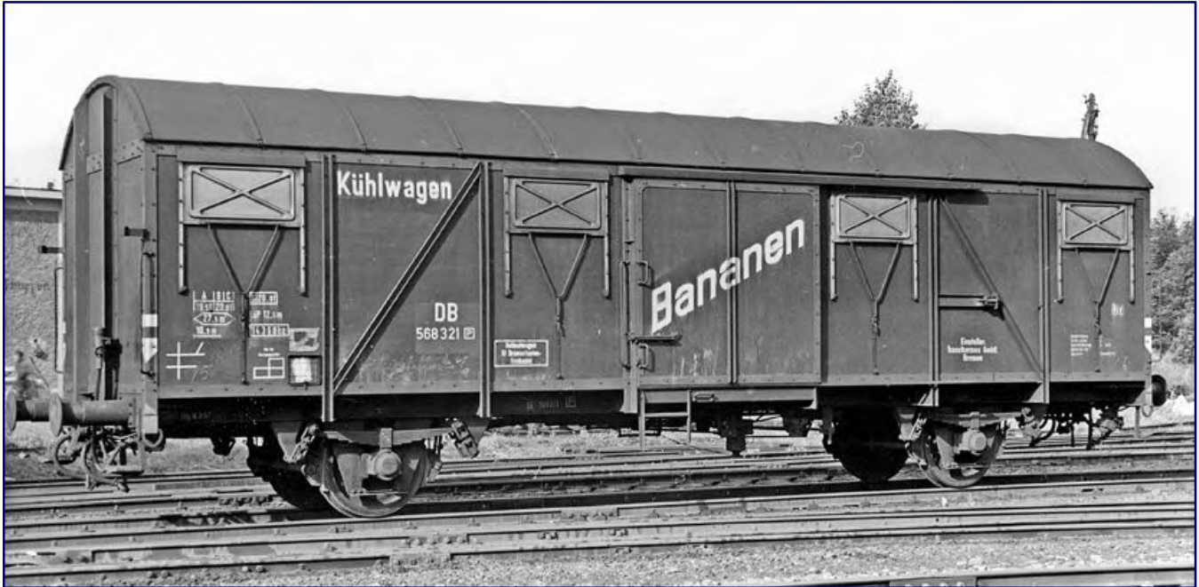
The Tnohs 59 heat protection wagons for the transport of bananas were prepared from covered freight wagon of the genus Glmhs 50. They had a superstructure with synthetic resin wood panels, which was to become standard in the future. When the car with the company number 568 321 [P] of Transthermos GmbH Bremen was registered in 1957, it was still almost brand-new and showed few traces of operation. Photo: Bustorff, Eisenbahnstiftung
