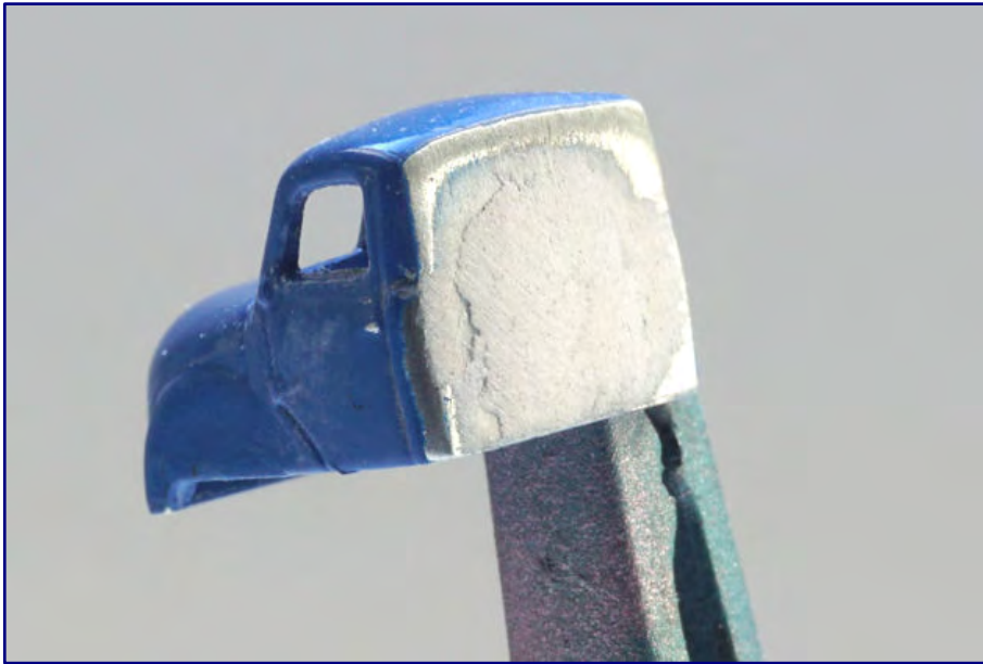
Before the filled area can be repainted in the cabin colour, the surface must first be sanded smooth.
