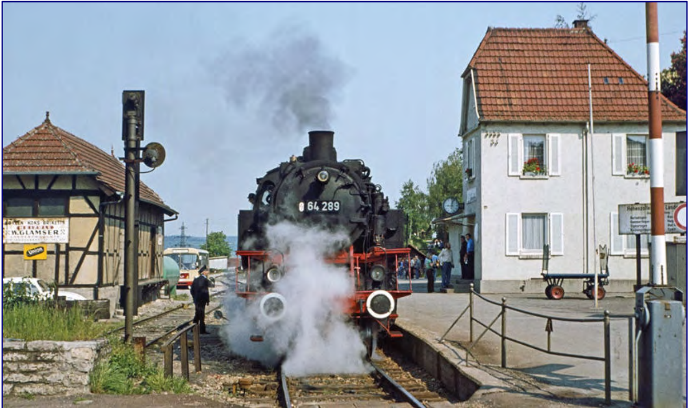
When 64 289 was photographed on 30 May 1977 on the Zollernbahn in Hechingen, it shows a different appearance than our model. The smoke chamber supports and ladders have been painted red, and the buffers are decorated with a warning coat of paint. Photo: Wolfgang Bügel
