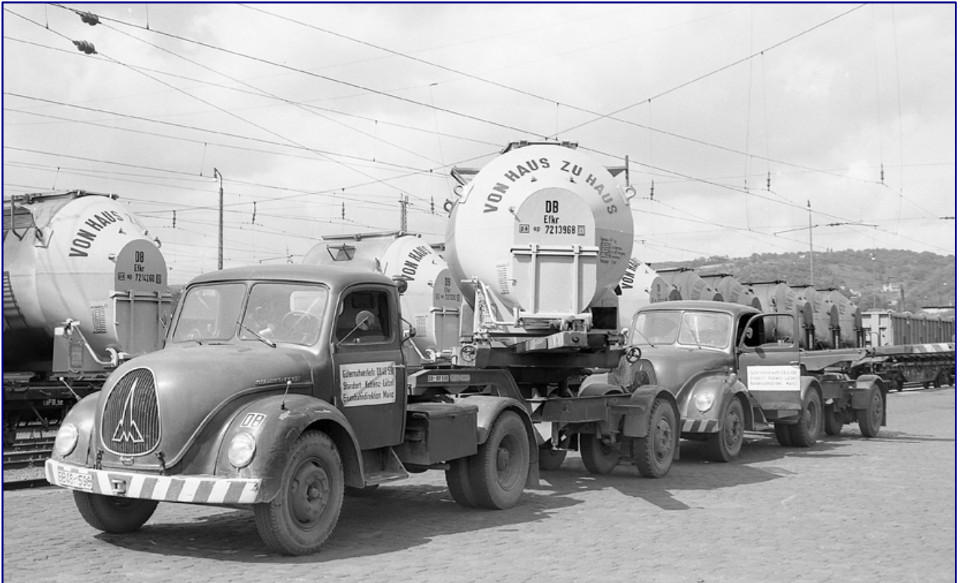
In August 1961, the loading of an Etkr container for fine bulk material by an Ackermann delivery vehicle was recorded in a sequence of pictures at the Koblenz-Ehrenbreitstein railway station. The vehicle with the registration number DB 49-596 drove parallel to the train on the loading road and swivelled the trailer 90 degrees over to the container wagon BTs 50. The Pa container is then rolled on rails onto the trailer and lashed there (top photo). Once it has been fixed securely for transport, the trailer swivels in again (bottom photo) and assumes its travel position. Photos: Slg. Eisenbahnstiftung
