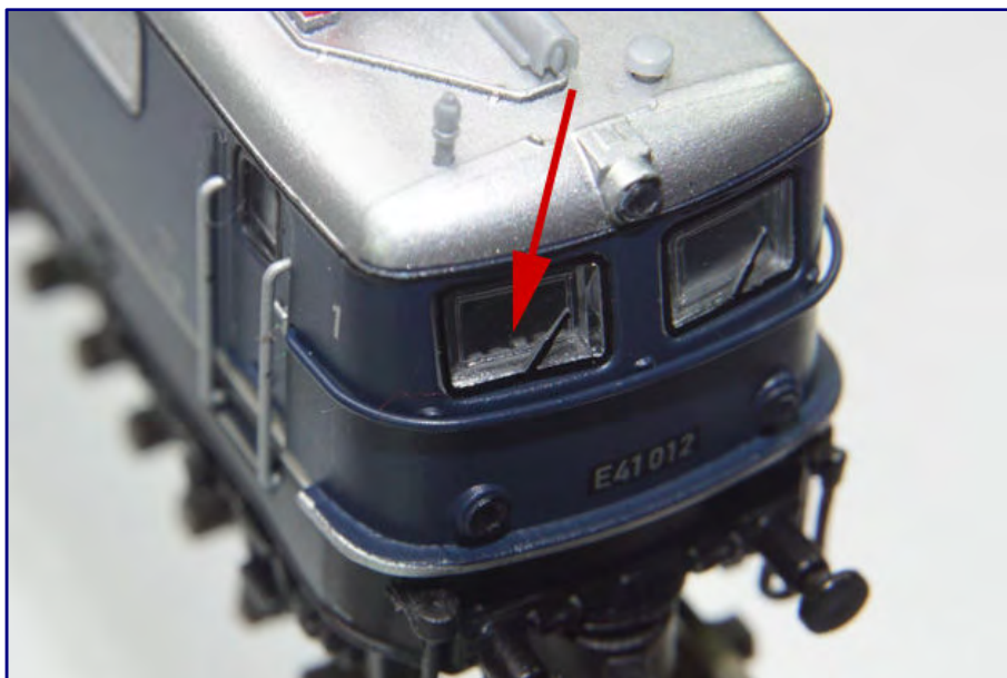
Even the interior of the driver's cab is partially reproduced, but this is barely recognizable through the transparent panes visible in the window surfaces. Nonetheless, we managed to make the relief of the display devices and indicator lights visible in the photo.
