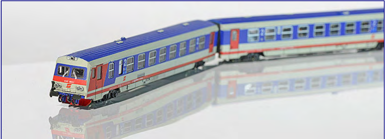
SMZ attracted attention in mid-2018 with the design of a kinematic close-coupling for Z gauge. For the first time, the Rh 5047 diesel multiple-unit train from ÖBB was equipped with it. Photo: Sondermodelle Z
