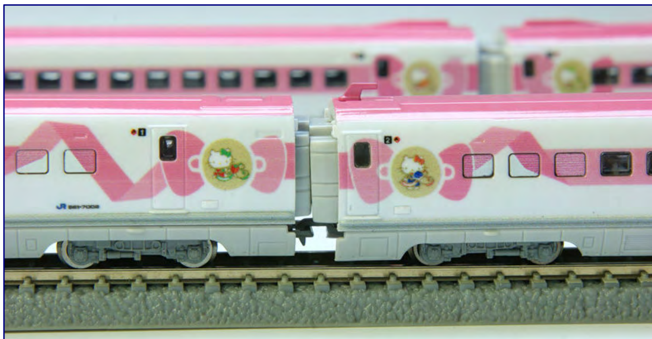
A horizontal ribbon covers the window areas in a straight line, interrupted by frequent upward and downward folds (top). All decorative motifs have been digitally printed onto the bodies. This is in particular evident from the halftone dots visible on the regional Hello Kitty motifs (bottom), shown here at the intersection between car 1 and 2.
