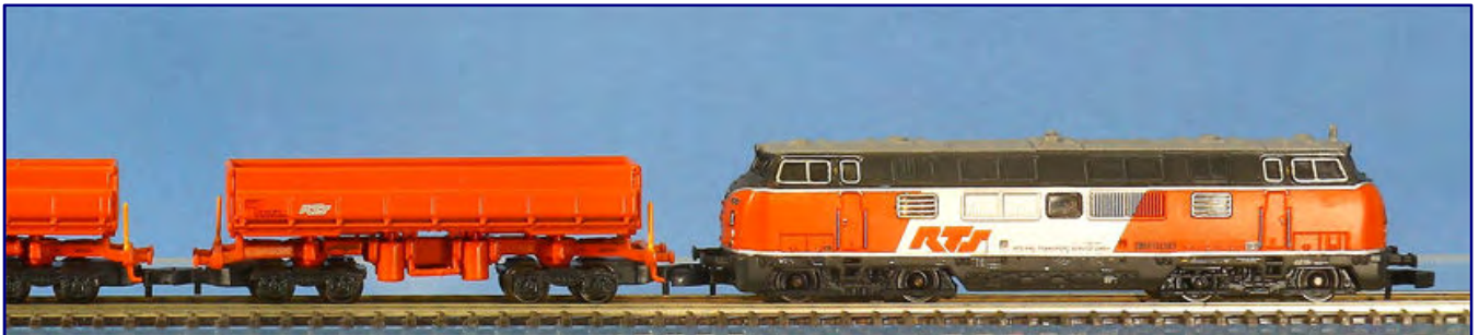
The RTS train, consisting of a class 221 diesel locomotive (88204; right) and three Eamos dump cars (82435; left) belongs to the current era VI.
