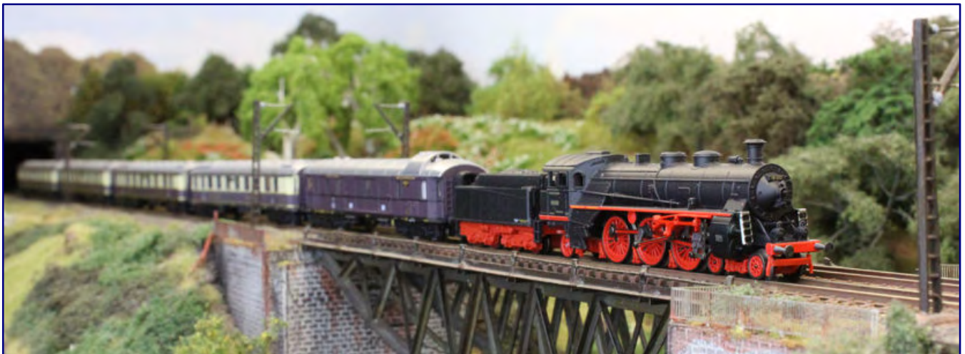
The Rheingold for epoch II (Art.-No. 81332) now appears with close couplers. Locomotive 18 433 has no smoke deflector plates yet, but is equipped with bell-shaped armature motor, detail control, brake imitations and track clearers. Photo: Jörg Erkel / 1zu220-Shop
