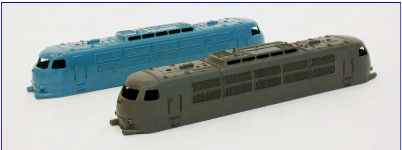
The addition of metal particles changes the colour of the material: The ABS plastic body shell is blue, whilst the metal filled plastic shell of the class 103 locomotive takes on the grey colour of the tungsten metal.
