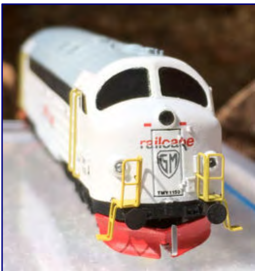
The TMY 1150 (46.125.01; photo above) from Railcare is not a pure colour variant, as can be clearly seen. It carries a front door below the top light (photo below left) and a different snow plough. The buffer ascents with railings also attract the attention of the observer (photo below right). Photos: Harald Möller
