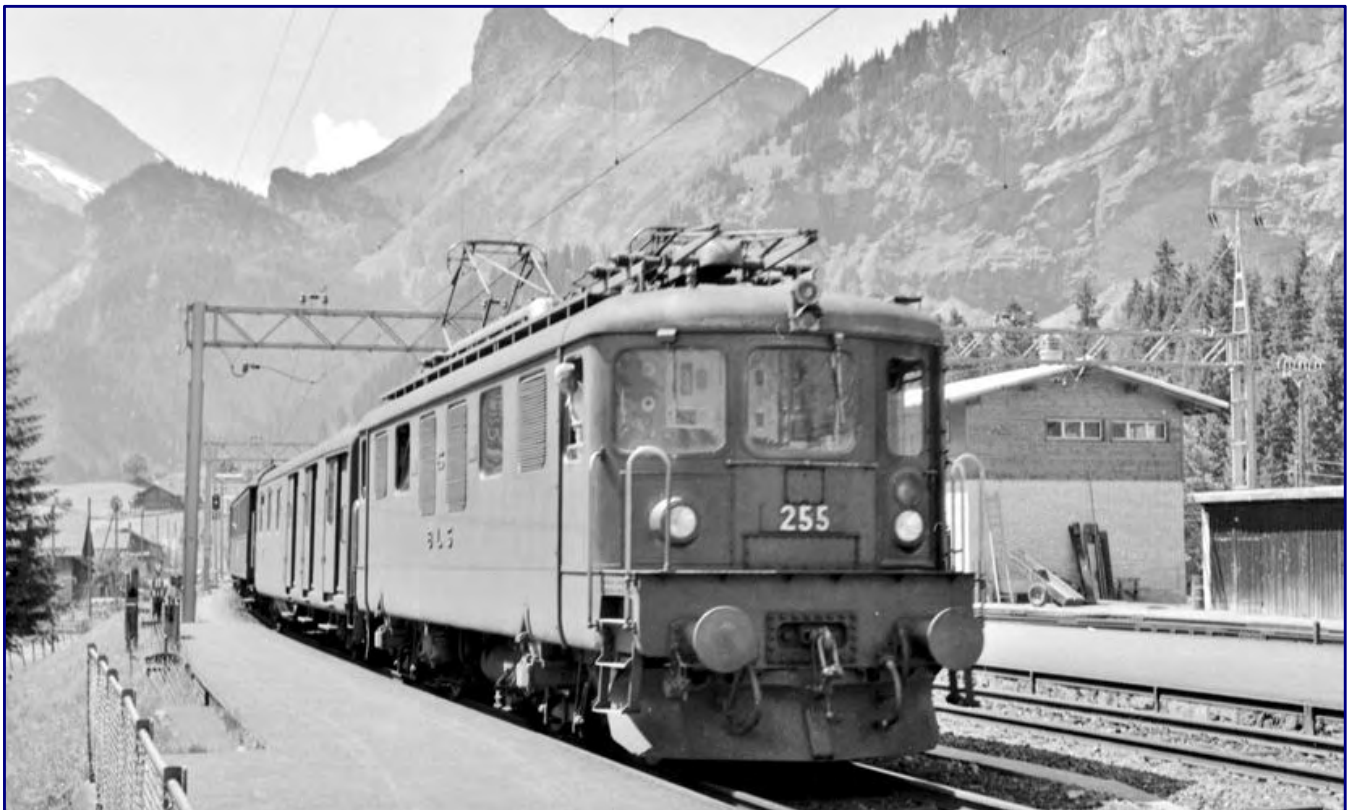
The Ae 4/4 of the BLS was an electric locomotive without a drive shaft, on which the DB could orient itself. In 1944/45 two units were purchased, followed by six more by 1954. Here the Ae 4/4 255 entered Kandersteg in June 1956 with express train 133. Photo: Kurt Eckert, Collection of Eisenbahnstiftung
