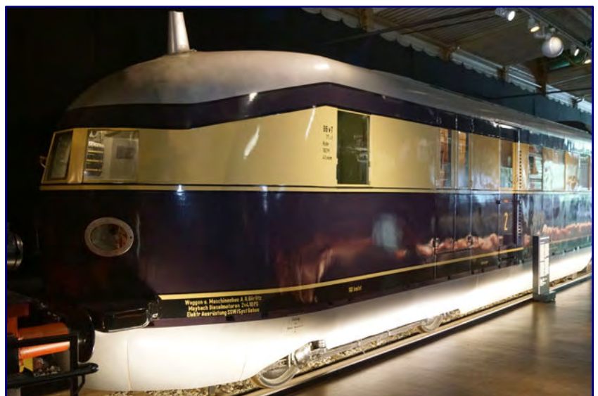
The "Flying Hamburger" in the shape of a SVT 877. Unfortunately, only one section of this diesel rail car remains, albeit in excellent condition.
