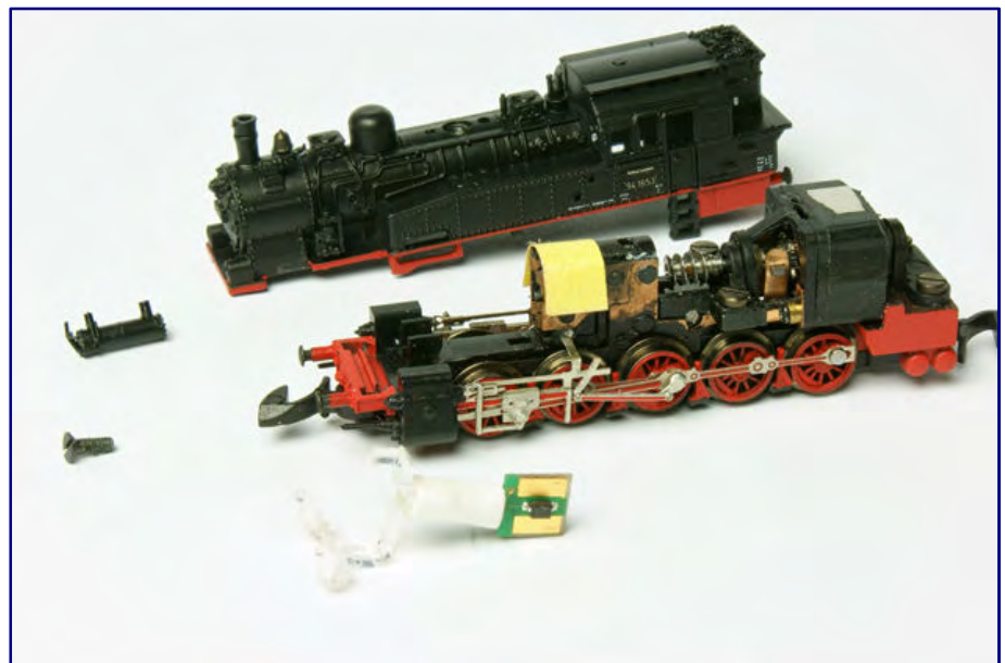
The LED insert of the 01 series can be used to upgrade the direction-dependent front lighting. We have pulled the white shrink tube of the former bulb over the LED and the transparent insert.
