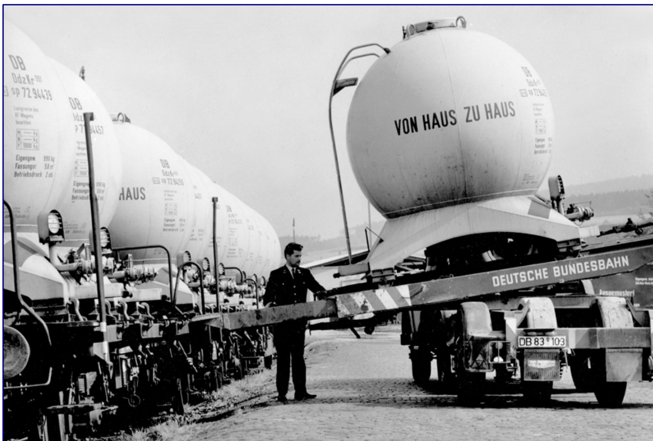
The cement tanks on a BTms 55 in Letmathe (March 1965; photo top) and the spherical tanks for compressed air discharge Ddzkr 551 (1961; photo bottom) are further examples of the many special tanks. Photos: Reinhard Todt, Railway Foundation (top) / Helmut Först, Eisenbahnstiftung (bottom)
