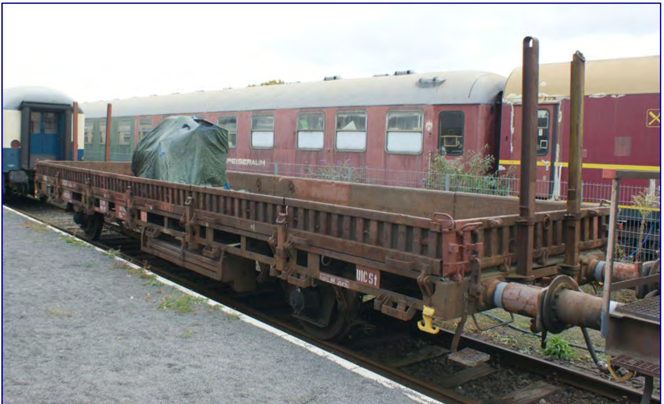
As with the new Märklin models, the front stanchions of this Kbs-type wagon are inserted from DB AG stock. The side stanchions, are stored in the pockets under the floor on the long side of the wagon.
