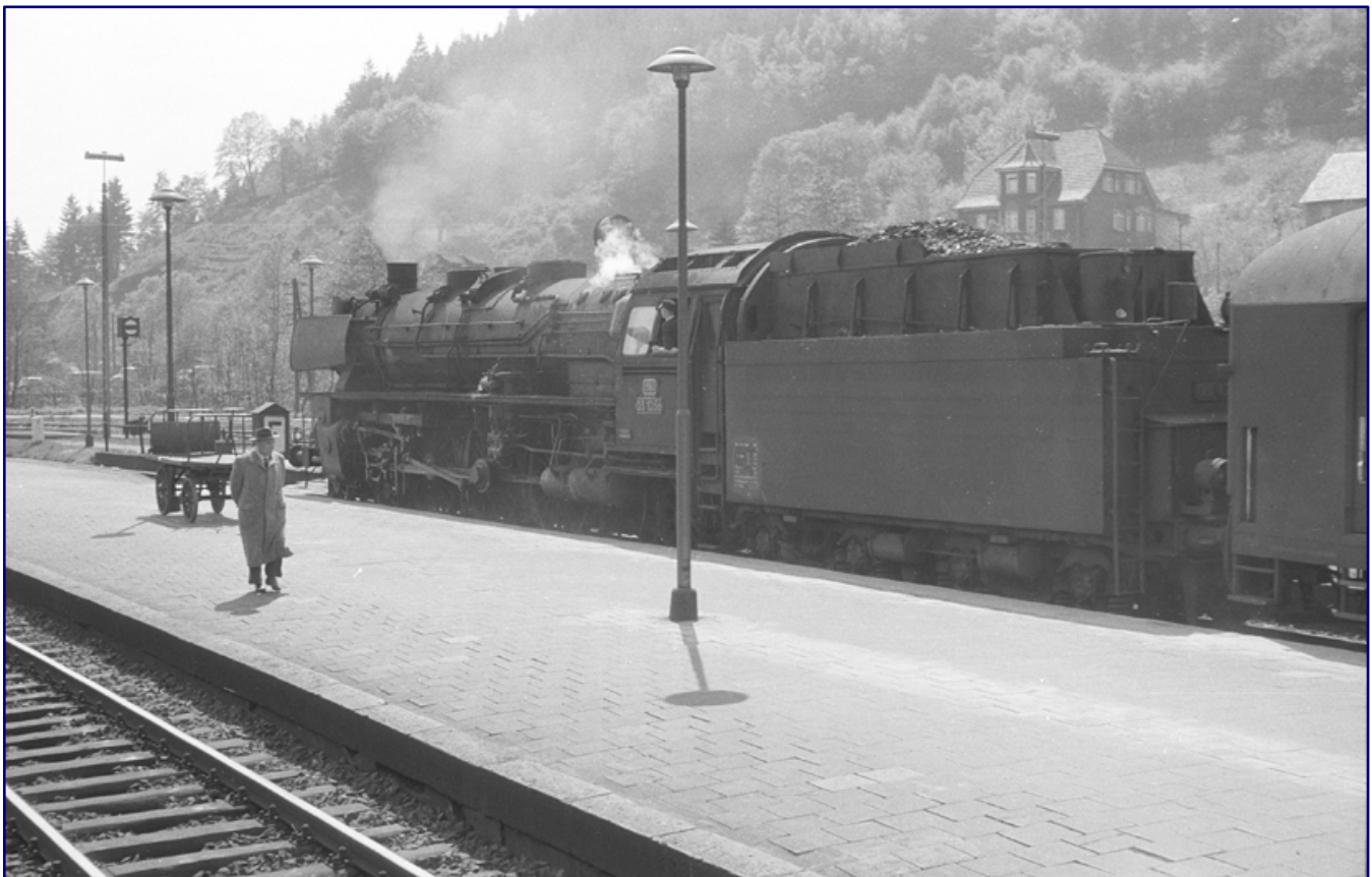
03 1056 is in use here, presumably in Brilon Wald, in the condition after its de-energization and reconditioning at Henschel. The surface preheater is still in front of the chimney. The tender has also already undergone initial modifications, as can be seen on closer inspection. At the time of this picture, the locomotive, which was the last to receive a high-performance boiler, was probably already at the Paderborn depot. Photo: Walter Patzke, Archiv Petkelis
