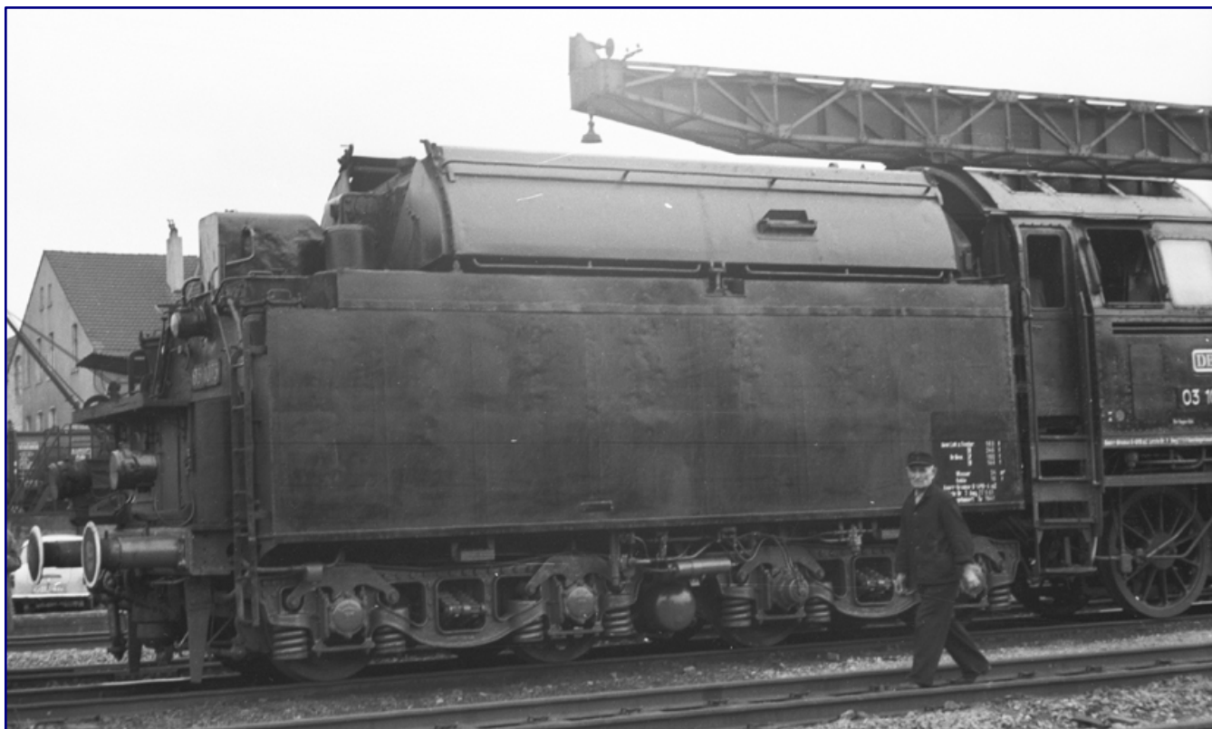
View of details of 03 1073 during the exhibition, including the closed cab with doors and the signs moved forward because of the rail inductive train protection equipment (picture above), as well as the tender with open coal box cover, replenishment equipment and buffer plate warning paint (photo below). Photos: Walter Patzke, Archiv Petkelis
