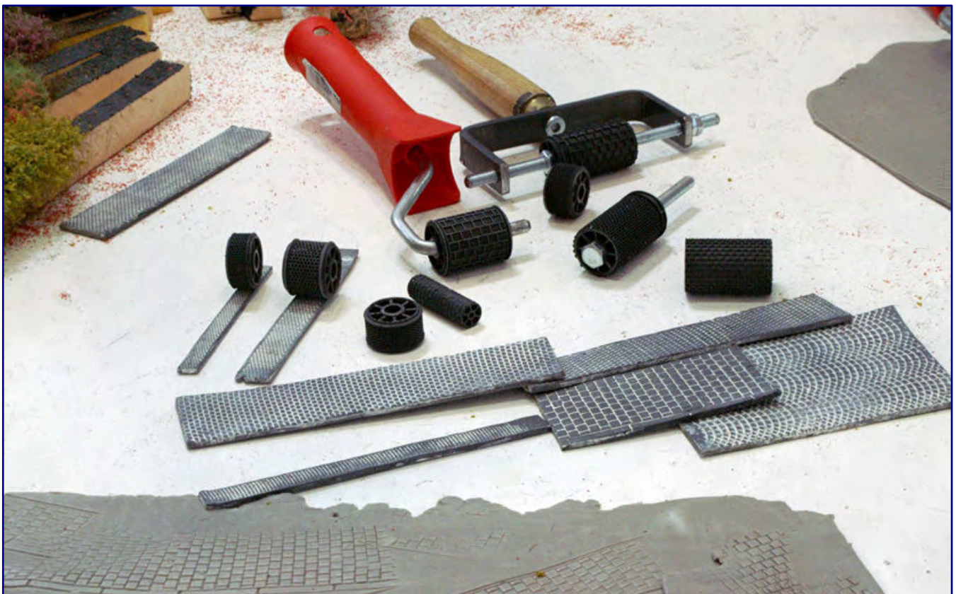
Among the various embossing rollers for paving there are also those for Z gauge. The rolled out, hardened and coloured material illustrates the working method of the Microrama product.
