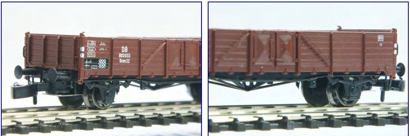
Fine details characterise the models, which are accurate to a tenth of a millimetre in all important prototype dimensions: shunter handles under the buffers and brakes at wheel level (photo left), as well as the correctly reproduced truss behind the fish belly, rope eyelets, and tank hooks (photo right).
