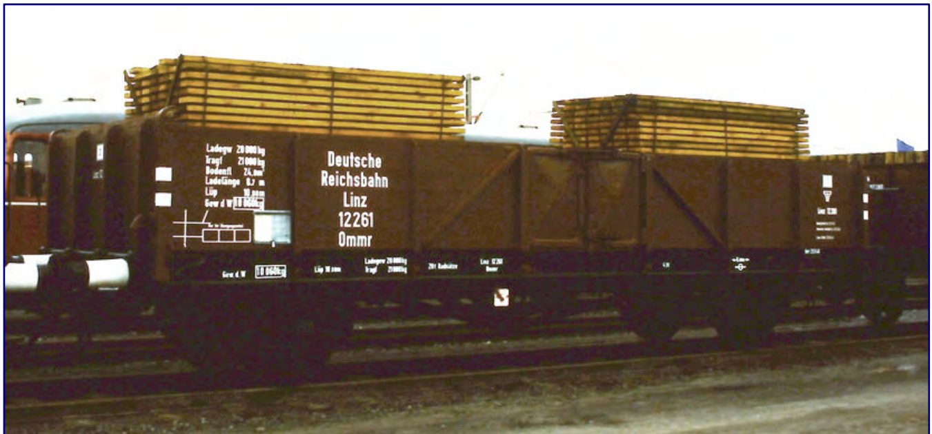
This reconditioned Linz also took part in the anniversary exhibition in October 1985 in Bochum-Dahlhausen. It is a representative of the design, as built, from 1941 to 1943. Photo: Manfred Kopka (CC-BY-SA-4.0)
