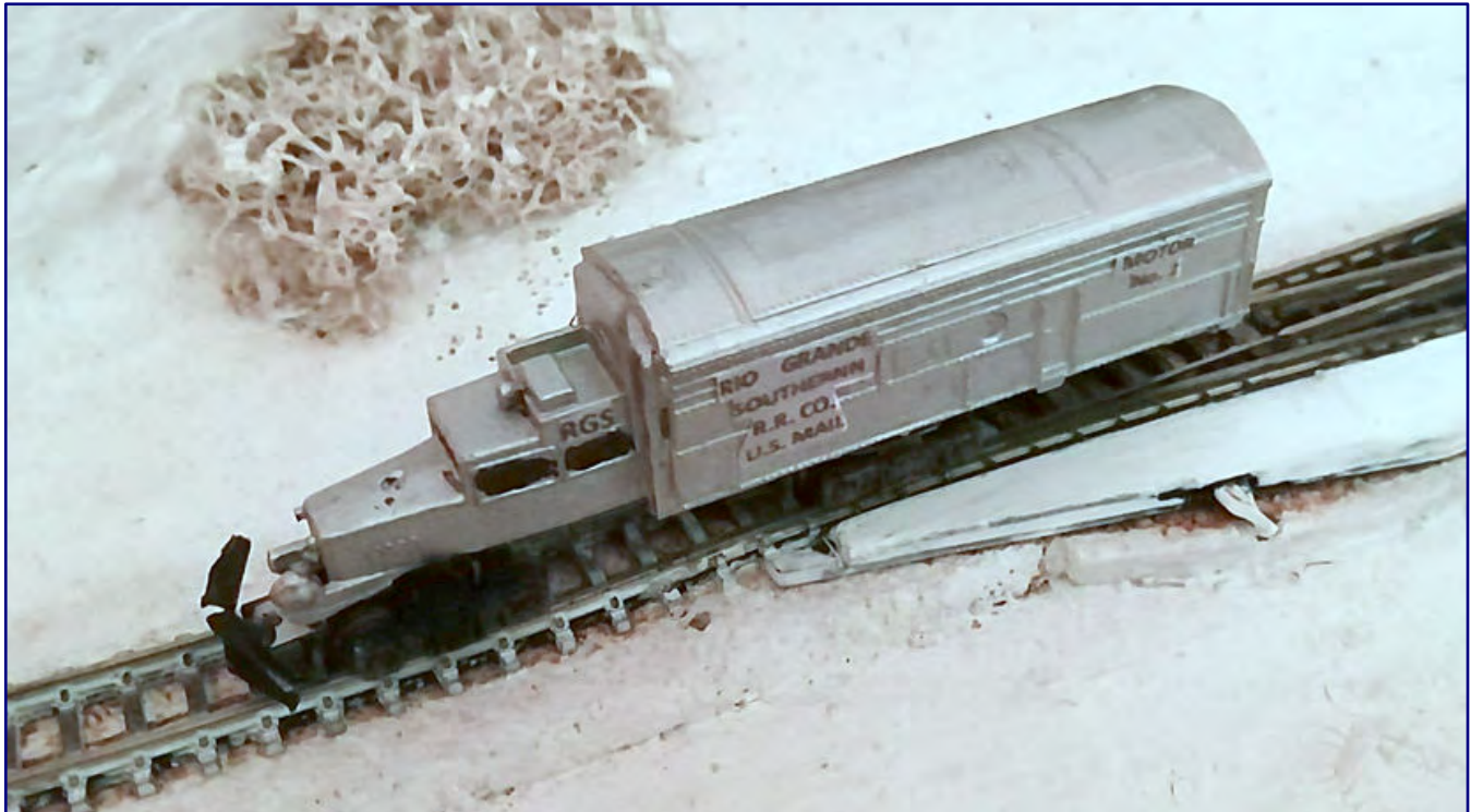
A look at the roof of the finished model shows that the fan rotors of the EMD F7 have disappeared: scraped off, sanded, filled and painted. Photo: Markus Krell
