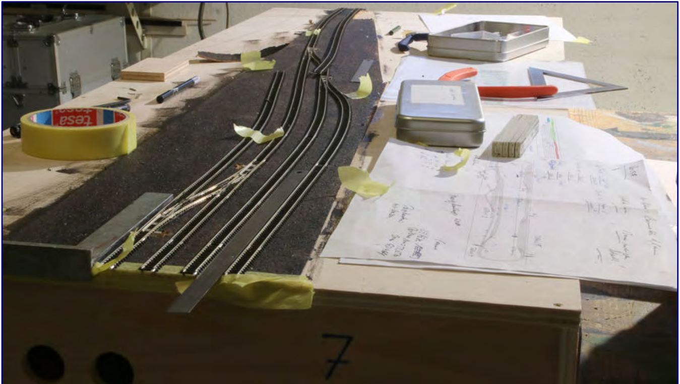
The turnouts are mounted with their lateral boxes removed to prepare for an underfloor drive. Careful attention is paid to the correct track spacing, which is "staked out" with a ruler.
