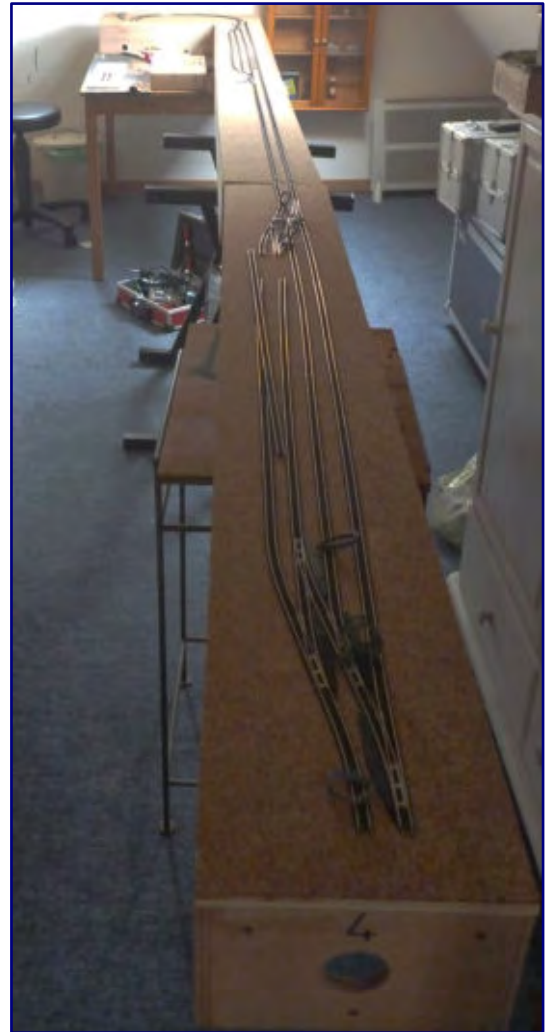
A 3 mm cork layer is placed on the finished boxes. This is followed by the trial construction of tracks in order to better assess the plan.
