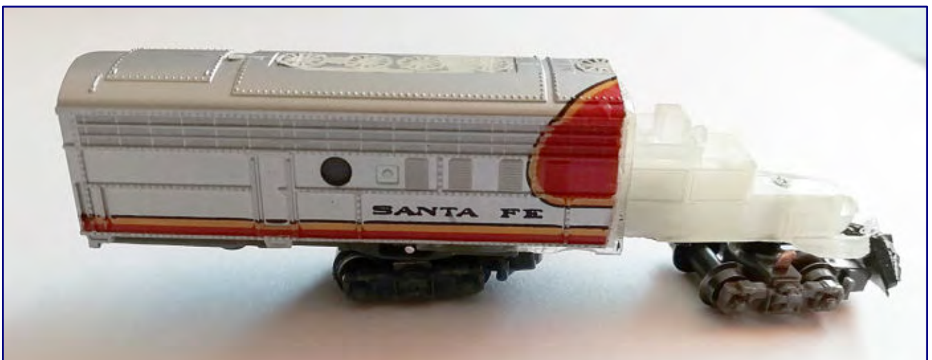
Image of the 3D printed model with its already modified body, the split Shorty chassis and the unpowered bogie bolted to the front of the hood. An EMD F7 shell from Märklin was reassigned and used for the superstructure, with the roof already having undergone some initial adjustments. Photo: Markus Krell
