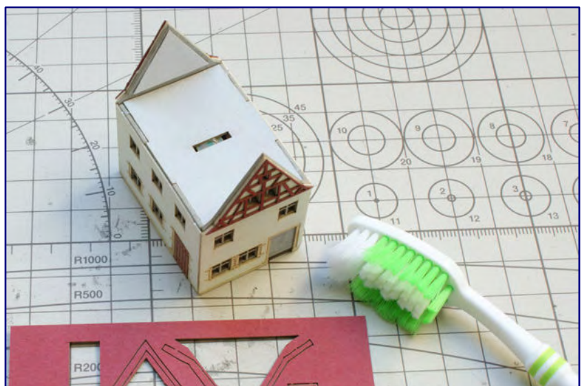
Traces of burning on laser-cut cardboard parts can best be removed with an old toothbrush.
