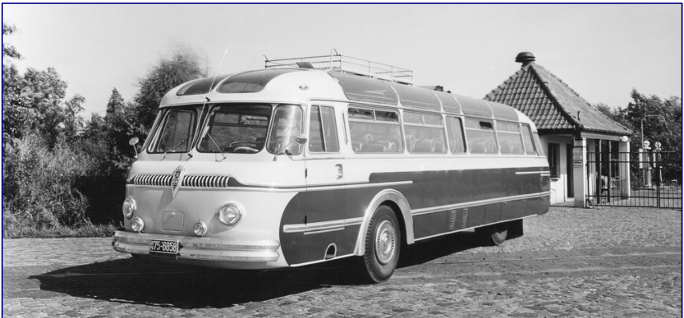
The basic model was also built as a coach version with the air-cooled KHD engine and was then called BS 311 at the factory. Roof edge glazing and roof rack were features of more upscale equipment at that time. Photo: Factory photo NWF, Archive Bernd Coldewey
