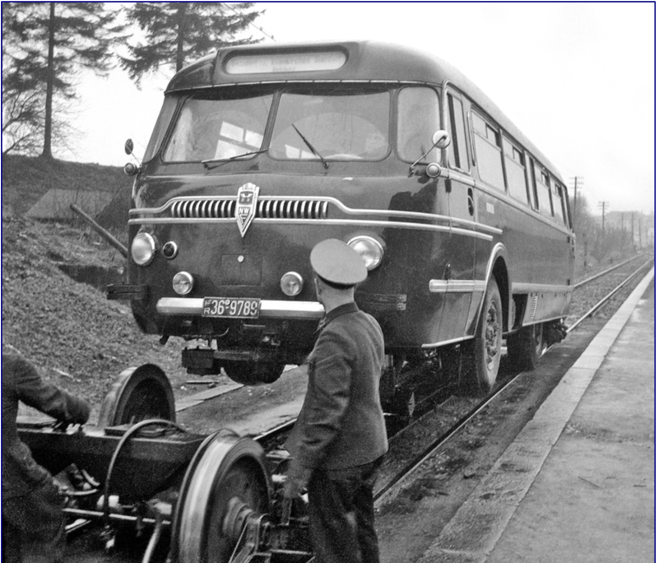
When the Schienen-Straßenbus (rail-road bus) with the French crew registration number FR 36-9789 is put on the tracks in Dierdorf (Westerwald) in April 1956 to continue its journey to Altenkirchen, it also demonstrates the work of the two front hydraulic rams of the series vehicle. Photo: Reinhard Todt, Eisenbahnstiftung
