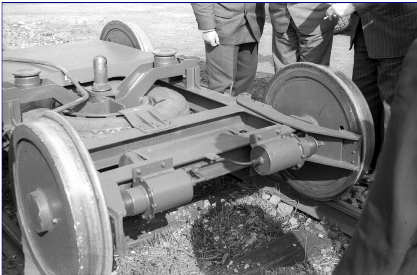
Here, according to records in May 1954 in Dürrstadt, the vehicle based on a Krauss-Maffei bus with the crew registration number AB 06-5410 is placed (photo above). The view on the track car also shows the brake cylinders and the supply lines (photo below). Photos: A. Dormann, Slg. W. Löckel (Eisenbahnstiftung)
