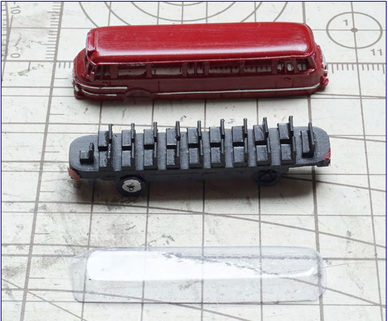
The rail-road bus was constructed in three parts: The body and chassis are made separately from resin, the window replicas are transparent deep-drawn parts.
