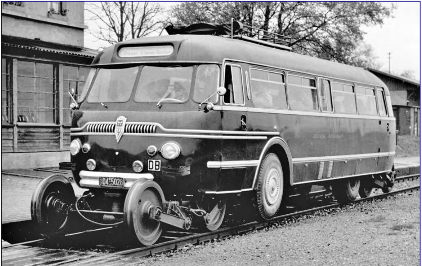
The Schienen-Straßen-Omnibus (road-rail-bus) (so named in the destination display) with the crew registration number AB 04-5028 shows the final series version of the bus and gauge coach in 1954, which was also selected for the Z gauge model. The front and rear entrance doors on the left side of the vehicle can be seen clearly; a sanding device on the gauge cars is still missing. The roof rack is only visible on some Schi-Stra-Bus. Photo: Below, Eisenbahnstiftung
