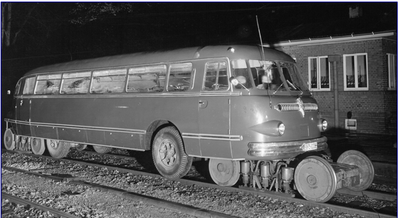
On this undated factory photograph, one of the vehicles, registered in Wilhelmshaven, is undergoing test runs with modified bogies (track cars) of the prototype type. Here, three brake cylinders on each side do not act on the disc wheels, but on a track support which is pressed onto the track similar to a magnetic rail brake. Photo: Factory photo NWF, Archive Bernd Coldewey
