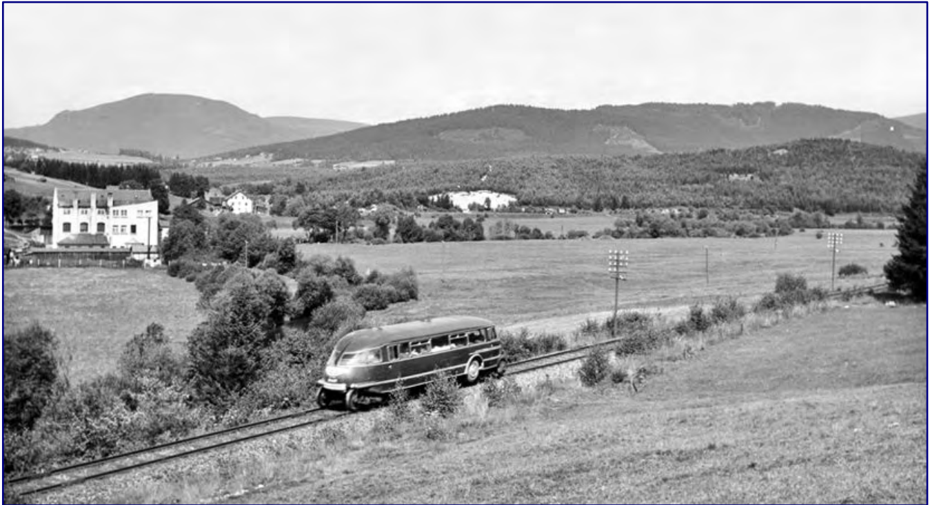
One of the first three Schienen-Straßen-Busse (rail–road-buses) from series production was captured in the picture on 10 August 1953 on the journey from Zwiesel to Grafenau. This first connection had been made a few months earlier and remained in service until the end of the summer timetable in 1956. Photo: Below, Eisenbahnstiftung
