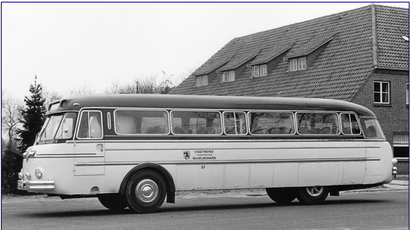
The Schi-Stra-Bus was derived from ordinary road vehicles. The road version of the series vehicle was this NWF BS 300, also powered by a KHD engine, and the specimen with Wilhelmshaven crew registration number was intended for the local public utility company. Photo: Factory photo NWF, Archive Bernd Coldewey
