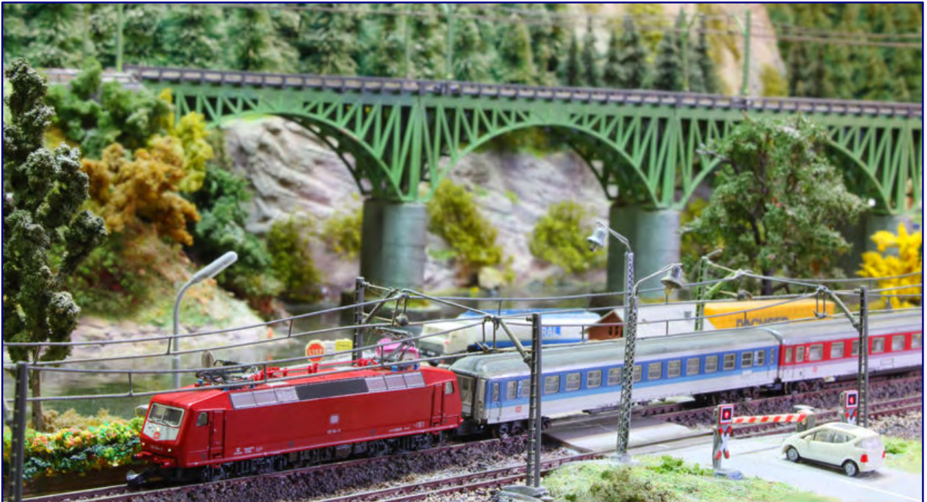
A class 120 Interregio passes through Märklin's half-barrier railroad crossing, which has been fitted with a Lemaco motor drive so that the barrier beams rise and fall in accordance with the original.
