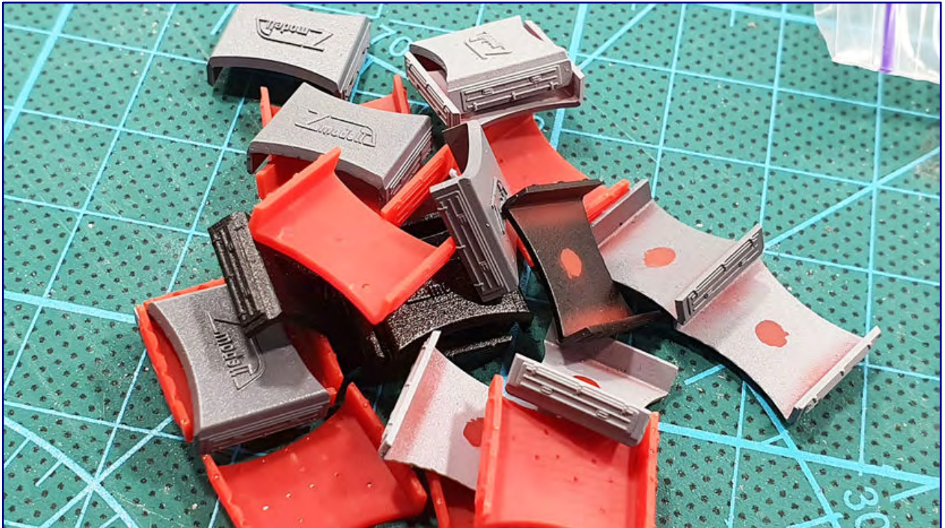
The milled central parts of the original electric loco cast block were covered with parts printed in the SLA process, which simulate the fuel tank of the diesel locomotive mounted between the axles.
