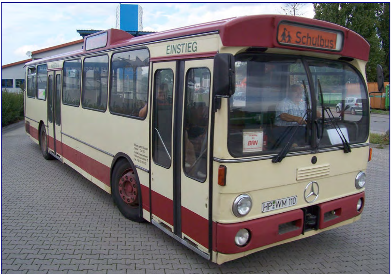
This Mercedes-Benz O 305, which was photographed in Heppenheim on September 26, 2005 and is still active as a school bus, is part of the original design to which we also want to adapt our model. In comparison to the example on page 19, differences can be seen above all in the smaller windshield, the resulting deviations in the front and the indicators mounted on edge. Photo: LosHawlos (CC BY-SA 3.0)
