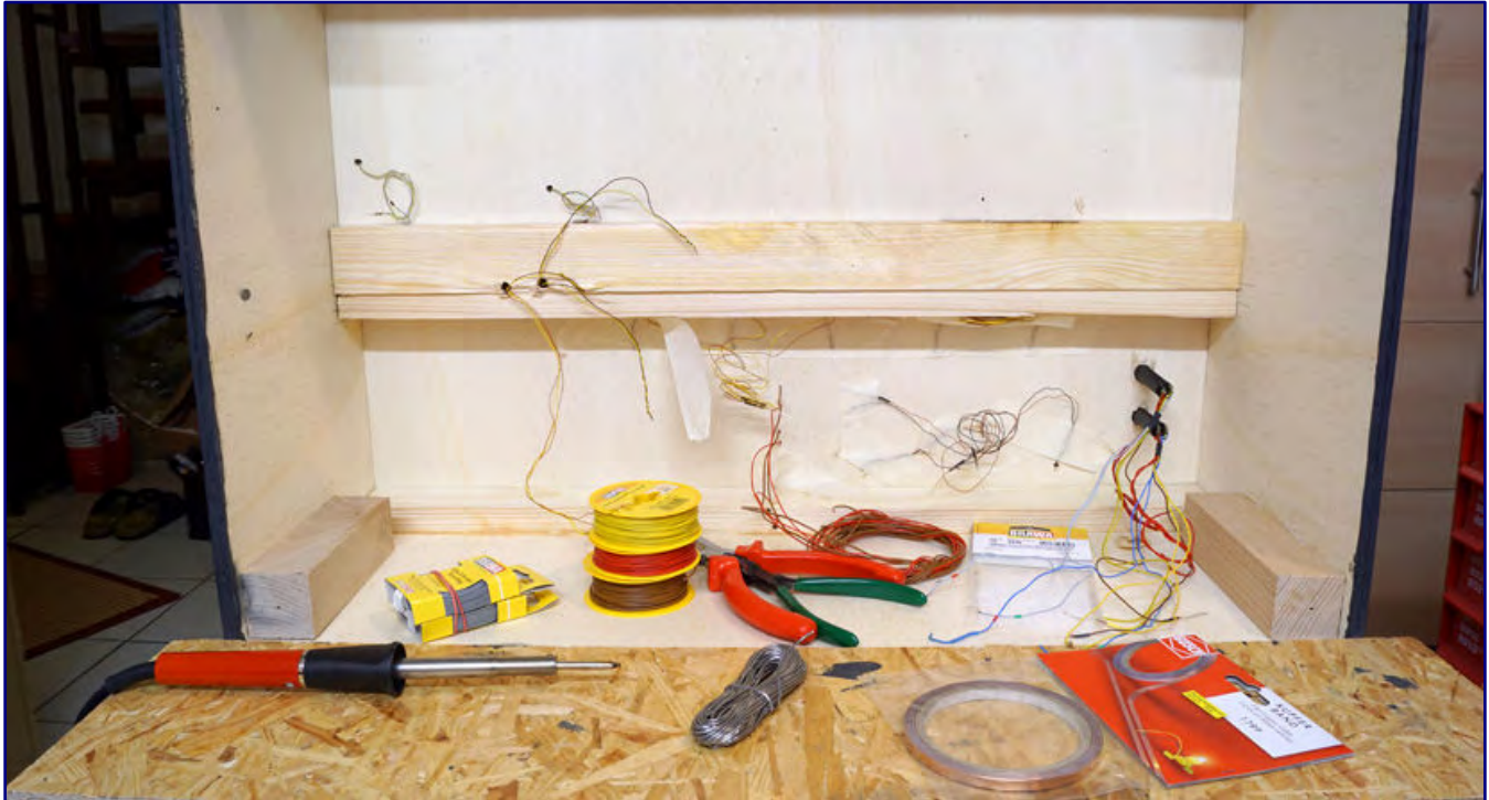
Starting on the wiring of the diorama: The wiring follows Märklin's colour coding scheme for Z scale electrics (see information box) are sourced from Brawa, as are the cable holders. The adhesive copper tape is from Busch, which can conduct currents of up to 2 A, and is used for soldered connections.
