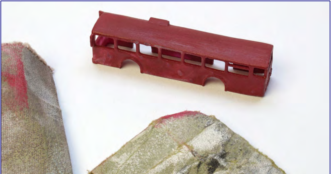
After the first coating, some unevenness and defects still come to light, which must be sandpapered before the next coating process.
