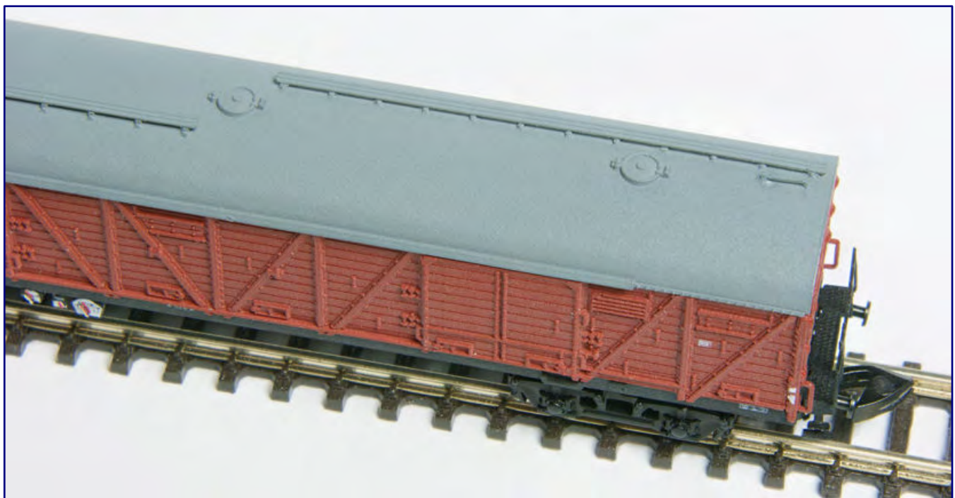
The three feed openings (two of them in the photo) for grain goods, which are closed with roof hatches and can be reached via gangways, are special features of this design and have been correctly reproduced by Zmodell. The grey handle on the right side of the roof should also be on the opposite side of the roof as in the model drawing.
