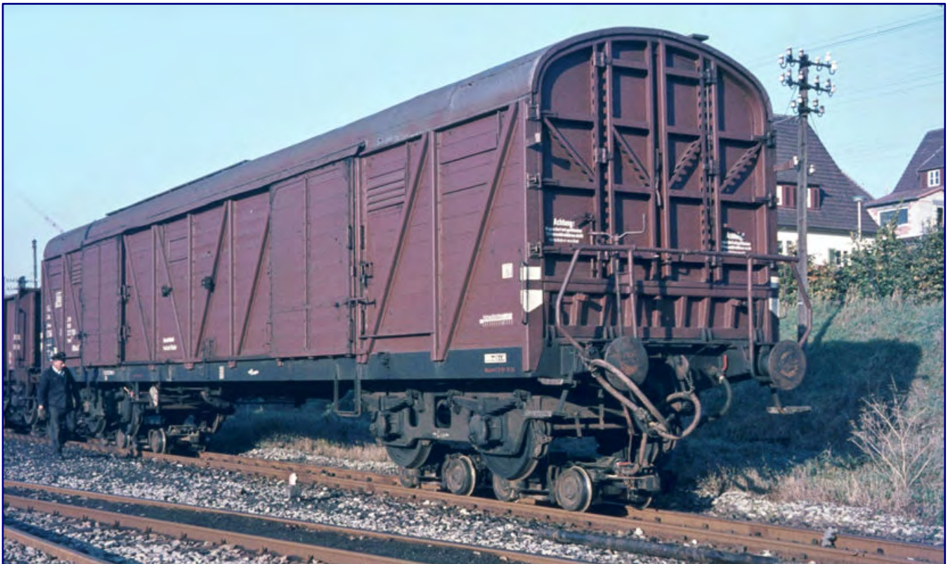
On 11 October 1967, a Harcs 340 is shunted standing on four trestles in Marbach station of the Bottwartalbahn. It is from the later deliveries, because the upper part of the gullwing doors is only diagonally stiffened. Like the car in the previous photo, however, it has long since lost its unloading doors for grain. Photo: Dieter Junker, Eisenbahnstiftung
