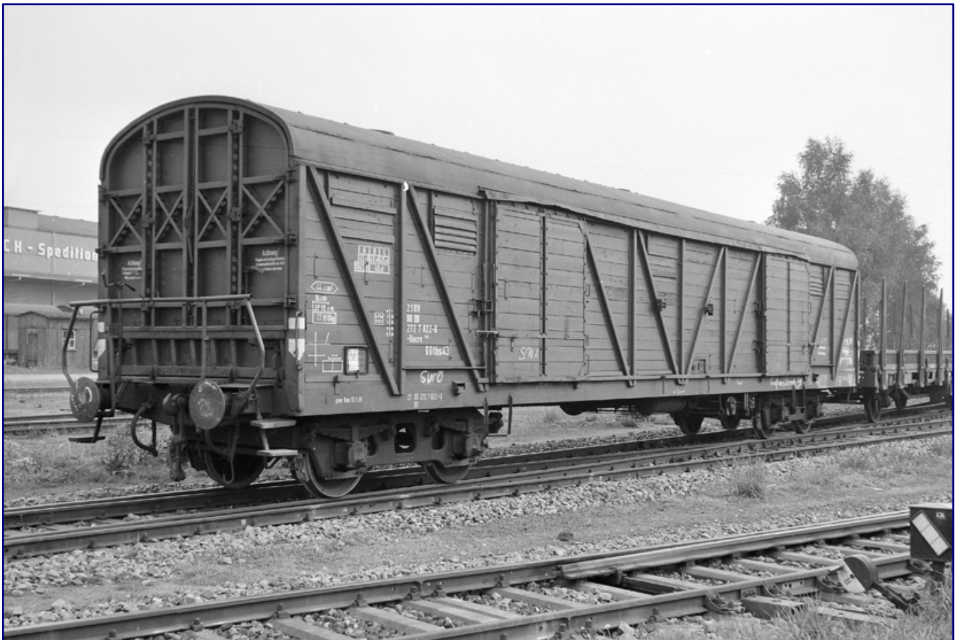
At Offenburg station the Hacrs 340 (ex GGths 43) with the road number 21 80 272 7 022-0 in May 1967 reveals that it originates from the early deliveries of its type: Its four-wing end wall doors are stiffened crosswise in the upper part. Photo: Reinhard Todt, Eisenbahnstiftung
