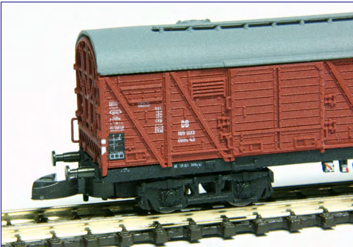
Buffers, axles, bogies and close couplers were made by Märklin, which forced smaller compromises that could not be noted without measurements. The lettering is very fine, but should have been a little bit darker and more opaque. On both photos you can see the missing roof handle at the end of the car without brakes.
