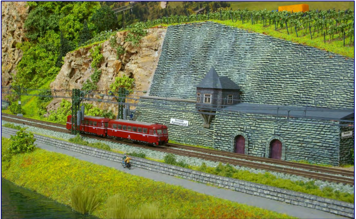
The two-part railbus focuses the observer's gaze on the self-built overhead line with double cantilevers and wheel tensioners on the masts.
