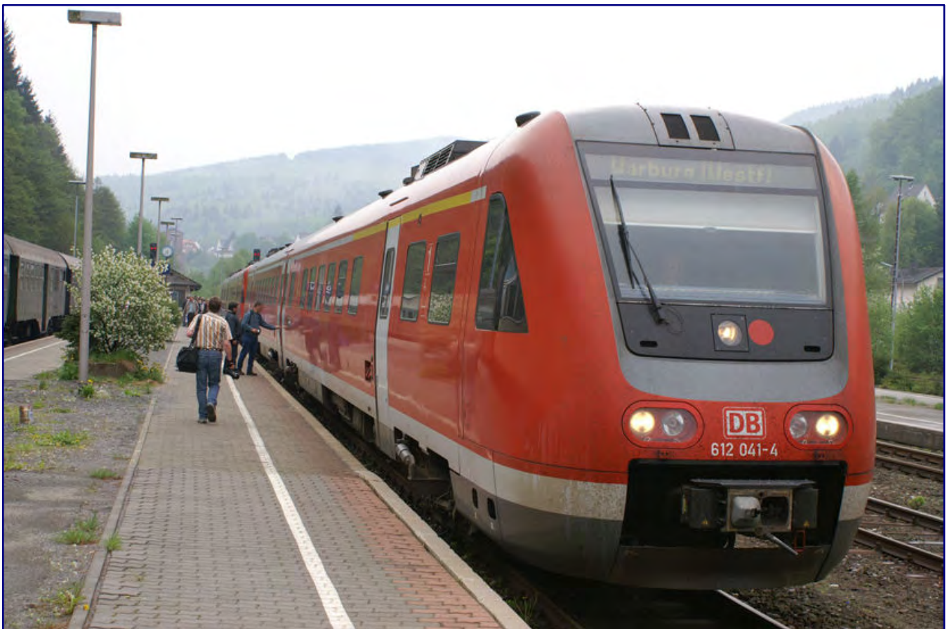
The original plan to speed up traffic by upgrading the Obere Ruhrtalbahn (Upper Ruhr Valley Railway) for tilting trains was reflected in the use of the class 612 "Regio-Swinger". Here, 612 041-4 is waiting to continue its journey to Warburg on 13 May 2006 in Brilon Wald.
