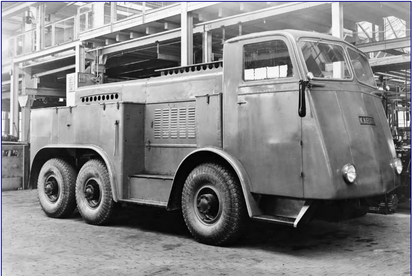
The type Z 6 R 3A from Kaelble was the heaviest and with 180 hp the most powerful tractor of its time, here probably brand-new taken on 11th November 1937. By adding extra ballast the vehicle could increase its total weight from 14.5 t to 21 t, which together with the four-wheel drive provided an impressive traction. In order to be able to carry this vehicle weight, special Fulda balloon tyres of size 13.50-20 were required. Photo: RVM, Archiv Eisenbahnstiftung
