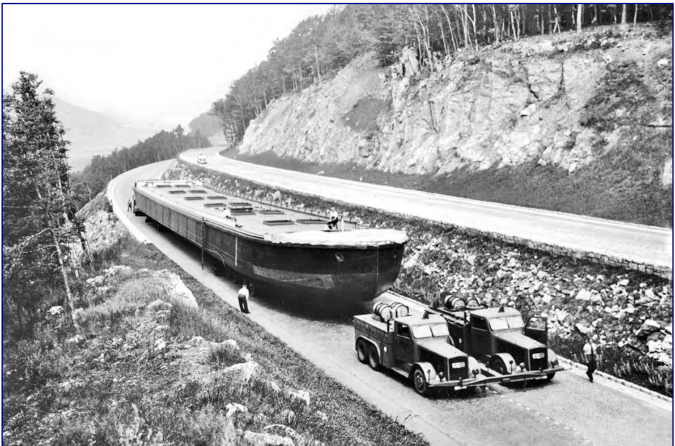
The heavy scooters, which travelled at a maximum speed of 8 km/h and thus barely faster than walking speed, gave the accompanying photographer many opportunities to take photos. Here, such a unit with a ship's hull circles the Kindinger Berg on the Reichsautobahn (autobahn) on 29 May 1940. Photo: RVM, Archiv Eisenbahnstiftung
