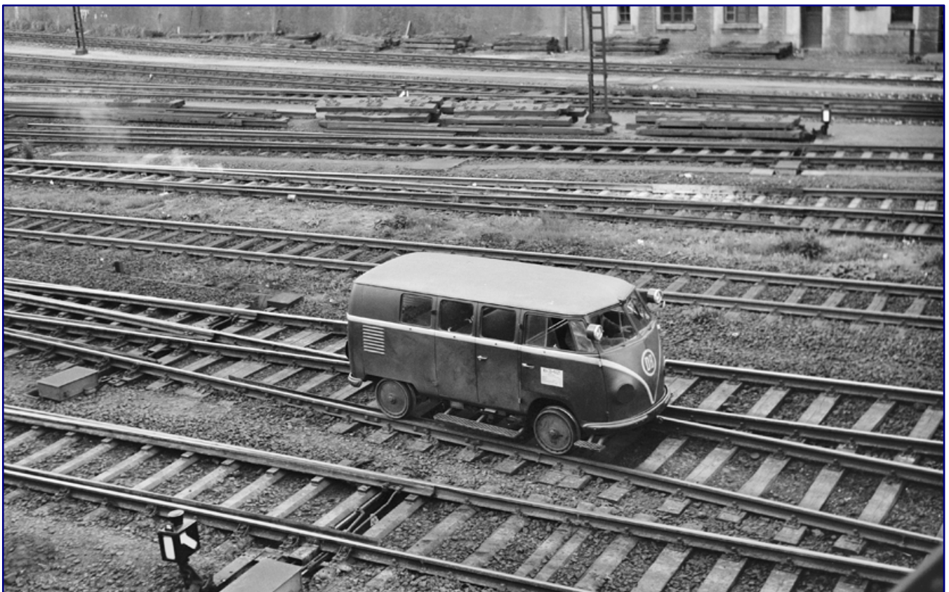
The railway master of Minden went on an inspection trip on 18 May 1961: After all, the Klv 20, based on the VW Transporter, was capable of speeds of up to 70 km/h, here the vehicle with the number 5021. It was braked by a foot pedal brake which acted hydraulically on all four wheels. Photo: Joachim Claus, Eisenbahnstiftung
