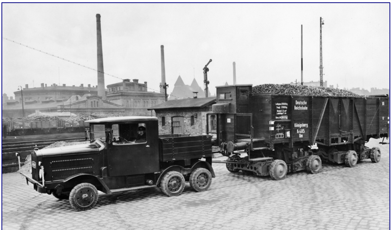
On 27 April 1933 the Reichsbahn in Berlin-Anhalter Gbf carried out test runs with the first Culemeyer team. The tractor is a Kaelble Z 6 R with 100 HP power. Only three tractors of this type were delivered to the Reichsbahn. Photo: RVM, Archiv Eisenbahnstiftung
