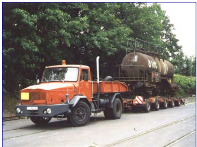
The Hagedorn plastics factory in Lingen (Ems) received tank wagons for road transport. The road transporter Faun F 610/36 Z (former DB 47-682) photographed in the photo on 11 September 2001 was used on its own responsibility, until 2005. Photo: Stefan Kunzmann (Public Domain)
