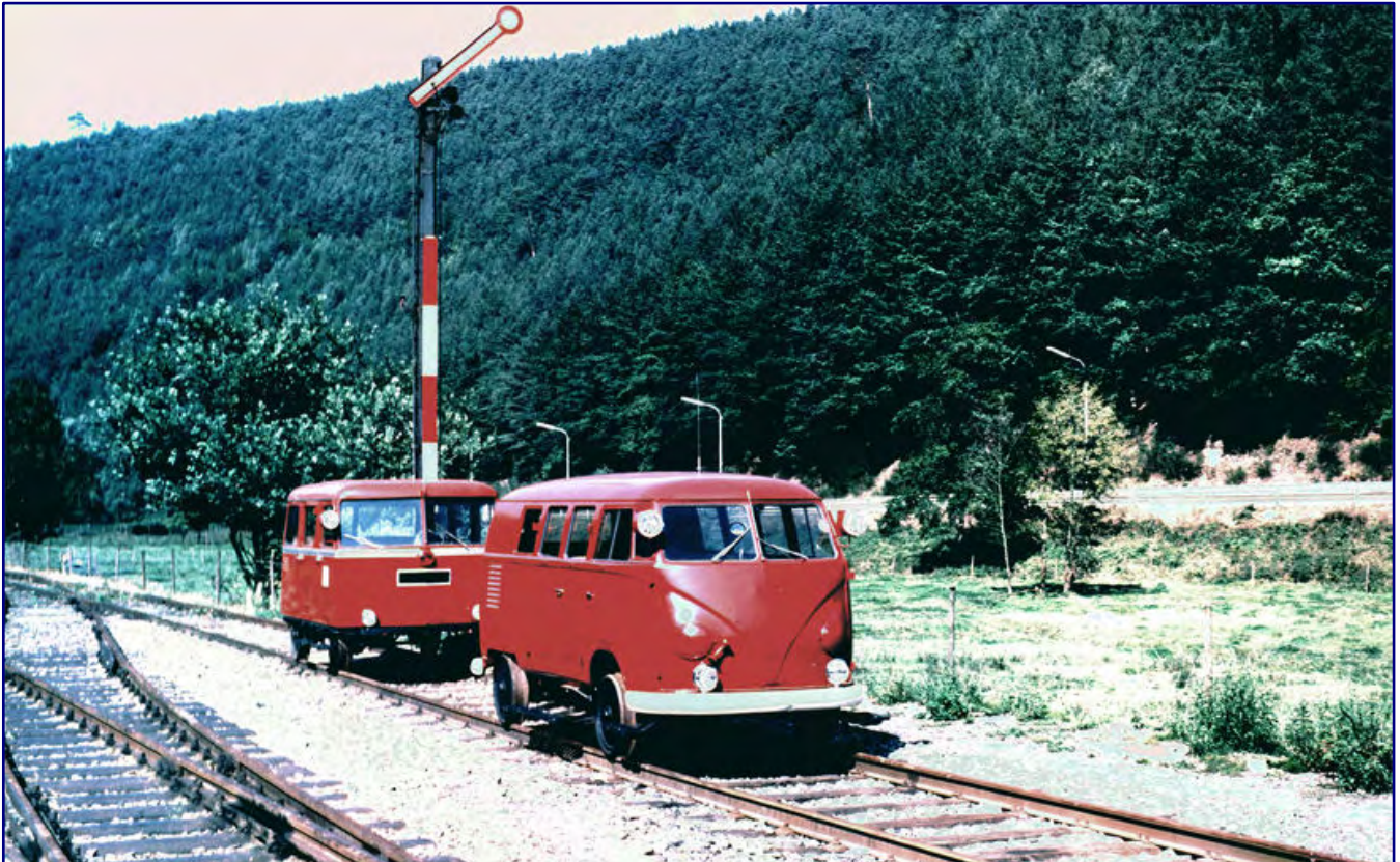
To save development costs, the Klv 20 was derived from a road vehicle. However, it was by no means the only railway master hand car in the service of the DB. On 17th September 1978 two types of construction were presented to the public in Elmstein, among them Klv 20-5011. Photo: Manfred Britz
