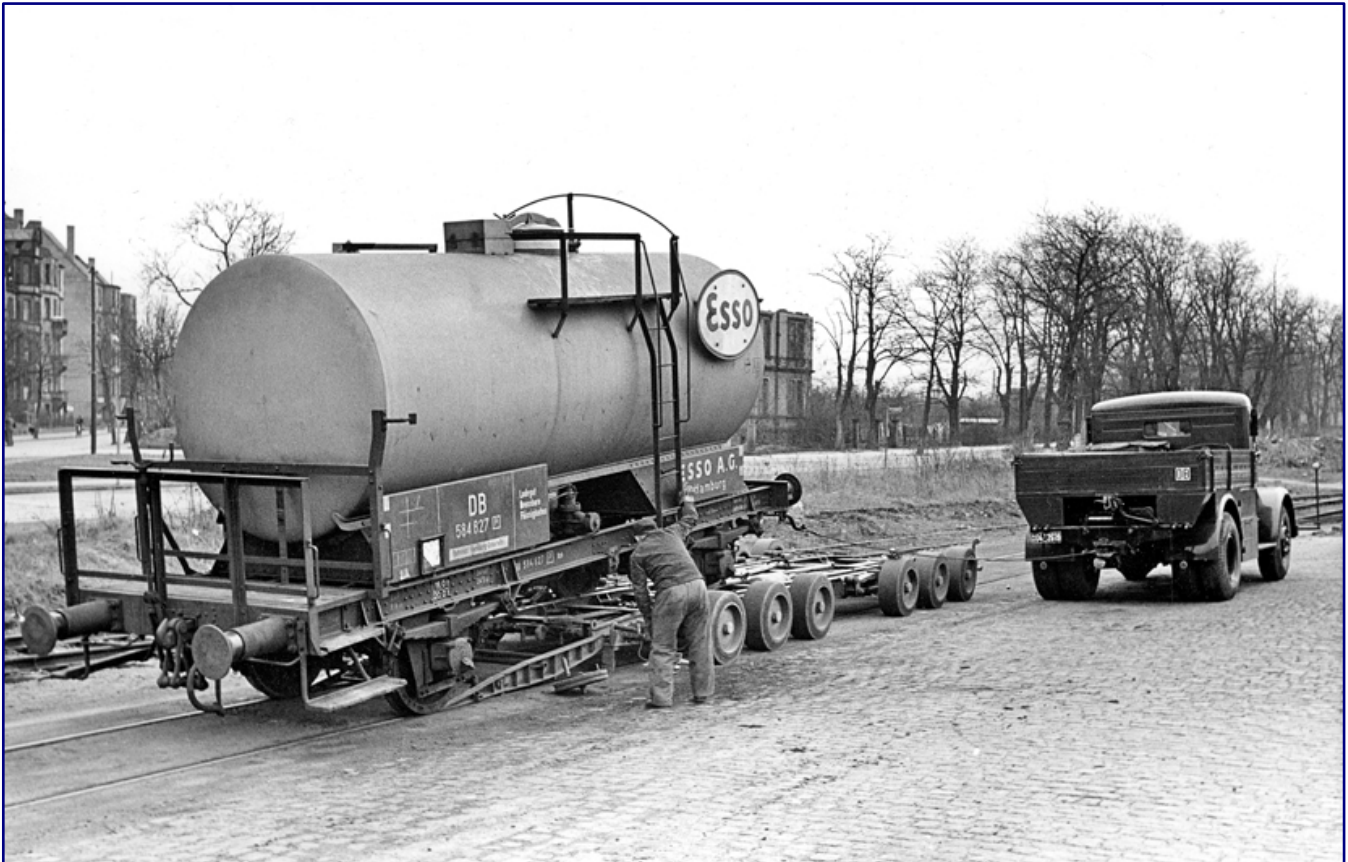
After 1945, the Culemeyer transports initially played an important role in the reconstruction and subsequent economic miracles. Photo taken at Hanau railway station in 1956 shows how the Kaelble tractor uses a cable winch and ramp to pick up a tank car from the German Esso AG onto its six-axle road scooter. Photo: Paul Trost, Archiv Eisenbahnstiftung
