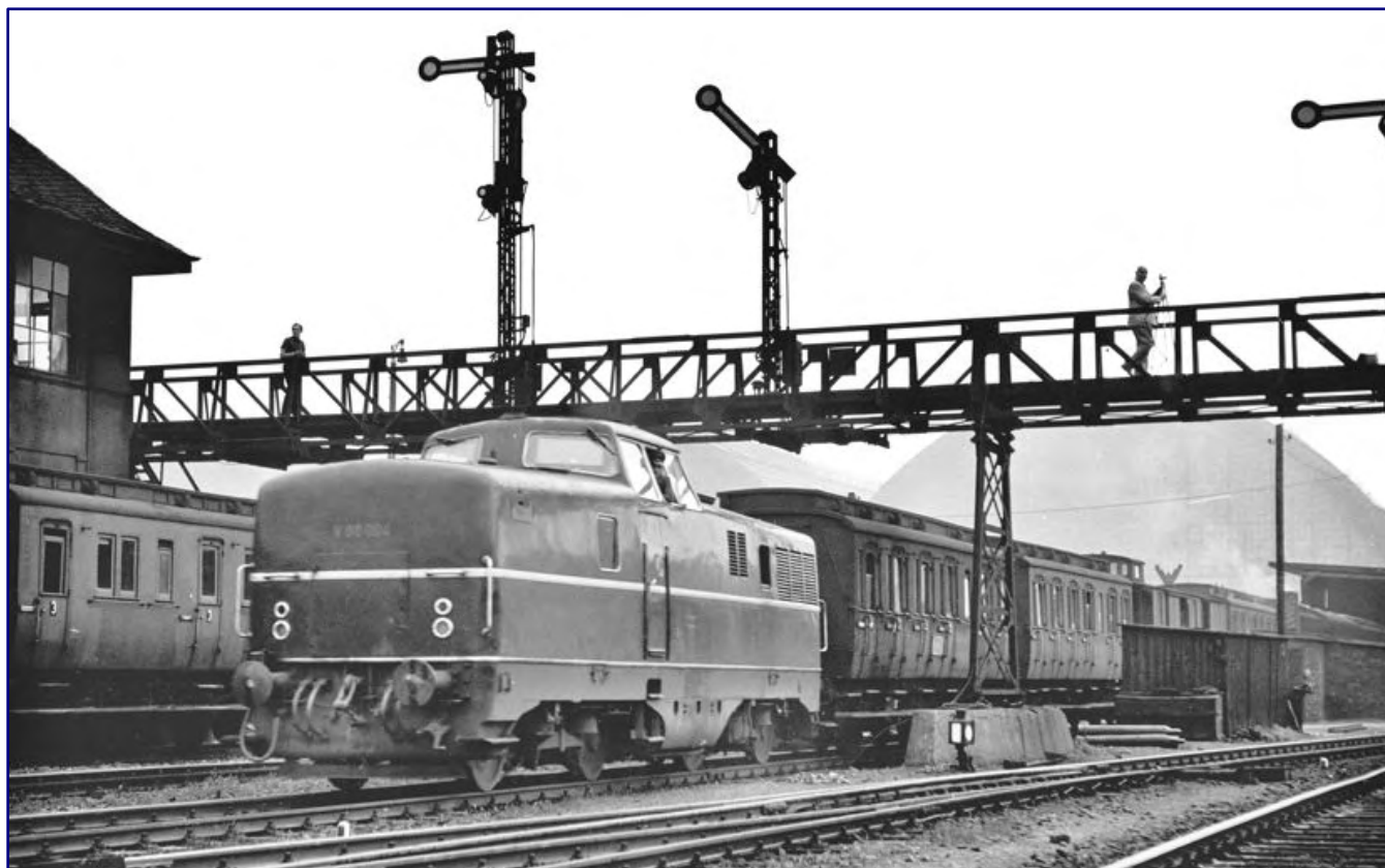
V 80 004 from the Frankfurt-Griesheim depot pushes its passenger train of blunderbusses between the Galluswarte branch and Frankfurt-West in 1954 without a doubt under indirect push-pull control, as can be seen from the direction of view of the driver remaining on the locomotive (photo above). The same locomotive still had to make do with Prussian compartment coaches when it left Frankfurt's main station in October 1952 (photo below). The three-light tip signal was not yet mandatory at that time. Photos: Reinhold Palm, Eisenbahnstiftung
