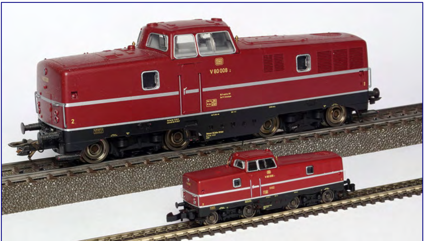
V 80 008 is in no way inferior to its larger sister in 1:87 scale (36082): The differences are almost limited to the more indicated driver's cab interior in the larger scale, the different system couplings and wheel flange heights.
