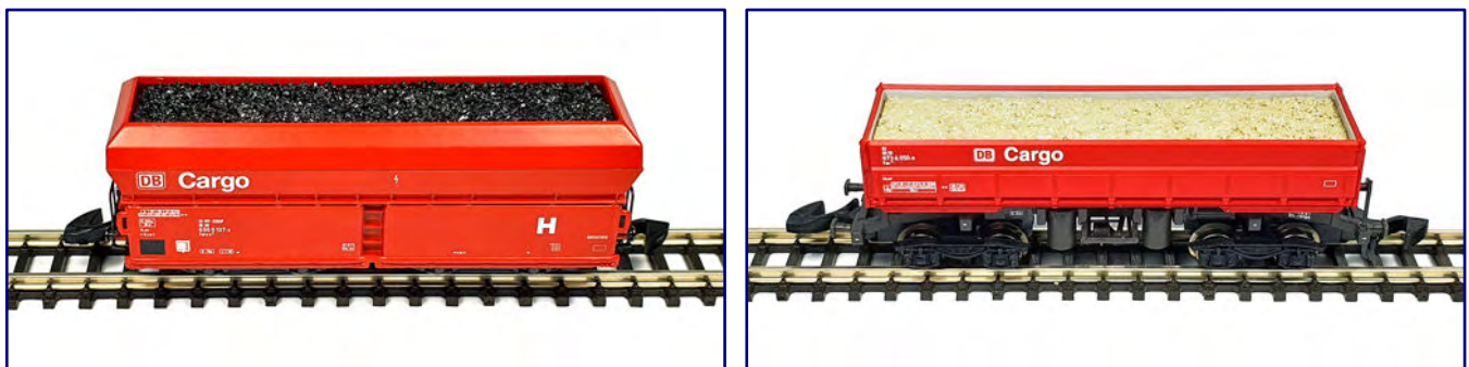
Märklin models for which loads are offered include the Fals loaded with coal (-001) here (photo left) and the Eamos filled with limestones (-010), in our examples (photo right). Photos: Zmodell
