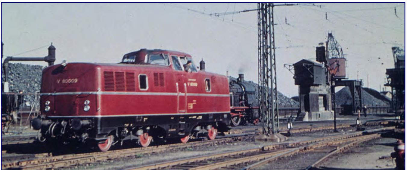
When the V 80 first saw the light of day, the steam locomotive still dominated everyday life, here in Nuremberg in April 1956, as V 80 009 passes through the scene. The only provisionally mounted, upper top light is interesting. Photo: Sammlung Peter Pfister
