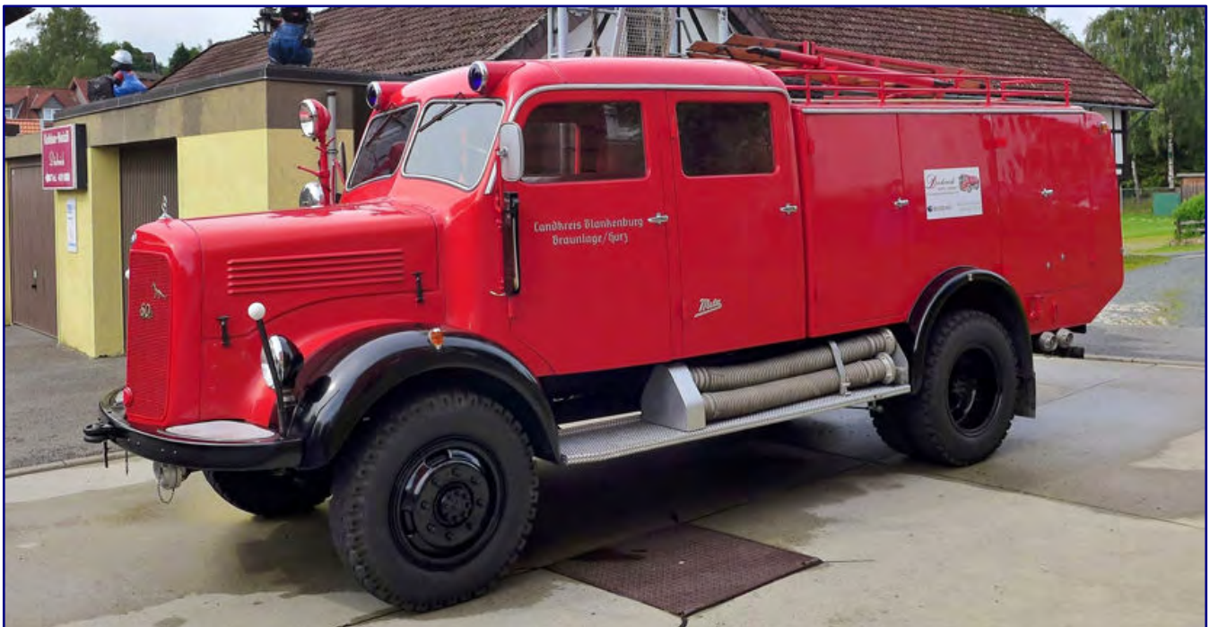
This four-wheel drive Mercedes-Benz LAF 3500 with Metz body from Braunlage / Harz (Lower Saxony) probably dates from the first year of construction in 1950. This is indicated by the blue warning lights, which are only directed forwards, and above all by the split windscreen, which was no longer common for this type of vehicle. Photo: Bahnfreund (CC-BY-SA-4.0)
