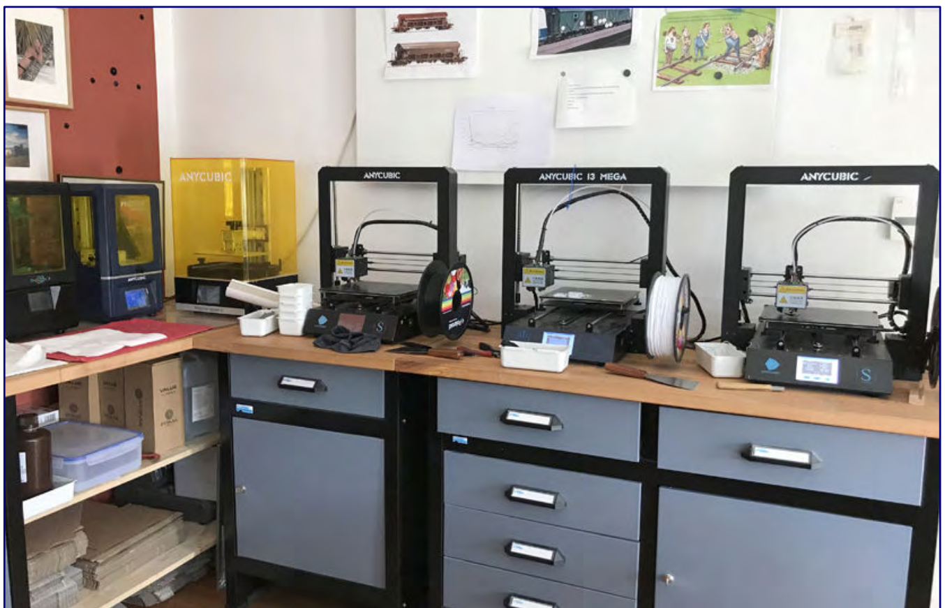
A look at the six 3D printers that work for NoBa-Modelle today: Depending on the demands of the project, printing is done in PLA and SLA processes.
