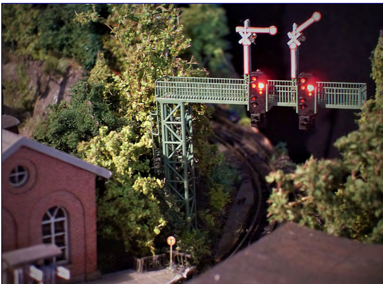
The fine and contemporary catenary wires for the Märklin system geometry (photo above) belong to the more recent designs of the small series manufacturer. A preview of the ongoing developments is offered by the signal cantilever with two colour light exit signals and wing signals marked as invalid (photo below). Photo (below): Henry Christophori
