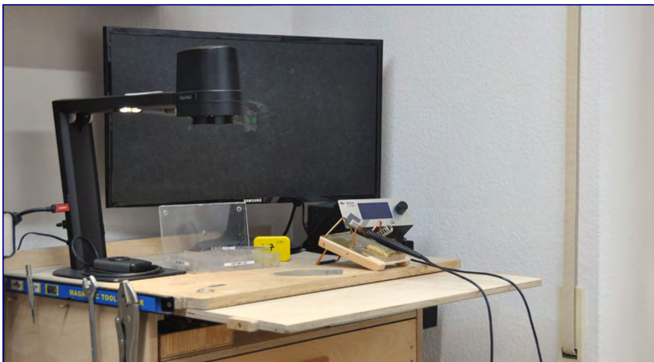
Heinz O. Schramm at milling work for his models (picture above), to his left you can also see his milling station. He is particularly proud of his camera soldering station (photo below) for the smallest parts, which allows 48x magnification. Photos: HOS Modellbahntechnik
