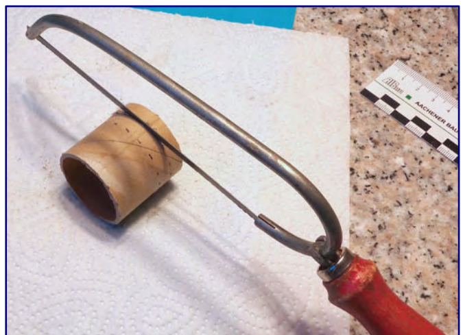
A cardboard roll with an inner diameter of 3.5 cm was used as the basis for building arches (left). The precise use of a handsaw produced cleanly cut circular segments (photo right).
