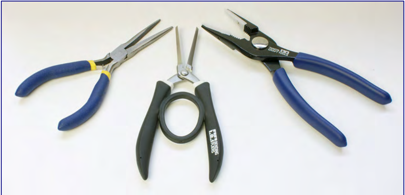
The mini needle-nose pliers from Revell (art. no. 39079; left), the moulding pliers for photo-etched parts (300074067; centre) and the needle-nose pliers with scratch protection (300074065; right), the latter two from Tamiya, are presented to you as valuable tools for model building.
