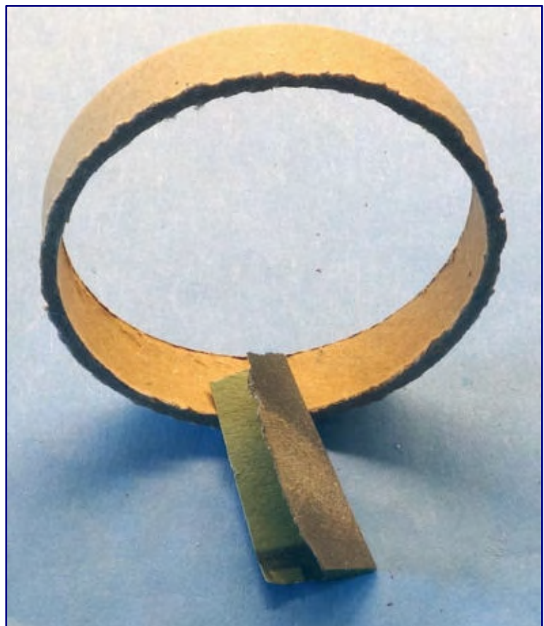
Rough edges that occur during sawing can be removed and smoothed with sandpaper.
