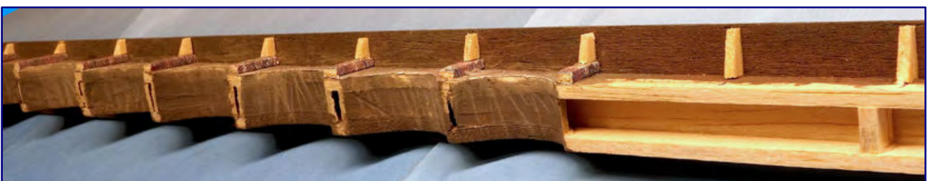
The cantilevers are glued on as shown here, but only on the side that will later face the viewer. The other side remains without these cantilever arms.
