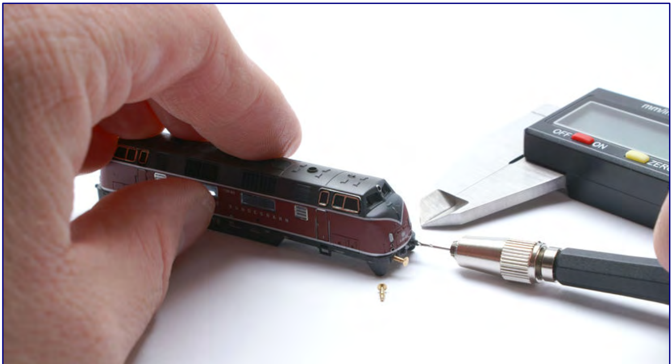
The standard buffers were exchanged for turned parts from FR Freudenreich Feinwerktechnik, the apron on driver's cab side 2 was furthermore closed with a polystyrene profile.
