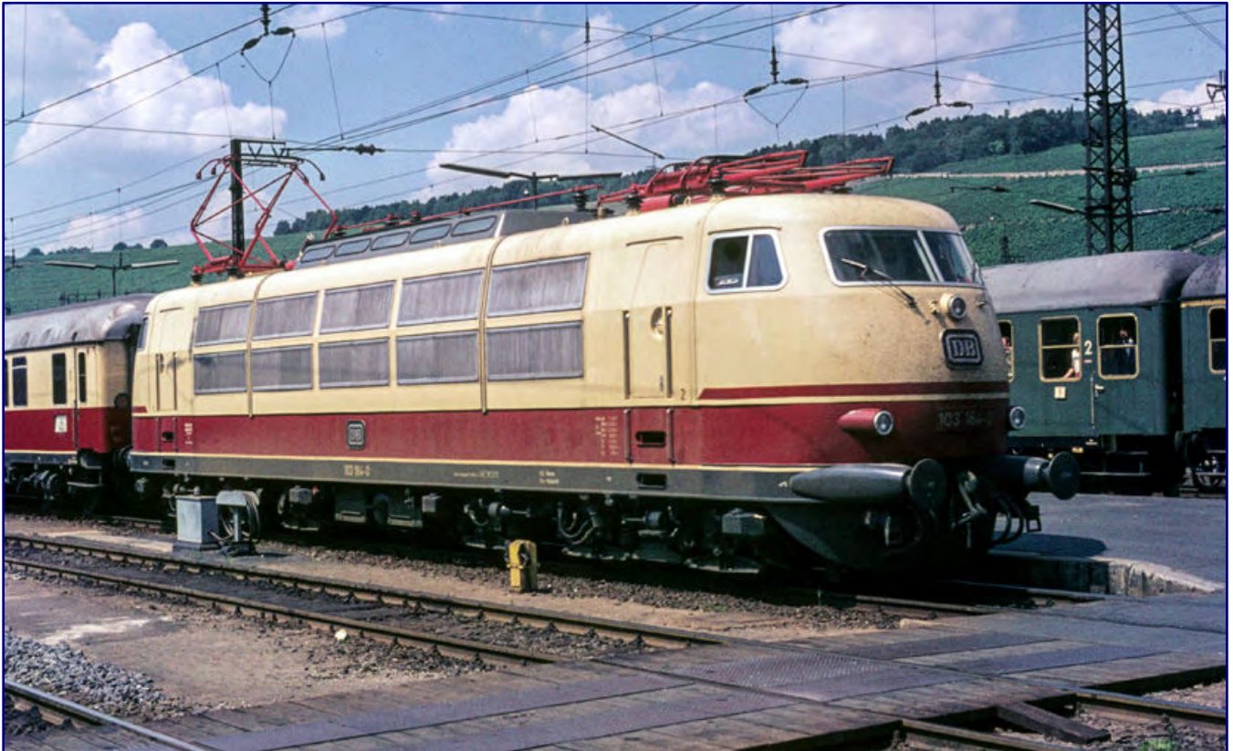
Whatever changes were to take place in the IC concept, the class 103 remained the pillar of this system for thirty years. When 103 164-0 was photographed in Würzburg Hbf, it still wore its front apron and also the DBS 54 scissor pantographs with Wanisch rocker. Photo: Archiv Petkelis
