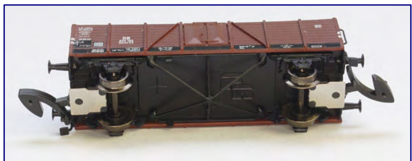
View of the wagon floor made of etched metal sheets with the spatial framework structure.
