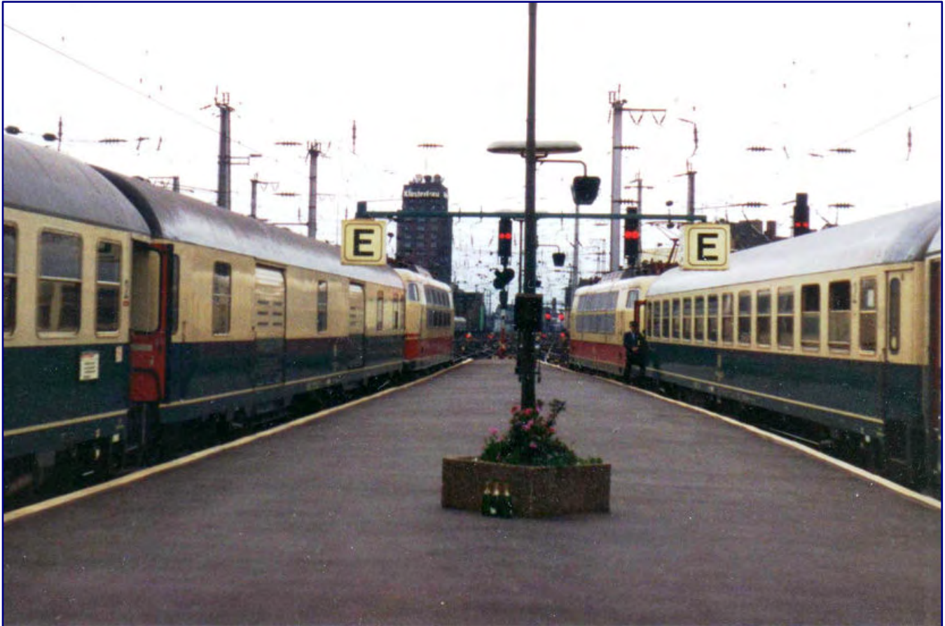
This photo from Cologne Central Station, taken in 1980, illustrates the principle of trains stopping at the same time on the same platform for quick transfers. The newly introduced platform sections, in the photo you can see the signs with the marking E, also belong to the IC '79. The IC 625 "Meistersinger" stopping on the left is one of the few Intercity trains to carry a baggage car. Photo: KlausMiniwolf (CC-BY-SA-4.0)
