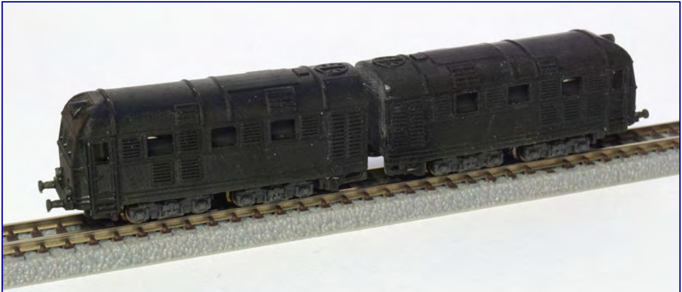
Test sitting on the chassis: To build up a V 188 from the two resin bodies from NoBa-Modelle, only two shorty chassis from Rokuhan are additionally required. The superstructures are simply attached.
