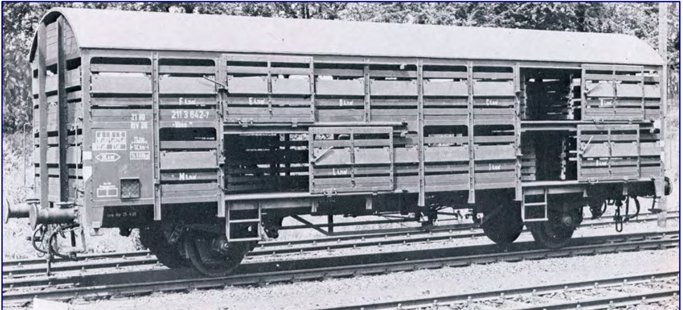
From 1968 onwards, the remaining livestock wagons that had not been converted into covered wagons of the standard design were designated as Hbes 358. The photo clearly shows the revolving doors for separating the individual crates. Photo: Werbeamt der Deutschen Bundesbahn, Slg. Trainini
