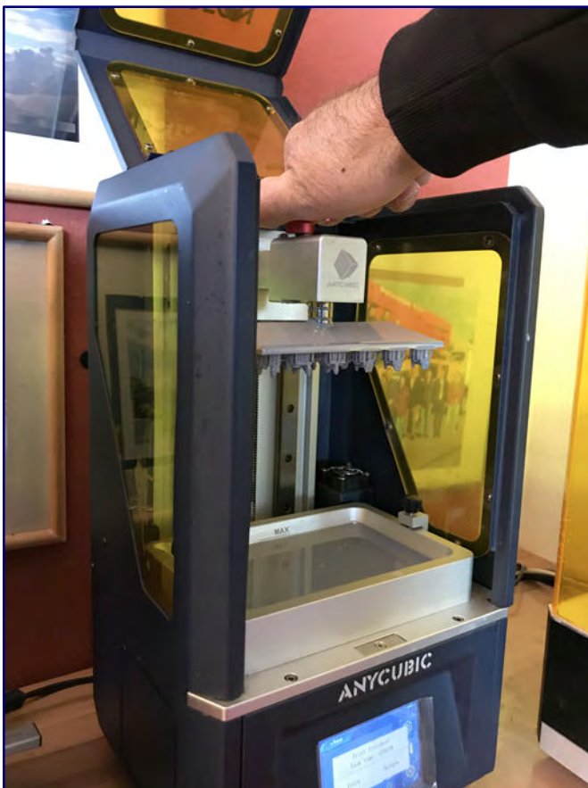
The printing is finished (photo on the left), the models reveal themselves after removal from the printing plate (photo on the right) and await further processing.
