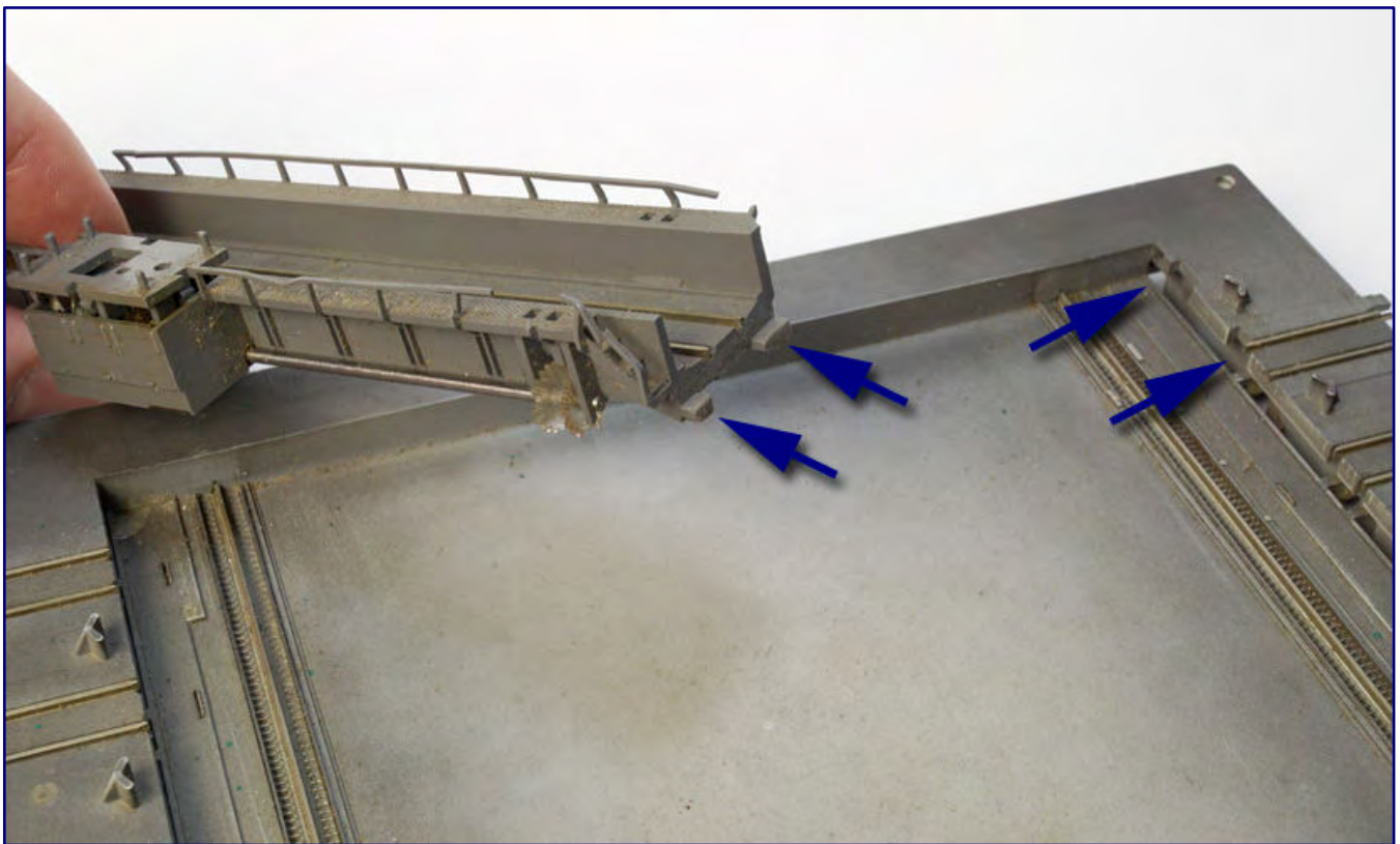
The arrows in the photo indicate the guide lugs on the platform (left) and the corresponding recesses at one end of the pit (right), recognisable by the lack of a track exit there, which enable removal by tilting.
