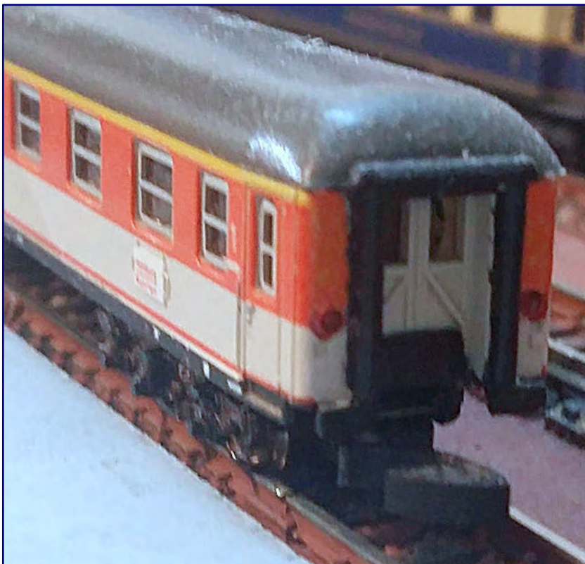
Early versions of Z scale passenger carriages can be significantly improved by painting the upper colour strip around the corner and by also painting the transition plates, tail lights and rubber beads.
