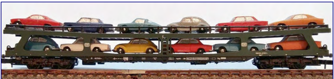
Two examples of DDm car transport wagons that can run on long-distance trains: up to twelve vehicles can be loaded on both floors of this double-decker wagon.
