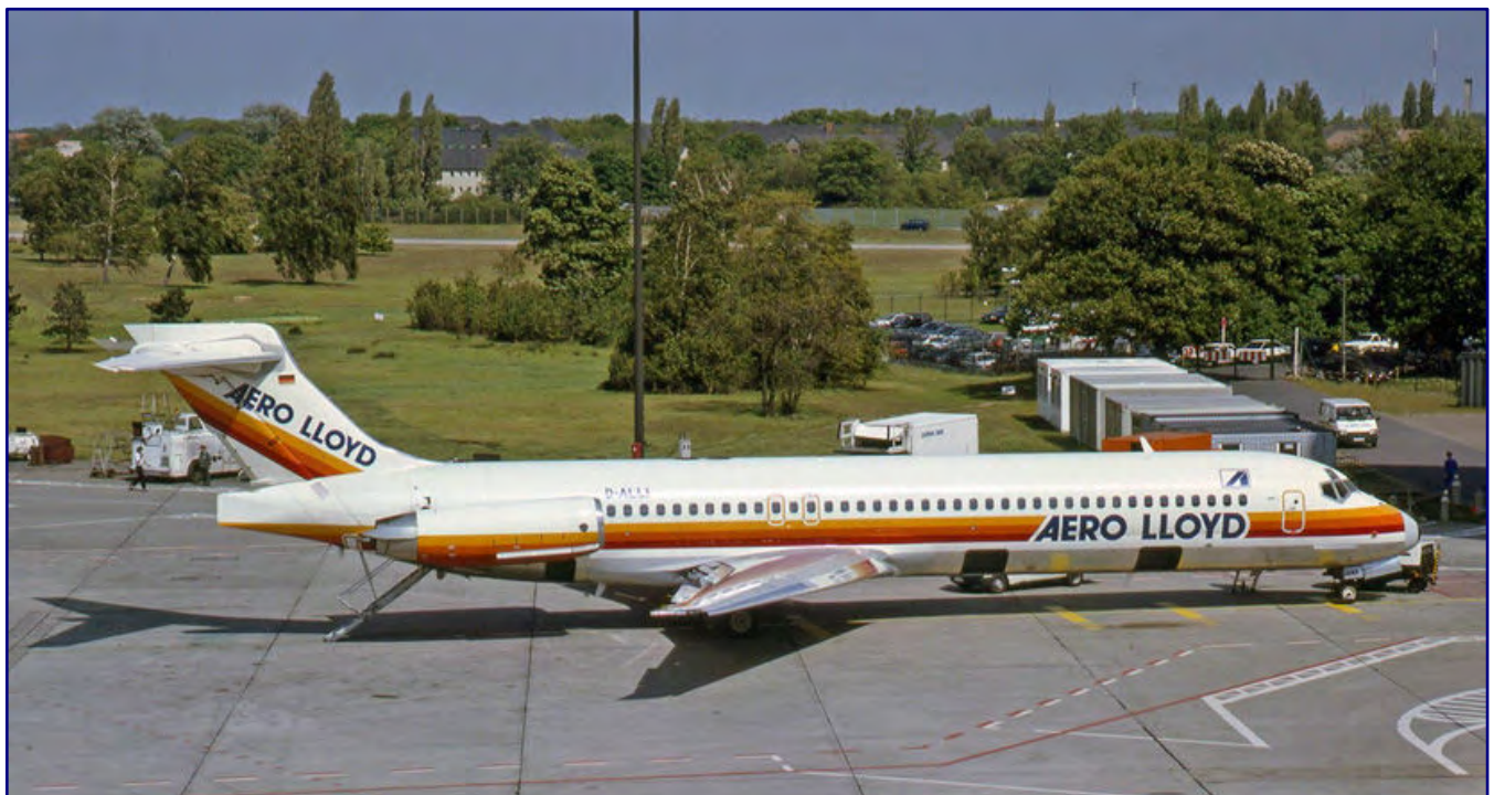
The McDonnell Douglas MD-87 (officially: DC-9-87) also flew at Aero Lloyd, and was a further development of the basic version. Photo: Ralf Manteufel (GFDL-1.2)
