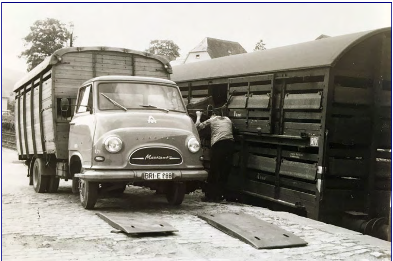
In the sixties, cattle transport is still a lucrative business for the Bundesbahn. In Brilon, Sauerland, small cattle are loaded from the Hanomag lorry into the upper deck of a still almost new Vlms 63 using a ramp. Photo: Gerhard Tüllmann, Brilon
