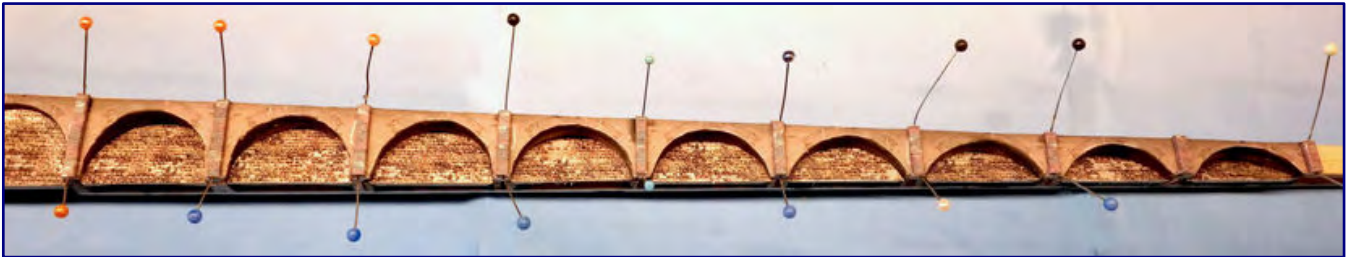
Until the adhesive sets, the pillars are fixed to the arcade base with the help of pins.
