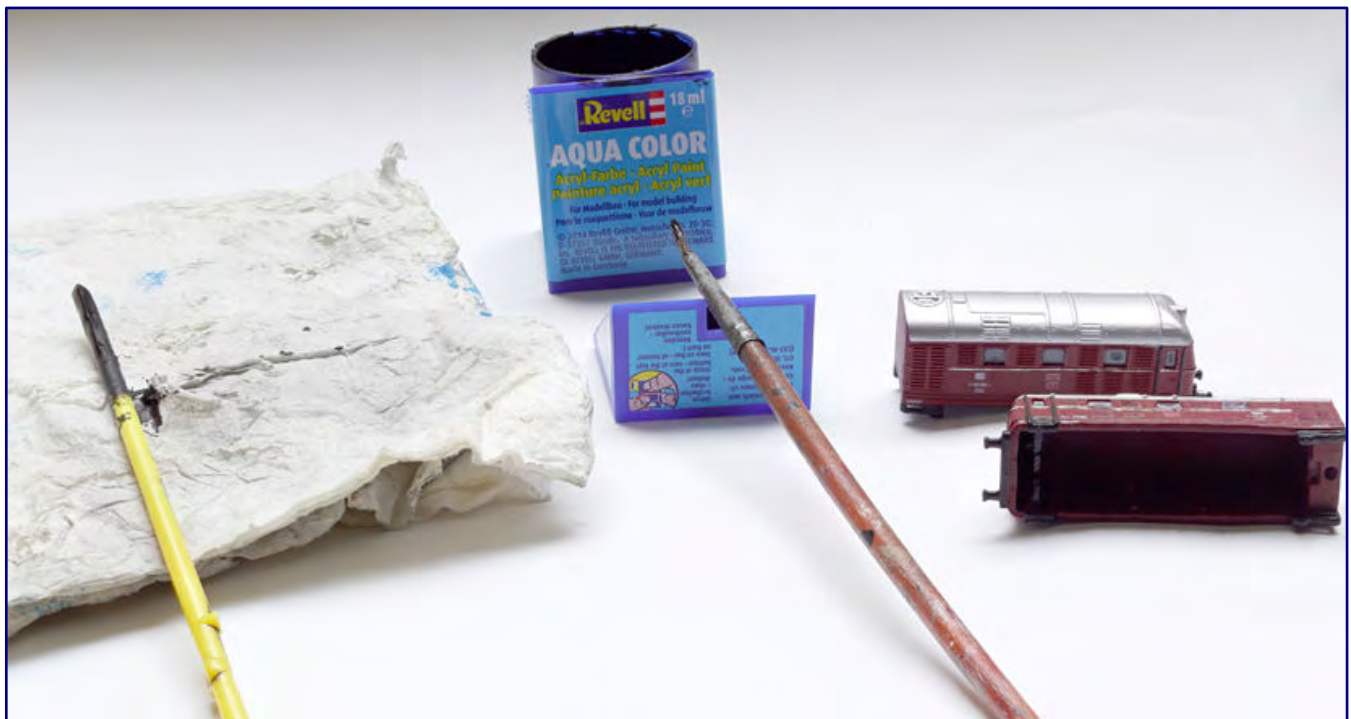
After the Micro Kristal Klear from Microscale has dried, all window surfaces are coated black on the inside with Revell lacquer to prevent unwanted light leaks or a view of the Shorty chassis block.
