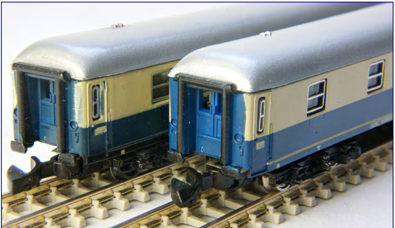
These two cars with item number 8722 from two editions illustrate the aim of the modification: On the older specimen (left) the coupler has a smooth upper edge and can catch on the buffer of a coupled wagon. The coupler of the newer specimen (right) already has a bevelled surface that prevents this and which oneself can easily modify. Optical deficiencies on the front sides of the cars are also clearly visible, as the printing has not been applied around the corners.
