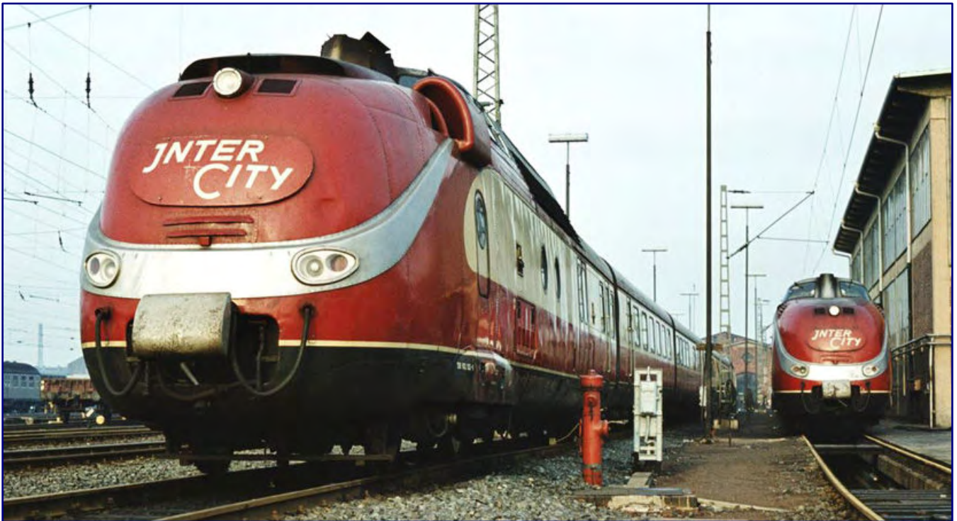
On four class 601 machine cars, the traction diesel engines were replaced by AVCO-Lycoming gas turbines (type TF35) with 2,200 hp output. The vehicles were easily recognisable by the significantly enlarged air intakes, as illustrated by the comparison of 602 002-8 with the regular version (right) on 30 November 1975. Photo: Prof. Dr. Willi Hager, Eisenbahnstiftung
