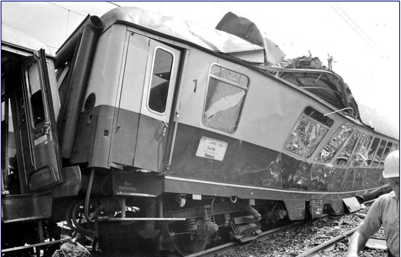
The rescuers must have seen a picture of horror, as this photo from the press conference on the day of the accident (12 August 1965) proves. According to subsequent investigations, TEE 77 "Helvetia" was travelling at around 120 km/h on the Riedbahn. The locomotive driver recognised the danger of the goods train, which was not free of profiles, and initiated an emergency braking manoeuvre. However, this was no longer able to prevent the collision at 11:35 am. Photo: Werner Kortokraks, Eisenbahnstiftung
