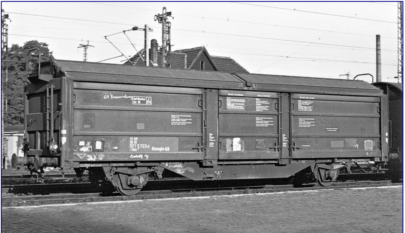
Tbis 871 with the car number 21 80 571 5 723-0 in weathered condition and with some first repair patches in in the city of Bebra. It is interesting that this car still carries its old designation Klmmgks 68. Comparing the photo with the one on page 6, the design changes on the sliding doors are obvious. Photo: Joachim Claus, Archiv Eisenbahnstiftung
