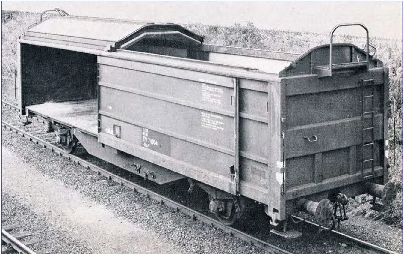
With this photo of a Tbis 870, Deutsche Bahn demonstrated to its customers the wagon's high flexibility for loading and unloading. Half of the roof area and, in this design, also half of the side wall were accessible at the same time. The photo also shows the transverse beam for reinforcing the superstructure and the catch hooks for the sliding roof at the end of the roof. Photo: Werbeamt der Deutschen Bundesbahn, Sammlung Trainini
