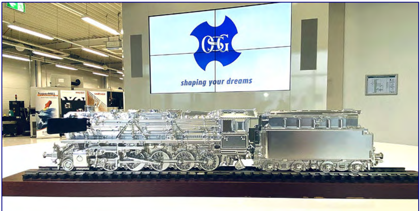
Milled from a cast block, this H0 gauge model of the 44 1315, museum locomotive is displayed in front of the new Märklineum. Photo: OSG Germany
