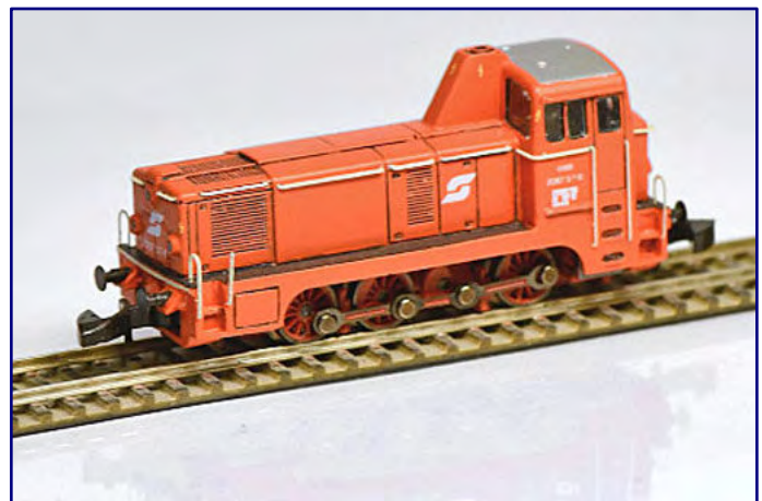
In Jaffa colours, the three-axle rod diesel locomotive 2067.57 will appear for shunting service. Photo: Sondermodelle Z
