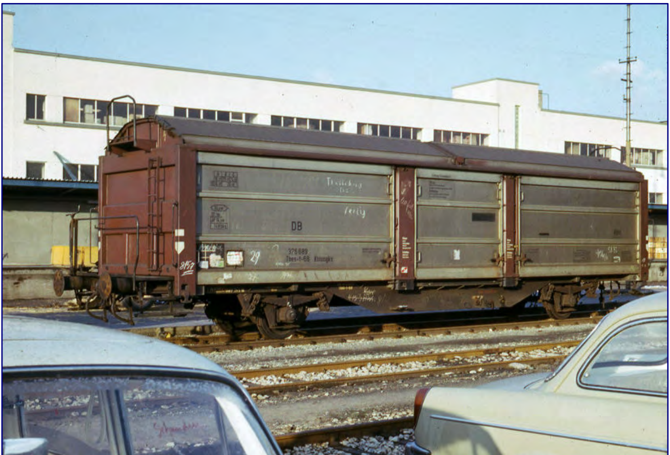
A perfect photograph of a Tbes-t-68 / Kimmgks of the German Federal Railways; here, the specimen with car number 376 889. This wagon belongs to the variant equipped with handbrake, and is 500 mm longer than the prototype behind Märklin's model. Nevertheless, it still serves as a valid basis for assessing the model. Photo: Fritz Willke, © Stefan Carstens
