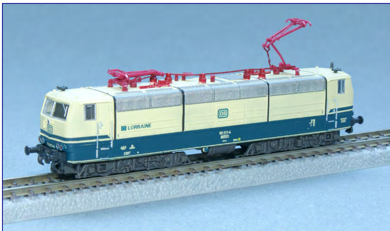
The class 103 (8854; top) was the first electric locomotive in the Mini-Club programme from 1974, initially still with clamped instead of bolted pantographs, as seen here. In 2015, Rokuhan demonstrated with its class 181 2 (T950-1; bottom) what true-to-scale pantographs that lay flat on the roof should look like.
