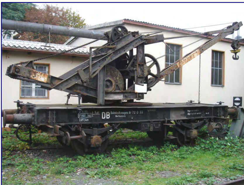
This hand-operated rail crane from 1901, last used as railway station car 72 033 at the Bamberg depot, was a reminder of the early beginnings of this type of car for the DB Museum in Nürnberg (Nuremberg) in September 2005.
