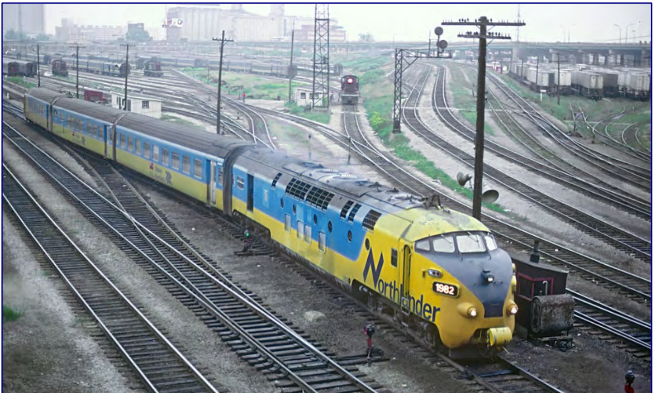
In September 1979, Ontario Northern 1982 is still in its original configuration, photographed in Toronto with the “Spadina Yard” marshalling yard and holding sidings in the background. A short time later, the failure-prone powerhead was to be replaced by an EMD F7P diesel locomotive. Photo: Marty Bernard (Collection Roger Puta)
