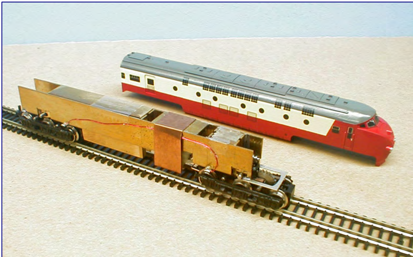
Chassis construction and power supply of the Märklin three-pole motor can be seen here from two different perspectives. The basic construction follows the previously built ALn 442 / 448 of the FS.
