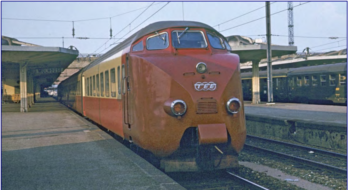
After the stop, the set shown on page 5 also allows a view of the driving trailer, which in addition to a large compartment also housed a recreation room for the on-board mechanic. Photo: Joachim Lutz (CC-BY-SA-4.0)
