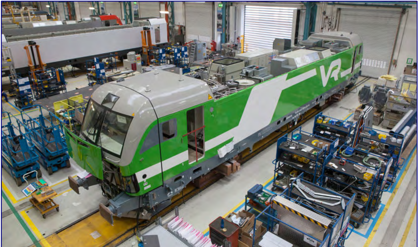
When this Vectron, destined for the Finnish state railway VR, is built in Munich-Allach, it allows a view into its interior with a firmly defined basic arrangement of the necessary components and aggregates. Photo: Siemens Mobility (Siemens-Pressfoto)
