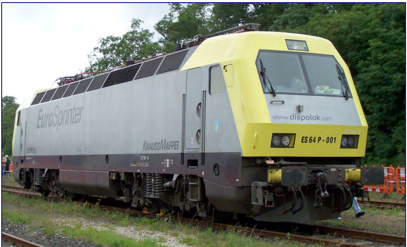
Siemens sent 127 001-6, the "EuroSprinter", into the race for a modern three-phase locomotive to succeed the class 120. Internally designated ES 64 P, the locomotive became the forefather of Siemens locomotives up to the Vectron platform. Photo: Urmelbeauftragter (CC-BY-SA-3.0,2.5,2.0,1.0)
