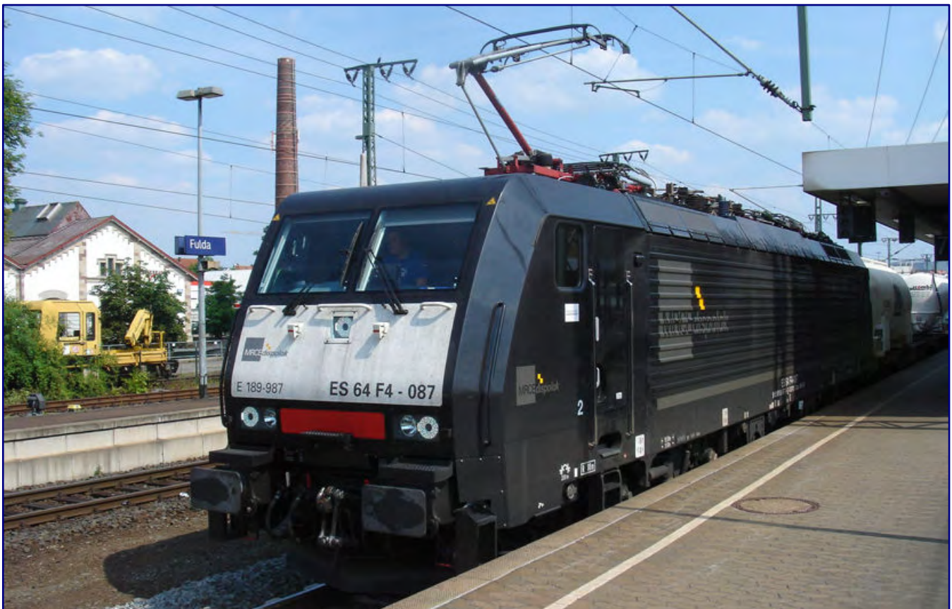
The Europrinter gave rise, among other things, to the class 189 as a multi-system locomotive for freight transport, internally designated ES 64 F4. It was also procured by Deutsche Bahn AG. However, this example taken in Fulda on 2 July 2010 is leased from MRCE.
