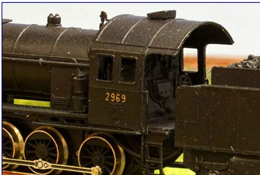
This photo shows not only the different coupling axle position by means of the third, fourth and fifth coupling wheel, but above all the driver's cab with interior equipment!
