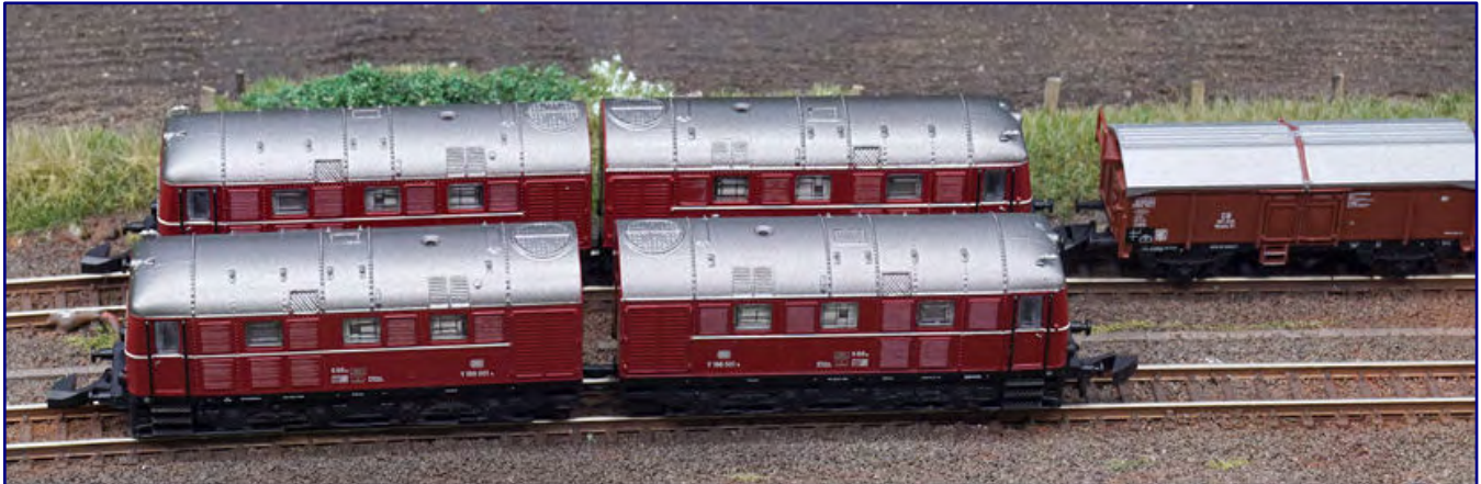
A direct comparison of two examples shows the different coupling positions when using the factory-mounted (bottom) and the short drawbar for the showcase and large radii (top).
