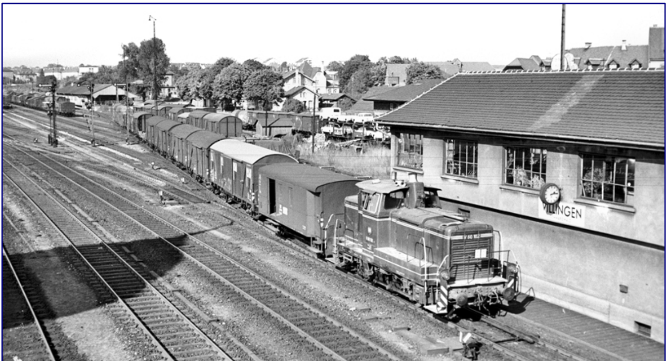
On 7 October 1962, V 60 102 was doing shunting work at Villingen station. Right behind her is one of the freight train luggage wagons Pwgs 41, which was built by Westwaggon Köln-Deutz with wartime simplifications, as also shown in the new Märklin model. Photo: Helmut Röth, Eisenbahnstiftung
