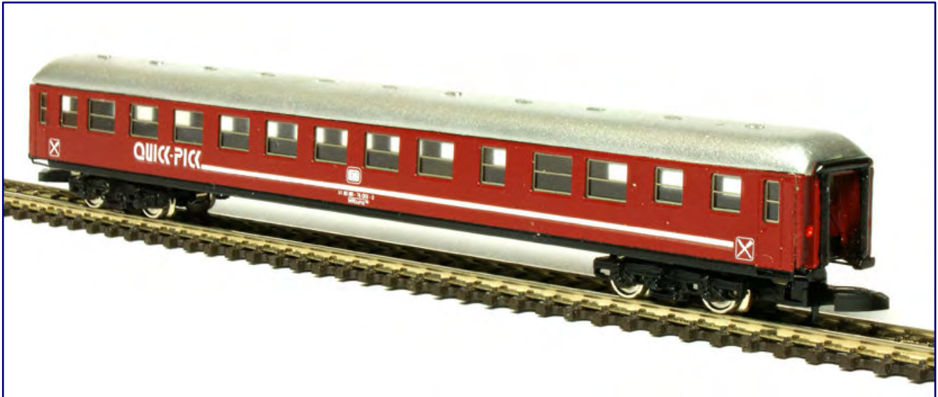
This DB self-service dining car WRbumz 138 from the Heckl Kleinserien programme was certainly unknown to many Zetties. The model, made with the help of etched sheets, exactly reproduces window sizes and arrangement on both sides.
