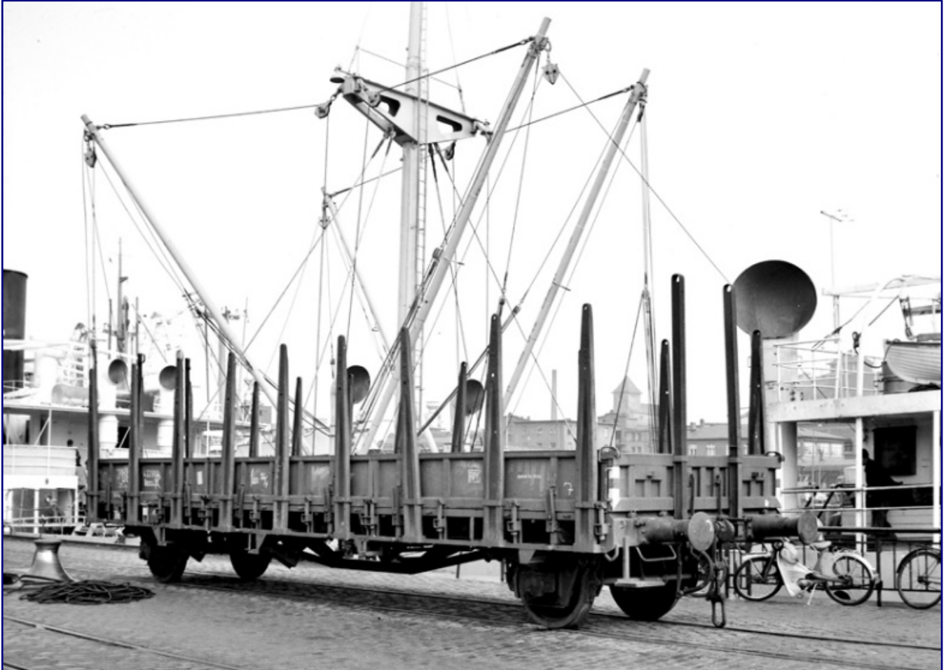
This stake car Rmms 33 with the road number 432 888 was photographed in Bremerhaven in September 1960. At that time, it was no longer common that it was still used with stanchions. Later, representatives of this type were still used as service freight wagons or railway service wagons into the nineties. Photo: Reinhard Todt, Eisenbahnstiftung
