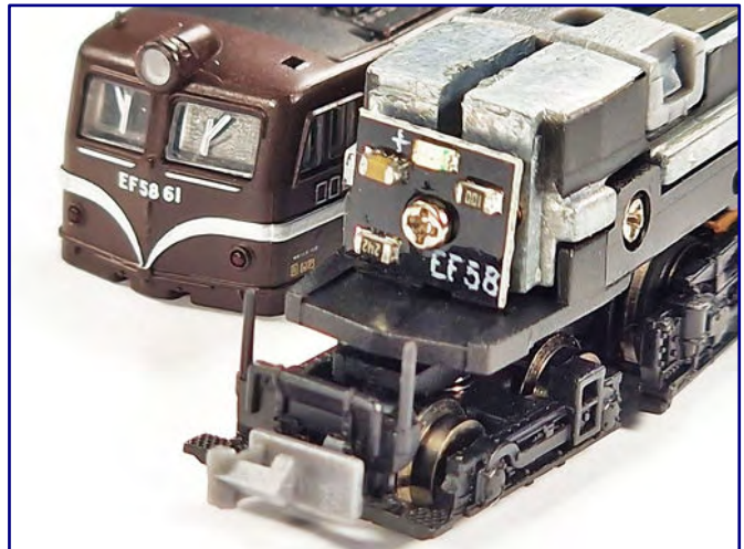
Photo above: The view inside reveals the small space under the housing. There is hardly any space left for the installation of a digital decoder.
