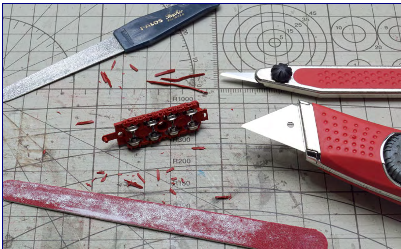
Photo above: The catches on the running gear for the weight used by Märklin have to give way, as well as the front buffers on the 3D printed housing are removed. The working surface of the heater must also be shortened a little with the file.
