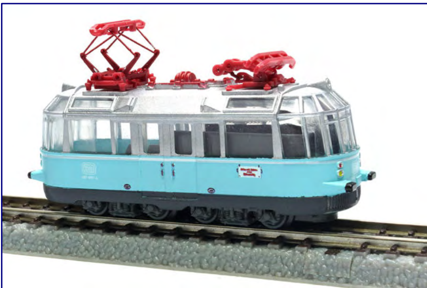
The Olympic blue version of the class 491 (art. no. ST015-1) shows us the finely and very prototypically designed scissor pantograph DBS54.
