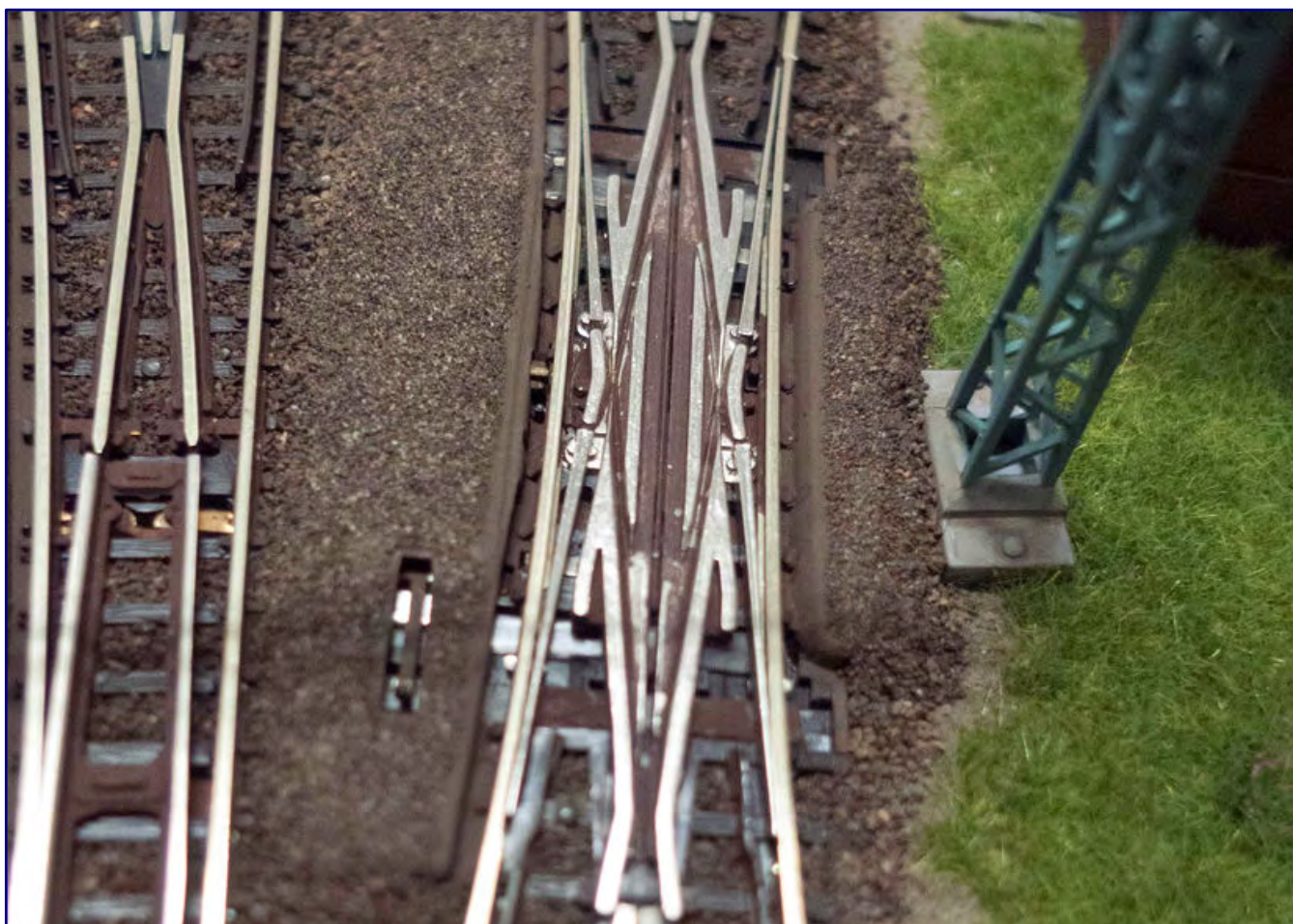
The double crossing turnout is only missing the prototypical turnout signal after editing, as described in the text (photo below).
