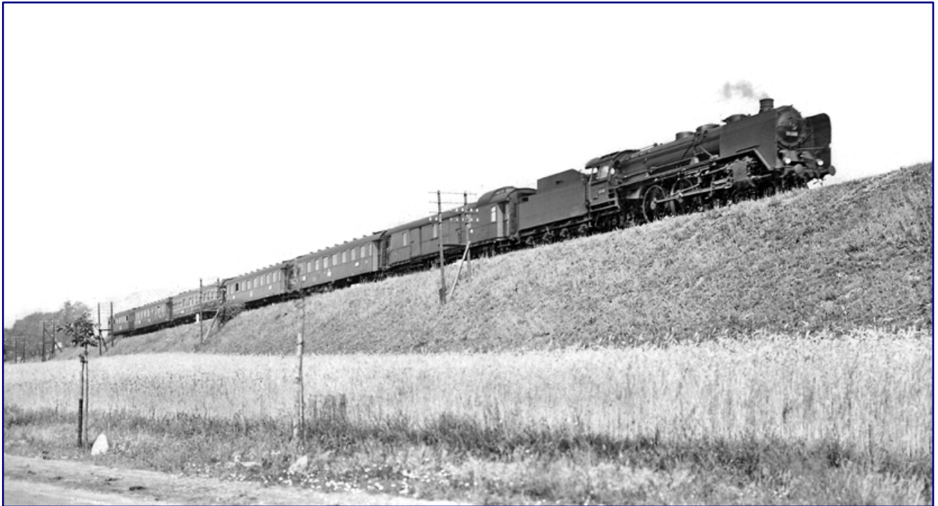
In front of the FD 23 (Hamburg - Berlin), the photographer had probably expected a class 05 locomotive, but instead it was 03 038 from the Bw Hamburg-Altona that led him on 2 August 1938. Taken between Zernitz and Neustadt (Dosse), its tender 2'2' T 32 of 1926 design, which we are making a model subject today, is also well featured. Photo: RVM-Filmstelle Berlin (Bellingrodt), Eisenbahnstiftung
