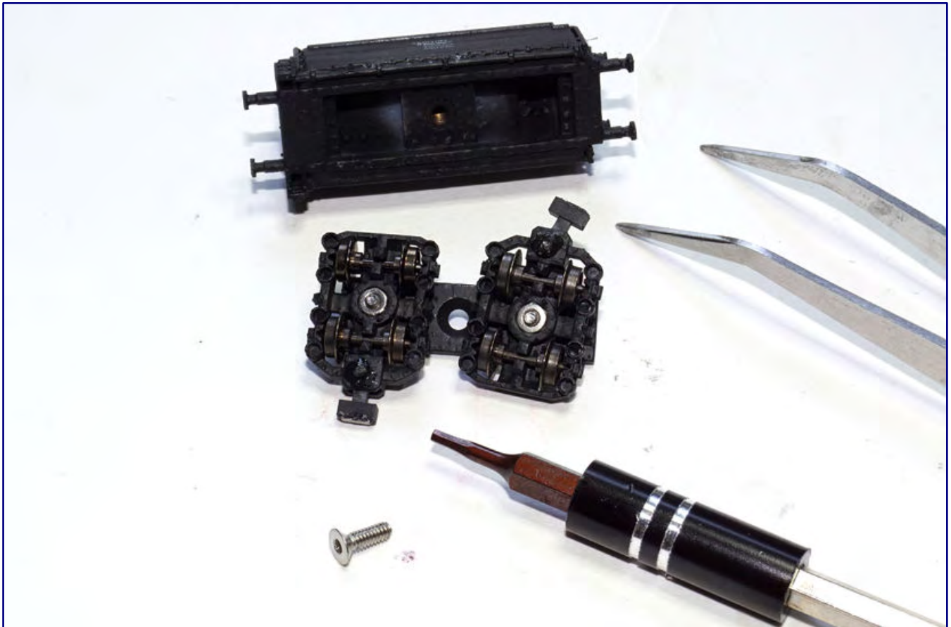
The screws of the bogies engage from above through the undercarriage into the glued-in nuts. The undercarriage floor, on the other hand, is screwed from below with a hexagon socket screw in the melted-in sleeve of the tender body
