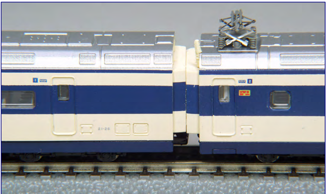
A close-up of all the different operating markings: Except for the printing on the sign next to the right-hand entrance door, they are all flawlessly executed. The delicate but movable pantographs are also a sight worth seeing.
