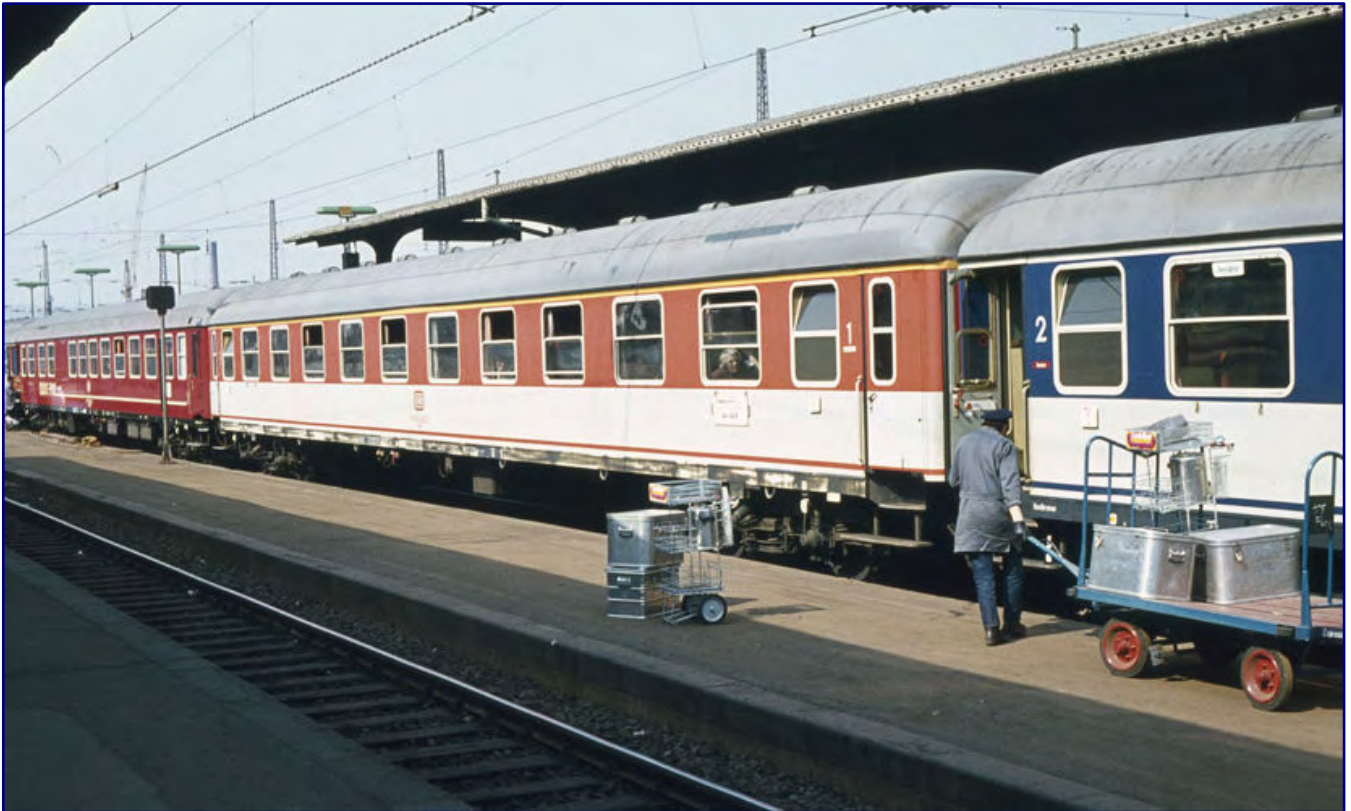
D 577 (Hamburg-Altona - Basel SBB) was one of the (predominantly) purely coloured trains, here at the head end in Kassel Hbf in 1974. It can be seen here that the DB's wish was not always realisable in operation. The blood orange Aüm 203 as coach 10 stands next to a purple WRbumz 138, to its right a Büm 234 joins it as coach 9. Photo: Volker Credé
