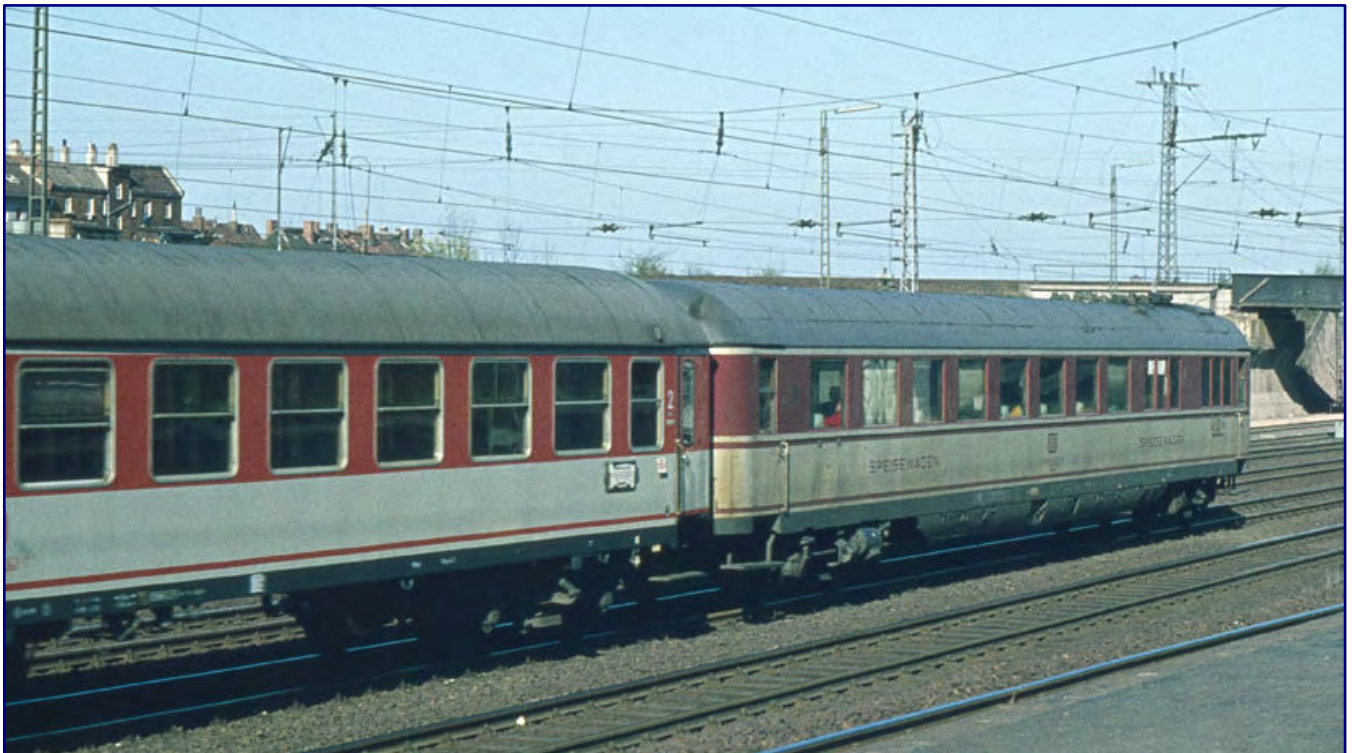
As many as five apron dining cars WRüge 152 took part in the colour test. Here, in 1974, next to one of only three couchette cars Bcüm 243 in RAL 4002 red-violet, the comparison shows the essential difference of an additional decorative stripe below the window band. Photo: Volker Credé
