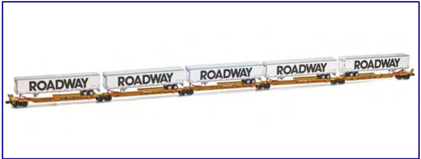
The TTAX Trinity RAF 53C Spine Cars (905205-1), which run on Jacob's bogies, are five-part and are being launched on the market as a new mould. Photo: AZL / Ztrack
