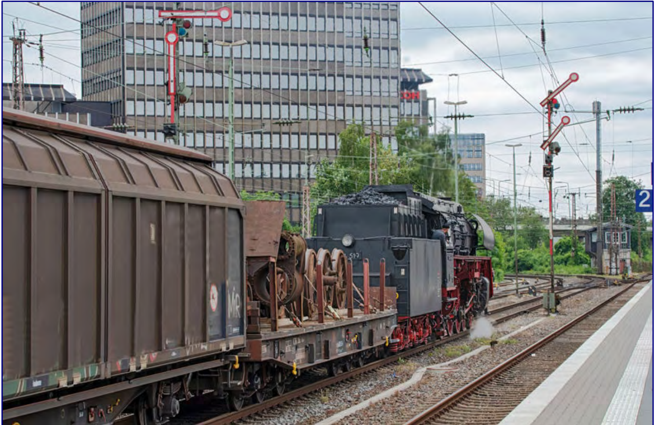
With 01 519 the circle closes: The original of the Märklin model survived as a heating locomotive in the form of a torso before it was completed and refurbished again. In the after shot on 24 June 2018, the tender view proves the coal box elevation missing from the model. Photo: Marcus Henschel, Sammlung Eisenbahnstiftung
