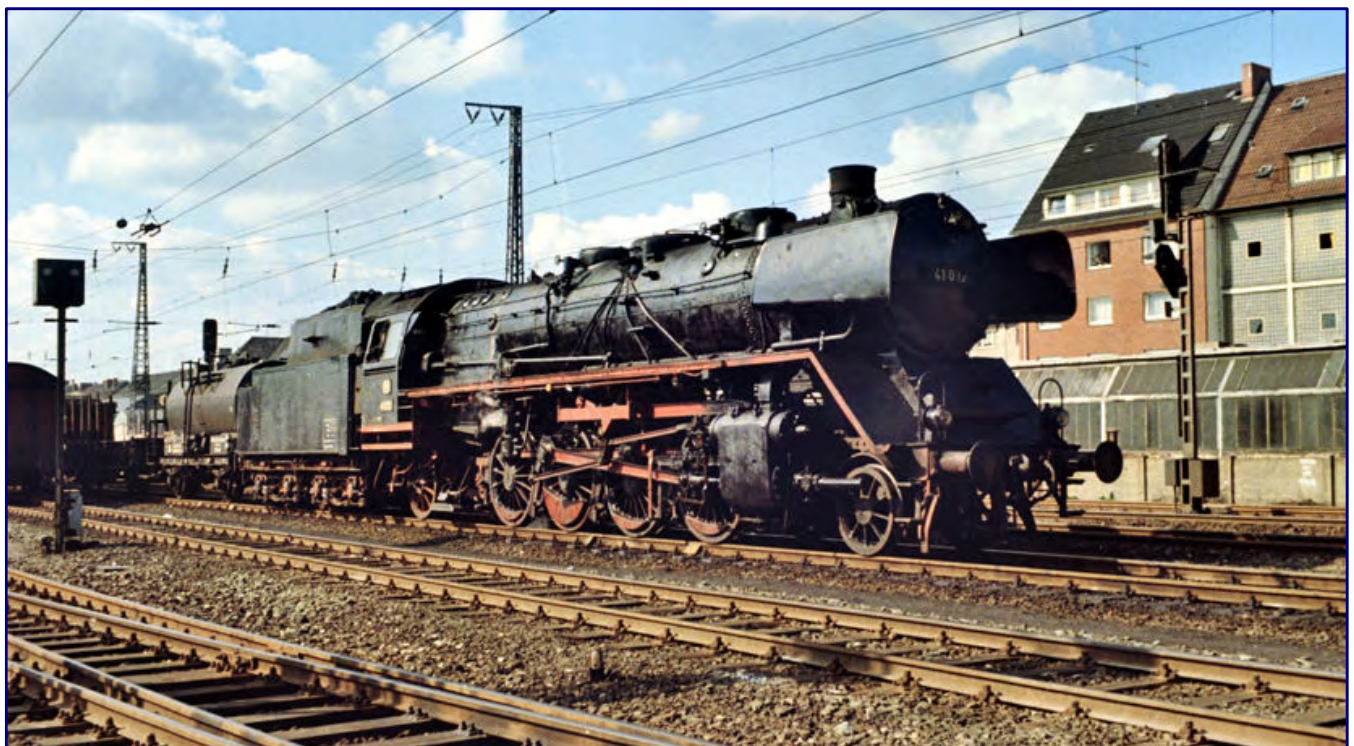
The photo of box tenders on DRG unit locomotives is far more colourful than manufacturer Märklin would have us believe: here 41 032 (with old construction boiler) from the Rheine depot was photographed in Münster (Westf.) Gbf on 11 April 1968. Coupled to it is a riveted 2'2' T 32, which it only received after 1945. Photo: Bernd Kappel, Eisenbahnstiftung
