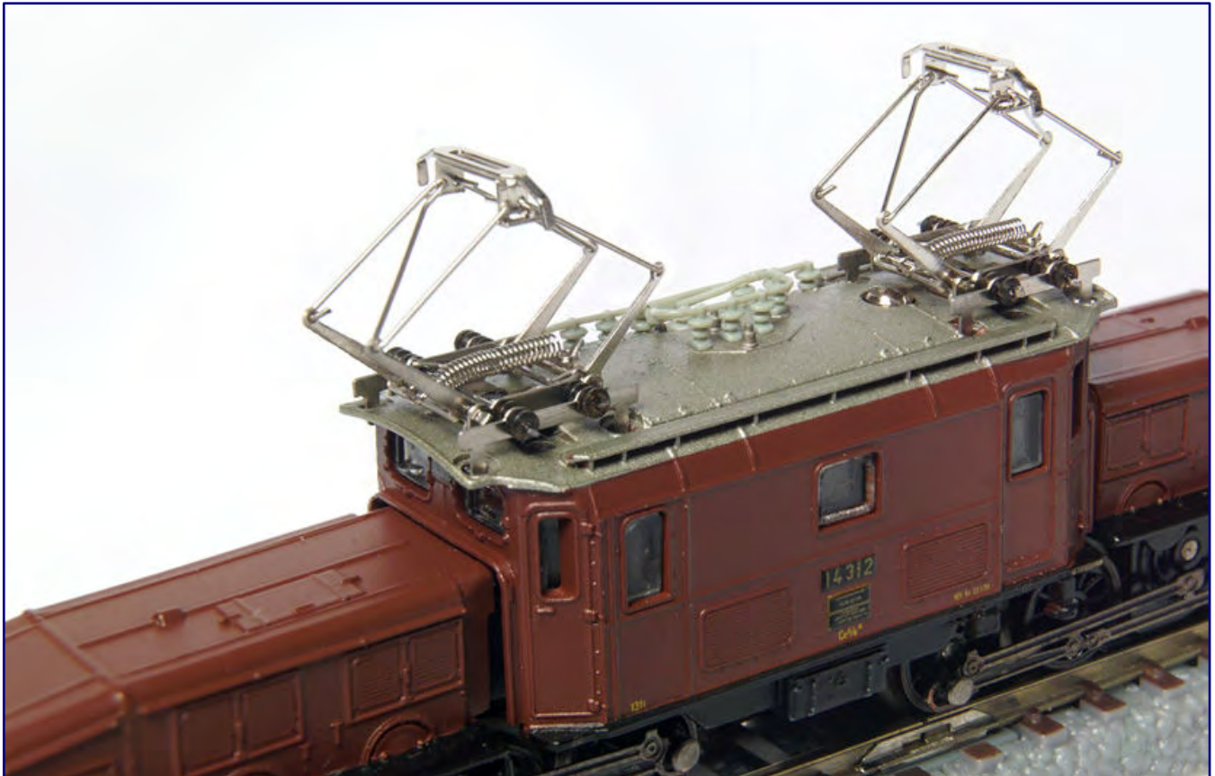
The version with insulator support replaces two other Märklin parts and also changes the shape and alignment of the insulators in a fine design.
