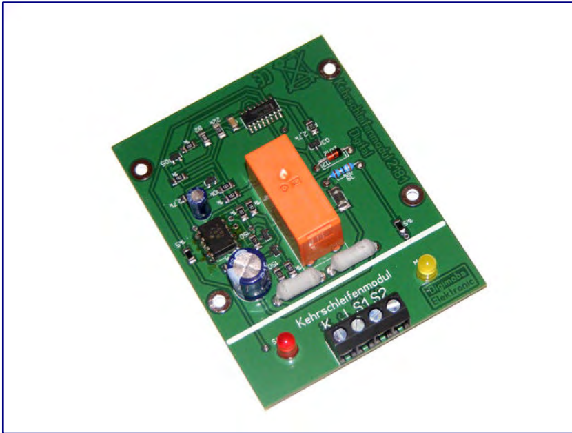
The digital reverse loop module (item no. 2181) is also interesting for use in Z gauge. Photo: Digimoba Elektronic
