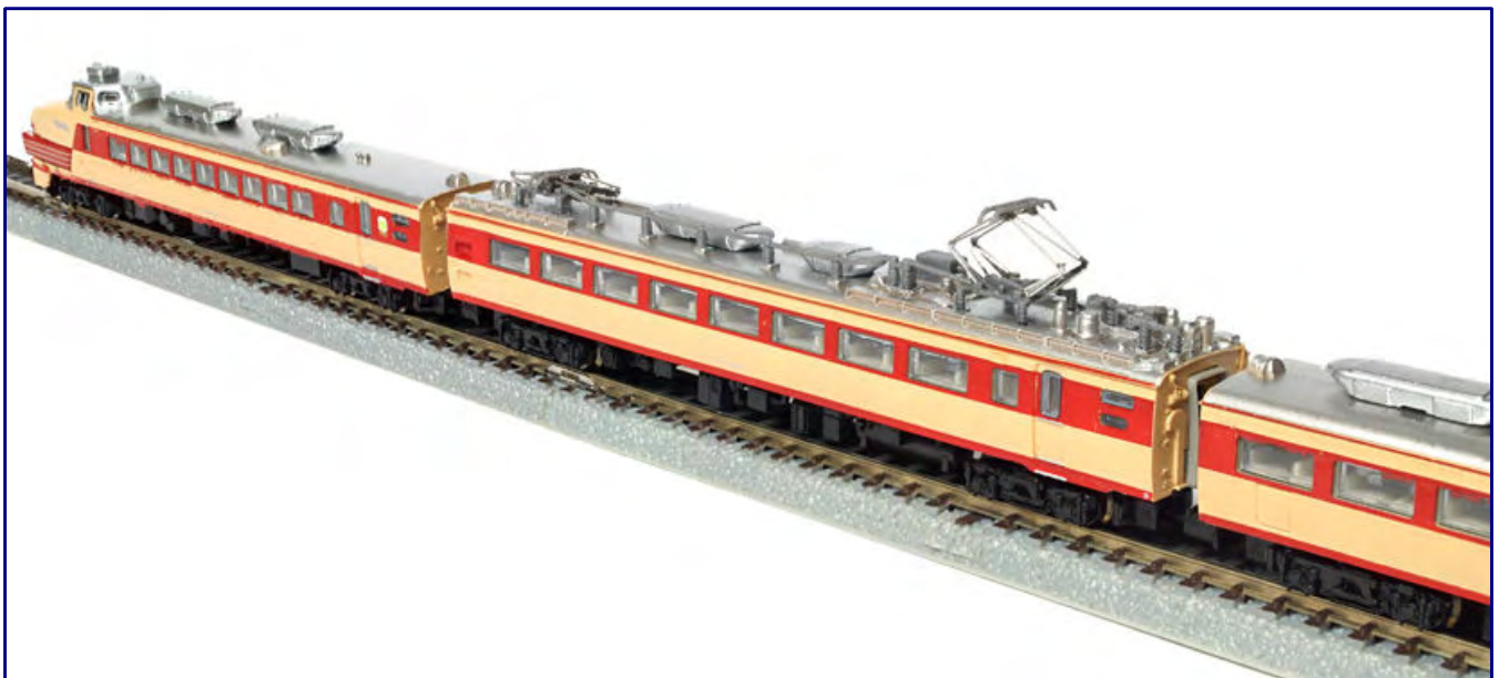
The scissor pantographs on the roofs of the JNR 485 series electric multiple unit from Rokuhan look successful: filigree, correctly sized, correctly mounted and fitted with diagonal braces. The front, lowered pantograph also lies flat.
